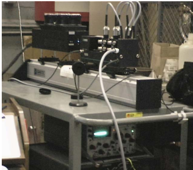
(a) LDV system used in this study
