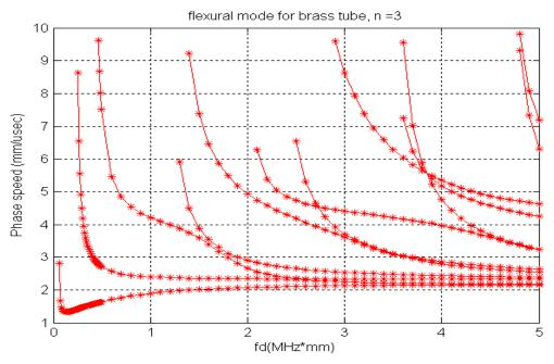
Figure 3.11a. The third circumferential order flexural modes in a brass tube, phase speed.
