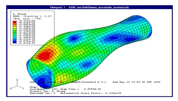
Figure 8.10. Lamb wave in a tube at time 6.9993e-4.
