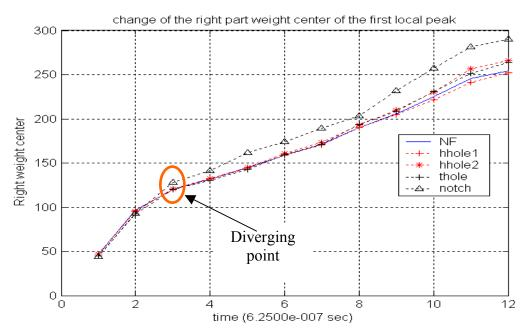
Figure 7.20. The change of right part weight center of the first local peak as the zooming window changing size from 100 to 1200, using anti-symmetric mode signals, propagating from the left to the right, input frequency 13 kHz.
