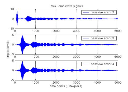
Figure 6.1. Lamb wave signals from an aluminum plate.
