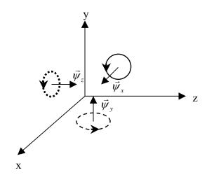
Figure 3.2. Vector potentials and particle movement.
