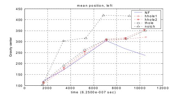
Figure 7.3. Change of left part weight center of local peaks from anti-symmetric mode signals propagating from the right to the left end, input frequency 14 kHz.
