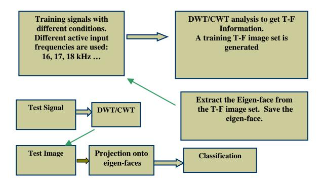
Figure 4.4. DWT/CWT + eigen-face analysis for structural flaw classification.
