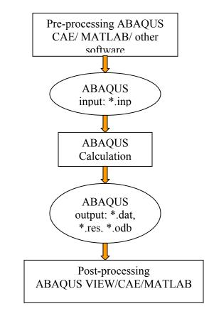
Figure 8.1. Flow chart for *ABAQUS* simulation process.
