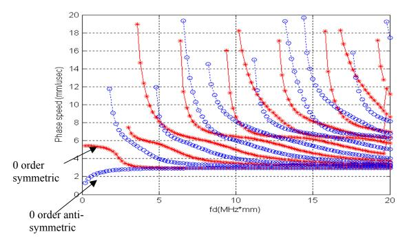
Figure 3.3. Dispersion curves for a traction free aluminum beam.
