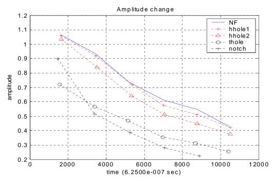
Figure A.5. Amplitude change in local peaks of anti-symmetric mode signals, propagating from left to right, input frequency 13 kHz.
