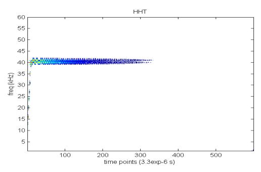
Figure 4.6b. HHT of the amplitude modulated signals illustrates frequency modulation introduced by amplitude modulation is small.
