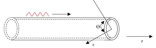
Figure 3.5. Guided acoustic waves in tubing.
