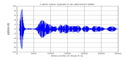
Figure 6.4. Lamb wave signal in an aluminum plate.
