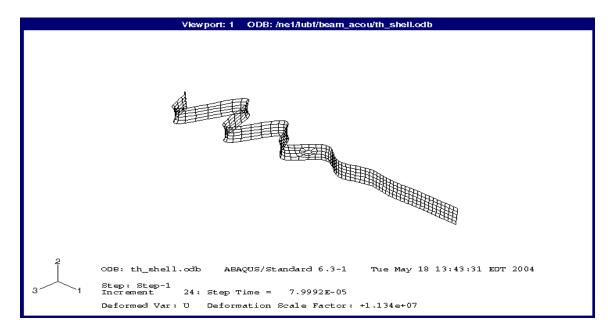
Figure 8.3. Lamb wave in a plate at time 7.9992e-5 second.
