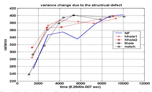
Figure 7.29. Spread change of local peaks from anti-symmetric mode signal before denoising, with input frequency 13 kHz.
