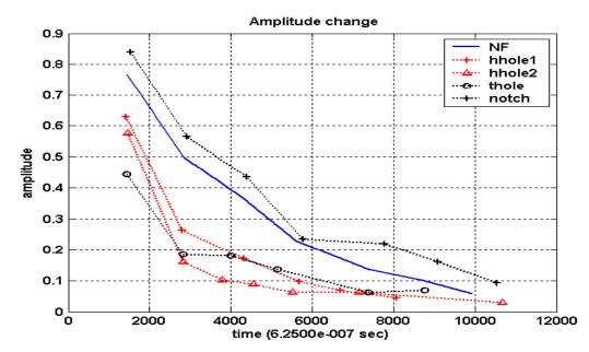
Figure 7.9. Amplitude change of local peaks of anti-symmetric mode signals in the water, propagating from left to right, with 13 kHz input frequency.
