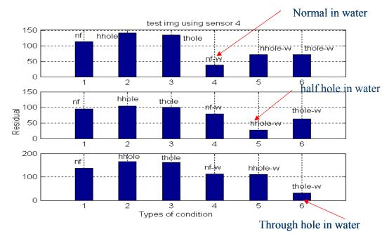
Figure 7.35. The tube defect classification using DWT + Eigen-face.
