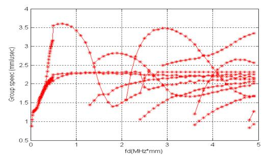
Figure 3.10b. The second circumferential order flexural modes in a brass tube, group speed.
