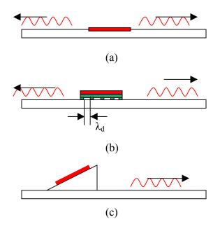
Figure 2.6. Methods of Lamb wave generation.
