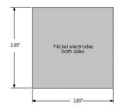
Figure 2.4. Piezoelectric sensor sheet. Thickness: 0.00105 inch (from PSI).
