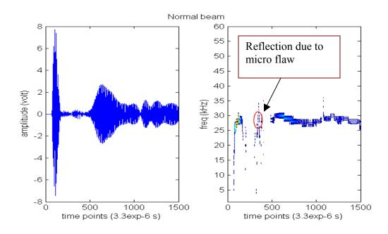
Figure 6.7. Normal Lamb wave signal and its HHT.
