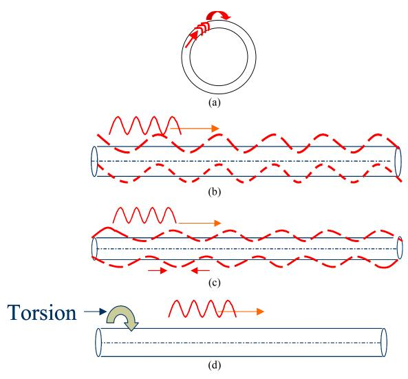
Figure 3.6. Lamb wave modes in tubular structures.
