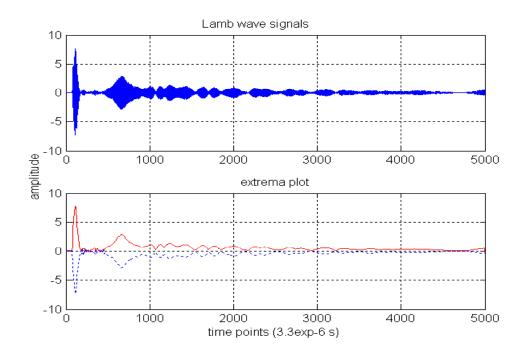
Figure 6.13. Lamb waves and envelope extraction.
