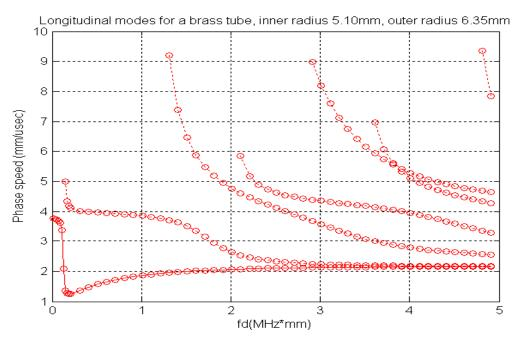
Figure 3.7a. Longitudinal modes in tubular structures, phase speed.
