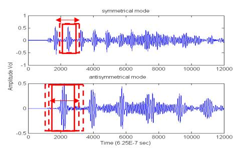
Figure 4.2. Signal localized properties using zooming windows.
