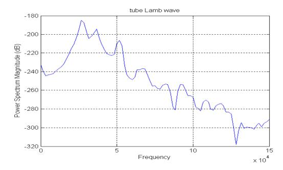
Figure 8.12. Frequency response for brass tube (from Simulation).
