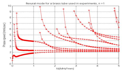
Figure 3.9a. Flexural modes in a brass tube with first circumferential order, phase speed.
