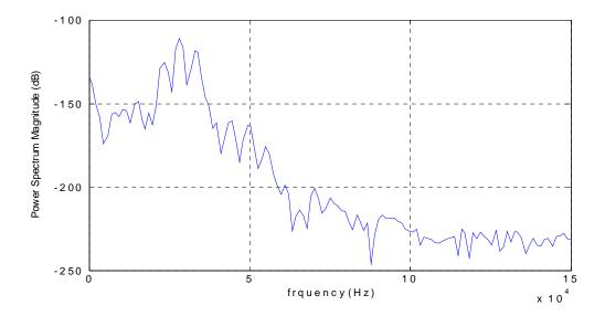
Figure 8.6. Frequency response for the plate (from Simulation).
