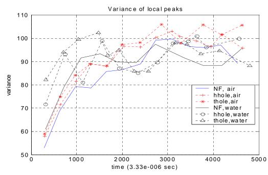
Figure 7.14. Change of variance of local peaks from anti-symmetric mode signals, propagating from the left to the right, with input frequency 16 kHz.
