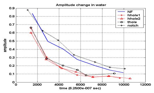
Figure 7.25. Amplitude change of local peaks from anti-symmetric mode signal after denoising, with input frequency 13 kHz.
