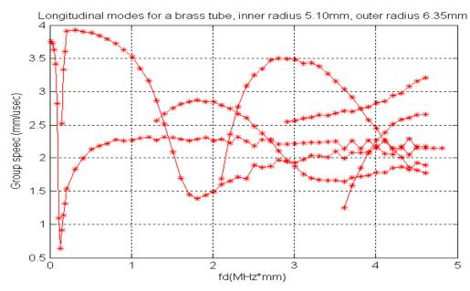
Figure 3.7b. Longitudinal modes in tubular structures, group speed.
