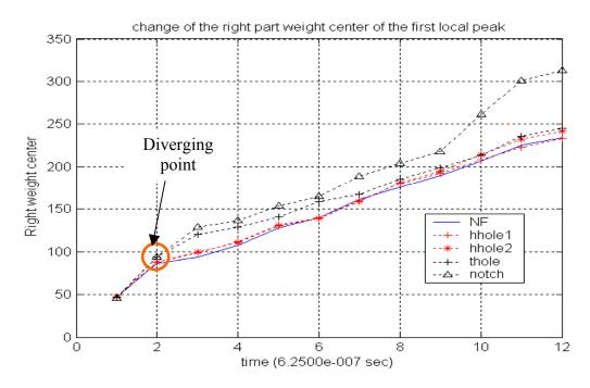
Figure 7.18. The change of right part weight center of the first local peak as the zooming window changing size from 100 to 1200, using anti-symmetric mode signals, propagating from the right to the left, input frequency 13 kHz.
