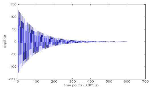
Figure 4.6a. amplitude modulated signals, 1000\*exp(-2\*t).\*cos(80\*pi\*t+1).
