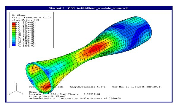
Figure 8.9. Lamb wave in a tube at time 6.3327e-4.
