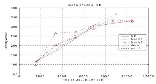
Figure A.3. The change in left part weight center of local peaks of anti-symmetric mode signals, propagating from left to right, input frequency 14 kHz.
