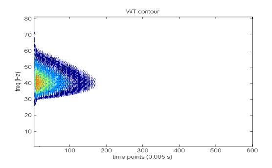
Figure 4.6c. WT of amplitude-modulated signals.
