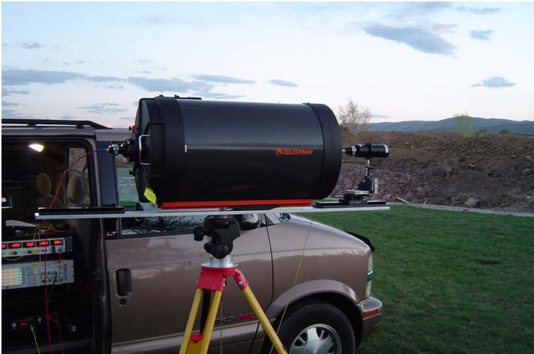
**Figure 19. Photograph Showing Outdoor Test Setup of Co-Aligned Transceiver with 14-Inch Telescope and 2-Inch Laser Source Optic**
