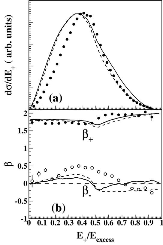
FIG. 3: (a)  $SDCS = d\sigma/dE_+$ , energy in units of the 100 eV excess energy. (b)  $\beta$ -parameter of the  $k_+$  and  $k_-$  momenta. The dots are the experimental data, the solid and dashed lines show 3C calculations in length and velocity form, respectively.
