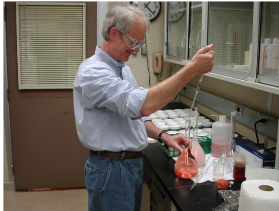
Photo 2 – Pipetting MWF to Flask
