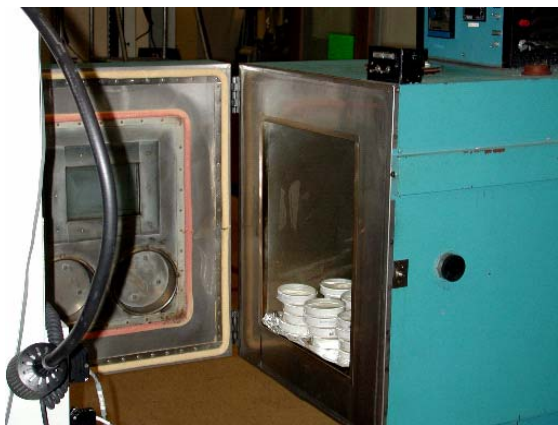
Photo 7 – Plates in Oven for Bake Out
