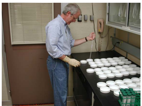
Photo 4 – Delivering Aliquot to Test Plate
