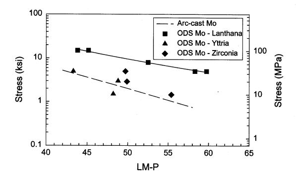
Figure 2. Larson-Miller plot of the stress rupture behavior of various 2 vol.% oxide ODS molybdenum compositions.
