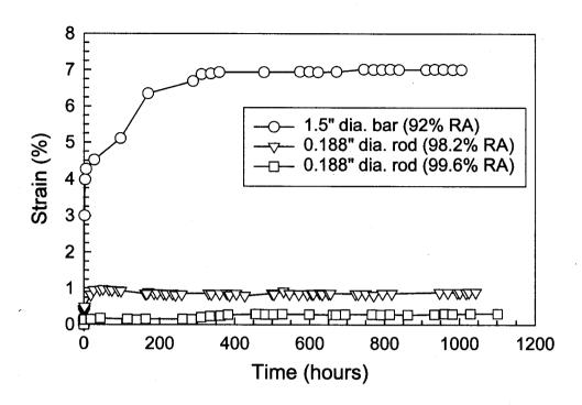
Figure 4. Effect of total cold work on creep resistance of ODS molybdenum; constant load uniaxial creep at 1600°C (2912°F) and 5ksi (34.5MPa).
