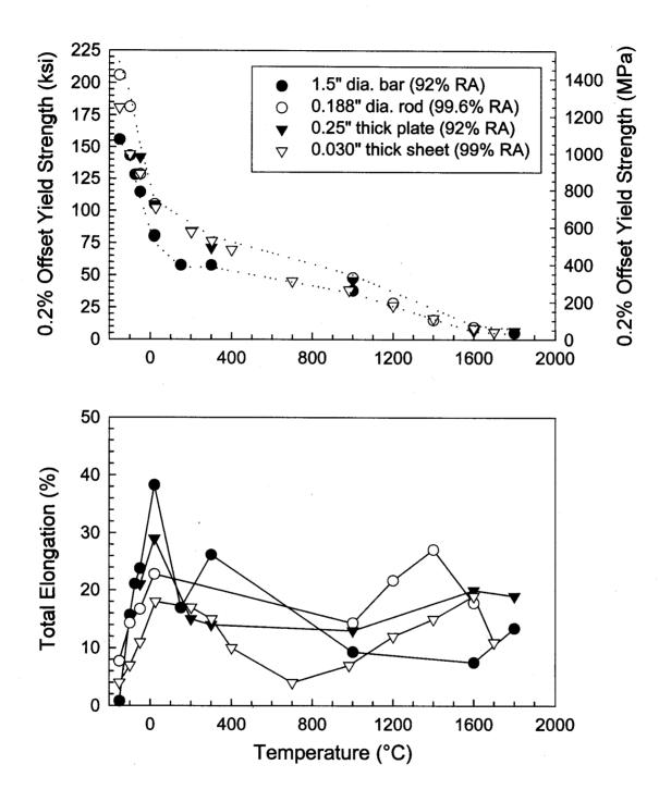
Figure 3. Tensile properties of ODS molybdenum as a function of temperature.
