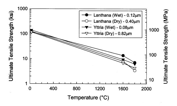
Figure 1. The effect of oxide species and processing method on the strength of 2 vol.% ODS molybdenum material as a function of temperature.
