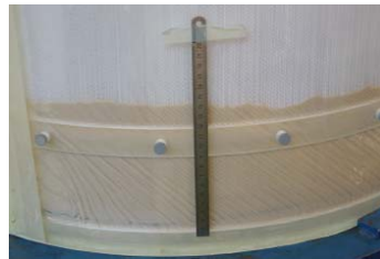
Injection of resin into the stack
