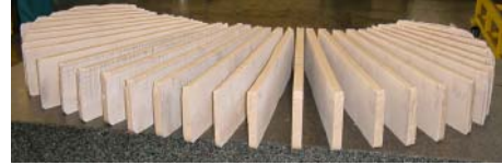
Pure resin – cut in slices for inspection
