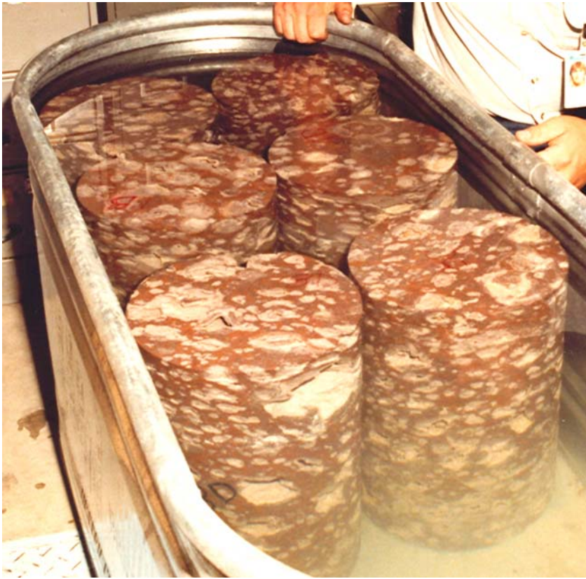
Figure 6.3-9. Large (267 mm or 10.5-in) Diameter Busted Butte Samples from the Tptpul Unit
