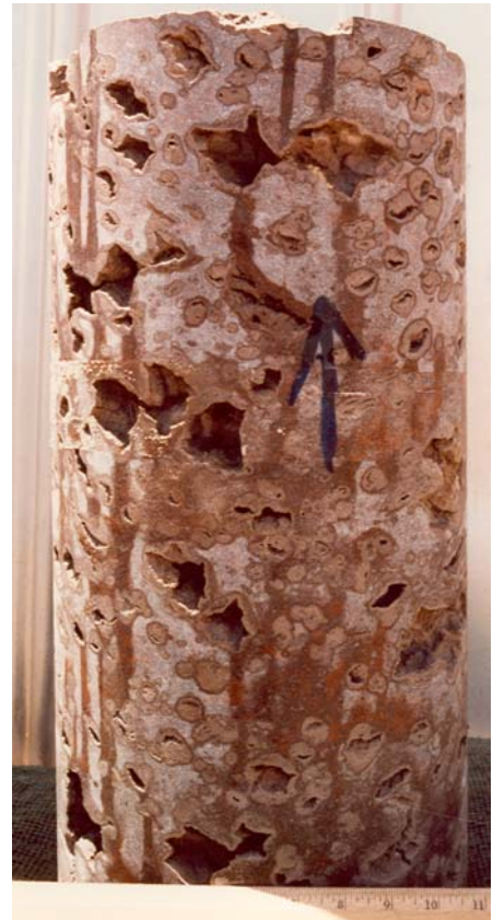
Figure 6.3-9. Large (267 mm or 10.5-in) Diameter Busted Butte Samples from the Tptpul Unit
