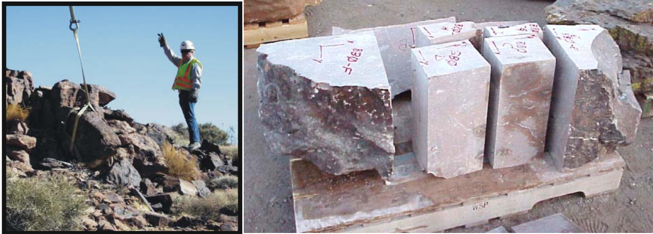
Figure 6.3-19. Rock block being removed from Busted Butte (left) and Development of Rectangular Specimens for Matrix Size Effect Study (right)
