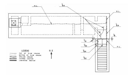
Fig. 3.73-Roof-slab crack pattern (structure CAb).
