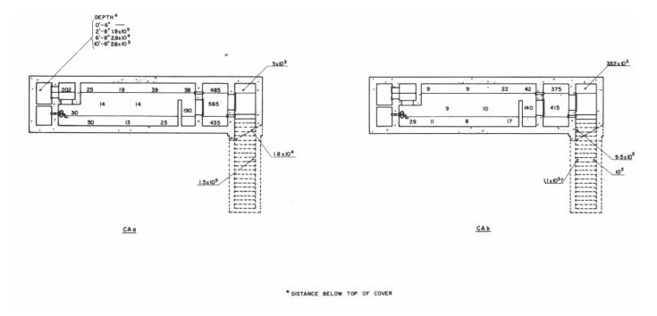
Fig. 3.120—Approximate total gamma dosages during first 52 hr after detonation (structure CA).
