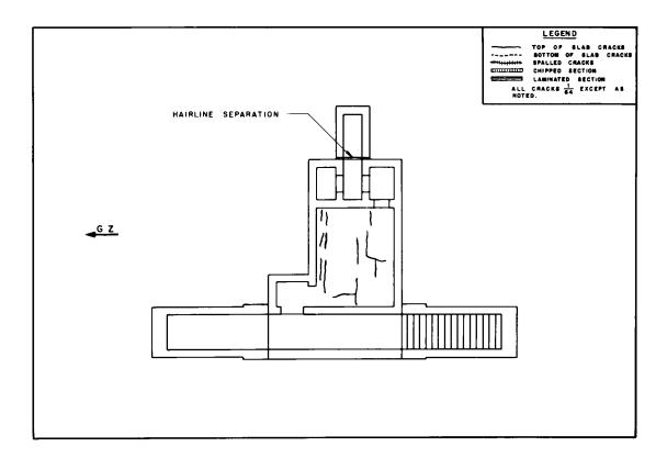
Fig. 3.100-Floor-slab crack pattern (structure RCc).
