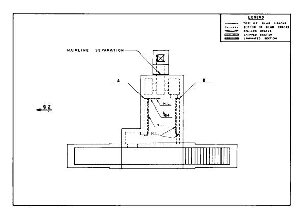
Fig. 3.99-Roof-slab crack pattern (structure RCc).
