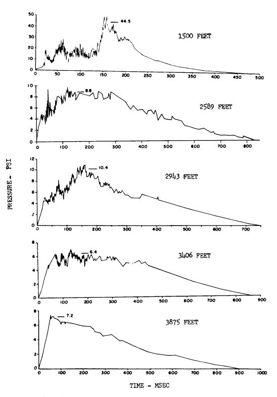
Fig. 3.109-Blast-line pressure-time; self-recording pressure gauge records.
