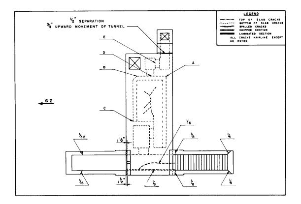
Fig. 3.33-Roof-slab crack pattern (structure RAc).
