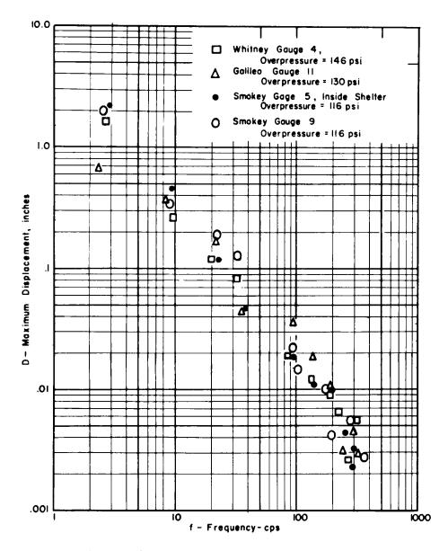
Fig. 3.124-Displacement-shock spectrum, horizontal direction.
