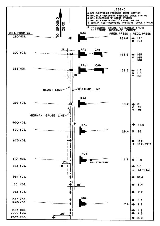
Fig. 1.4—Location and orientation of structures, project 30.7.
