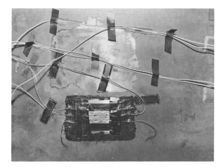
Fig. 3.70 — Detail of strain gauges on main blast door (structure CAa).
