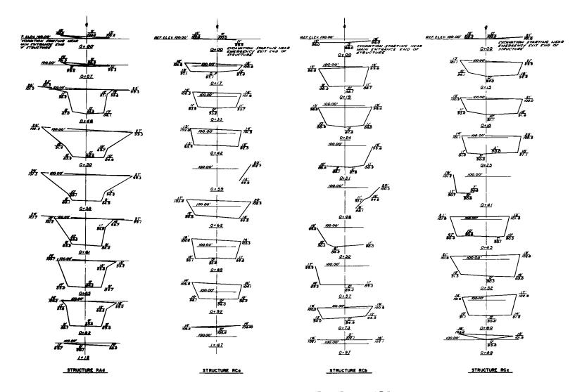
Fig. A.23-Excavation of structures RAd, RCa, RCb, and RCc.
