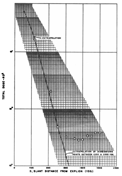
Fig. 3.122-Blast-line total gamma dose-distance curve.
