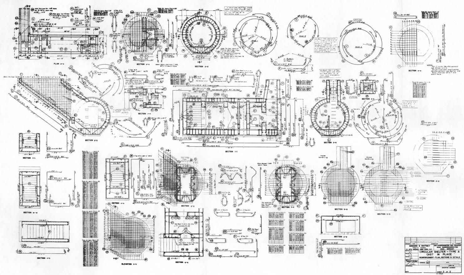
Fig. B.2.2-Reinforcement plan (sections and details) for type A cast-in-place circular shelter.
