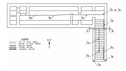
Fig. 3.59-Floor-slab crack pattern (structure CAa).
