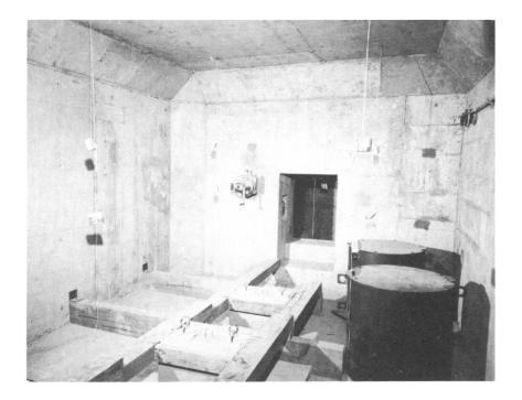
Fig. 2.16-Shock-gauge canisters and Ensolite test equipment.
