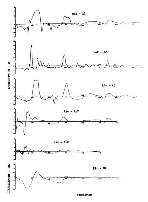
Fig. 5.125—Acceleration- and displacement-time, acceleration test gauge records.
