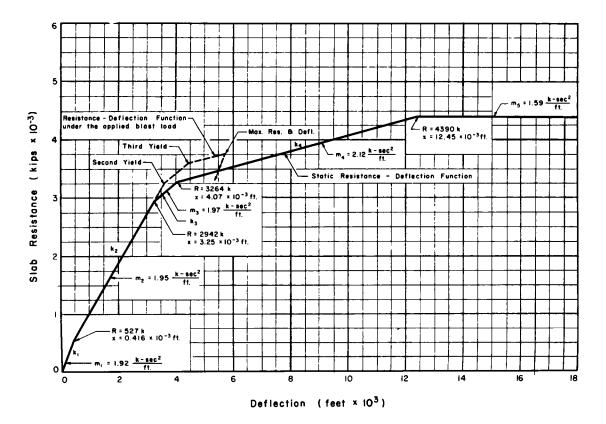
Fig. C.2—Resistance-deflection curve.
