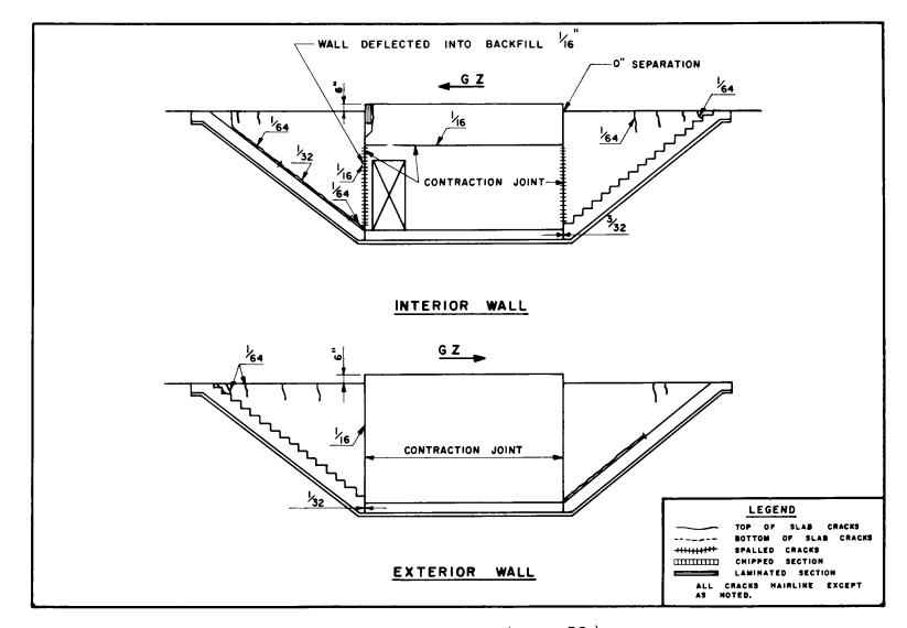
Fig. 3.84—Entrance crack pattern (structure RCa).
