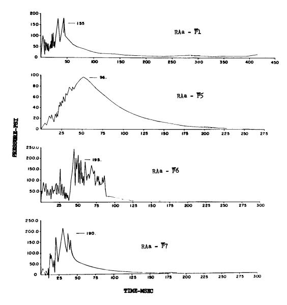
Fig. 3.104-Pressure-time; BRL self-recording pressure gauge records.
