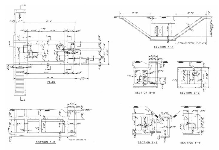
Fig. 1.1—Architectural layout for type A rectangular shelter.
