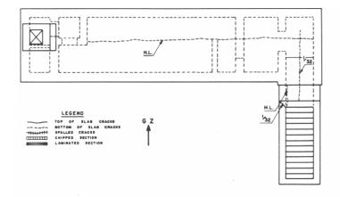
Fig. 3.58-Roof-slab crack pattern (structure CAa).
