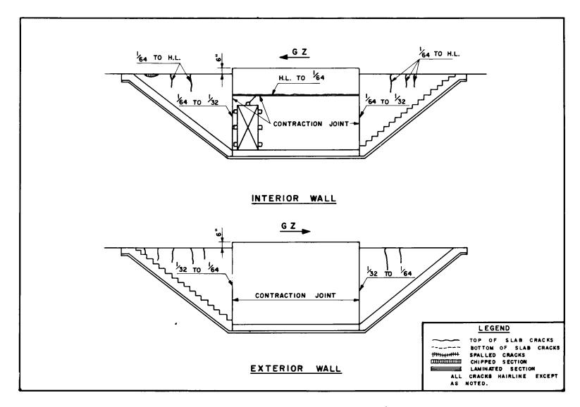
Fig. 3.94-Entrance crack pattern (structure RCb).
