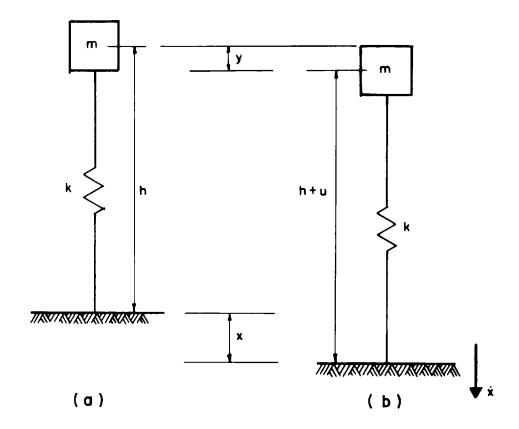
Fig. 2.14 - Single-degree-of-freedom spring-mass system.
