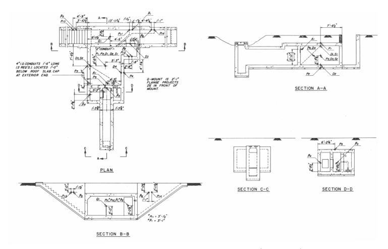
Fig. 2.10-Instrumentation layout for type C rectangular shelter (structure RCa).
