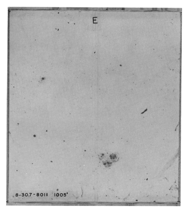
Fig. 3.128-Sticky-paper dust collector, type B (structure RAc).
