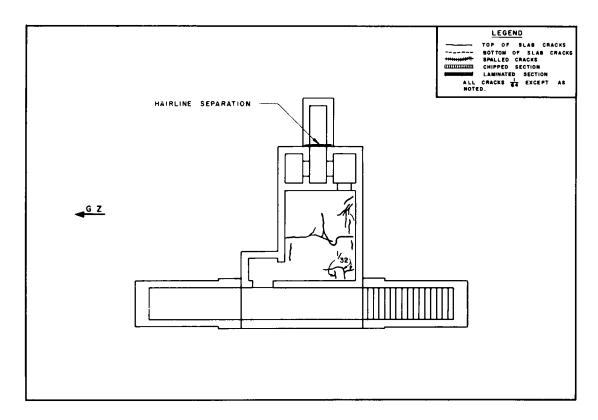
Fig. 3.93-Floor-slab crack pattern (structure RCb).
