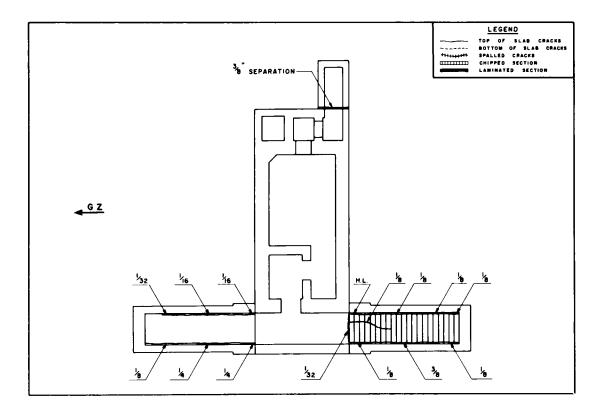
Fig. 3.55-Floor-slab crack pattern (structure RAd).
