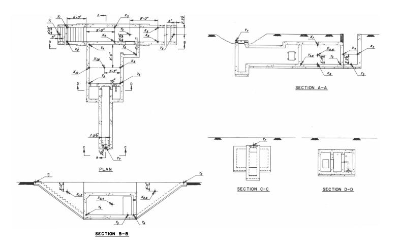
Fig. 2.3—Type C rectangular shelter, survey points.
