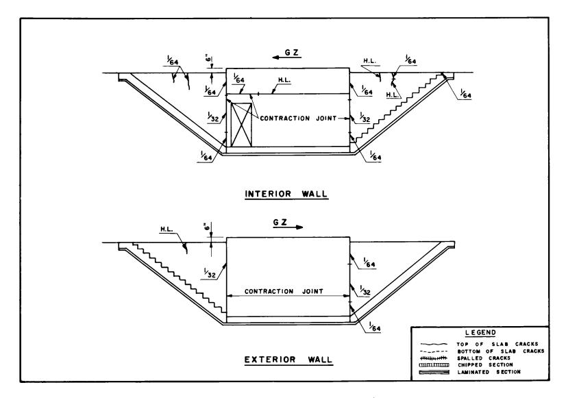
Fig. 3.101—Entrance crack pattern (structure RCc).
