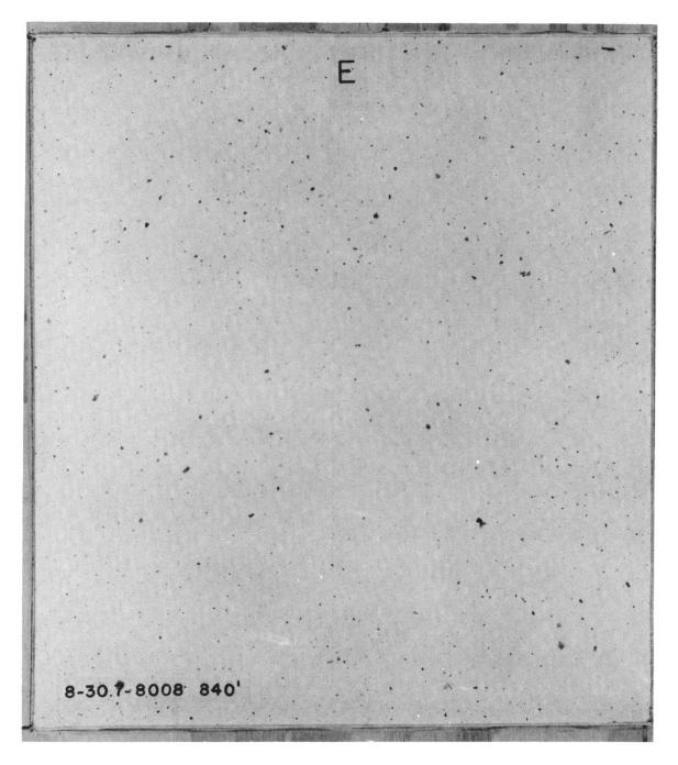
Fig. 3.126-Sticky-paper dust collector, type B (structure RAa).
