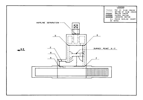
Fig. 3.92-Roof-slab crack pattern (structure RCb).
