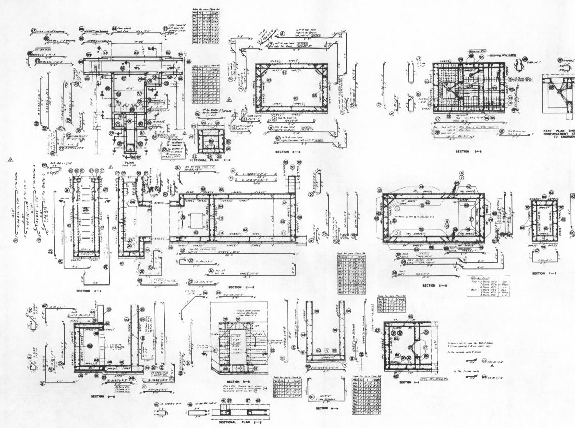
Fig. B.3.2-Reinforcement plan (sections and details) for type C cast-in-place rectangular shelter.
