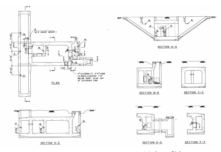
Fig. 2.6 — Instrumentation layout for type A rectangular shelter (structure RAc).
