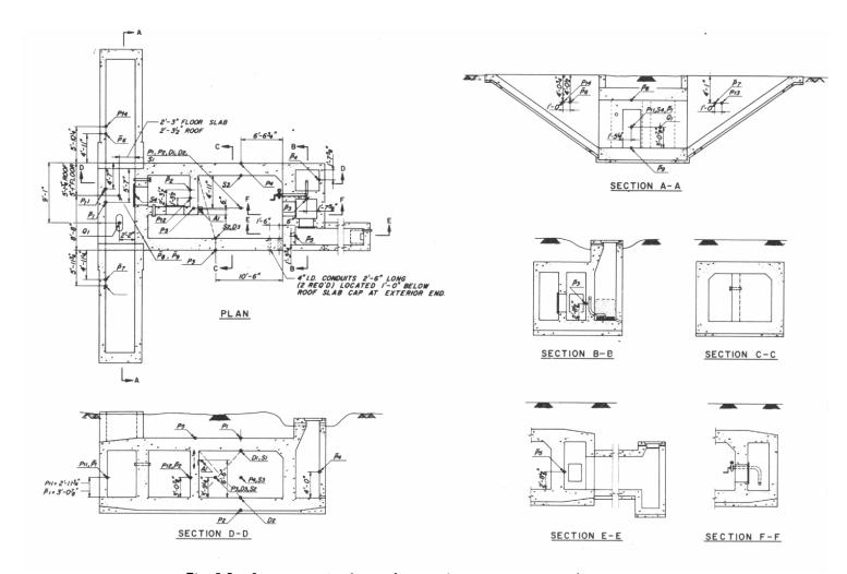
Fig. 2.5- Instrumentation layout for type A rectangular shelter (structure RAb).
