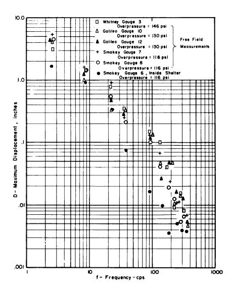
Fig. 3.123-Displacement-shock spectrum, vertical direction.
