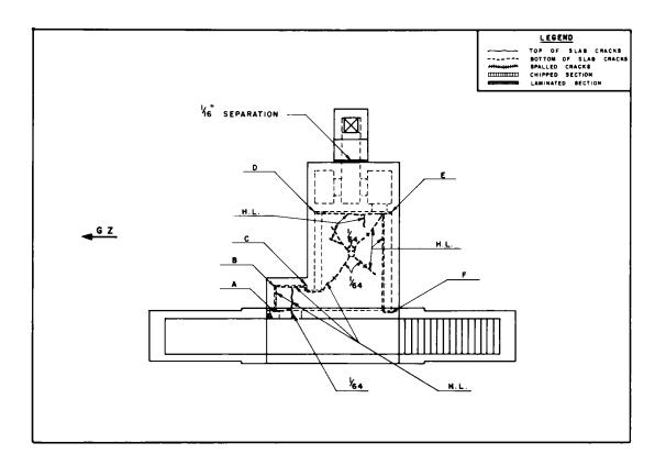
Fig. 3.82-Roof-slab crack pattern (structure RCa).
