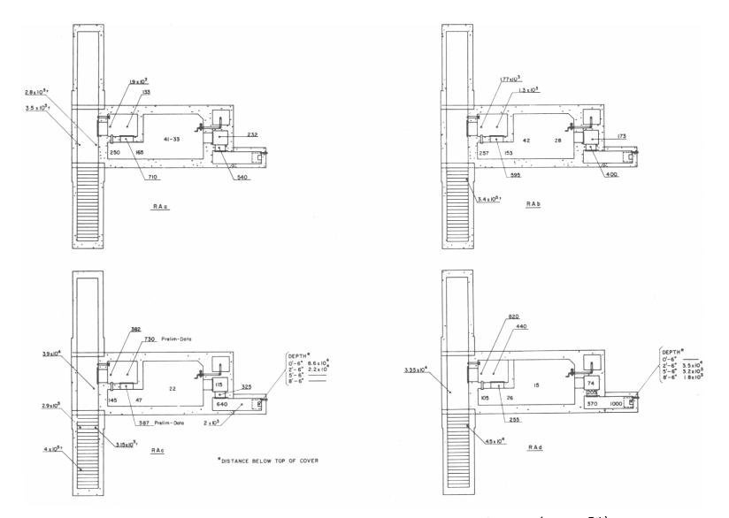
Fig. 3.119-Approximate total gamma dosages during first 52 hr after detonation (structure RA).
