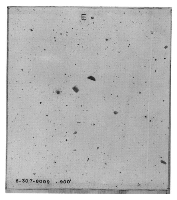
Fig. 3.134-Sticky-paper dust collector, type B (structure CAa).
