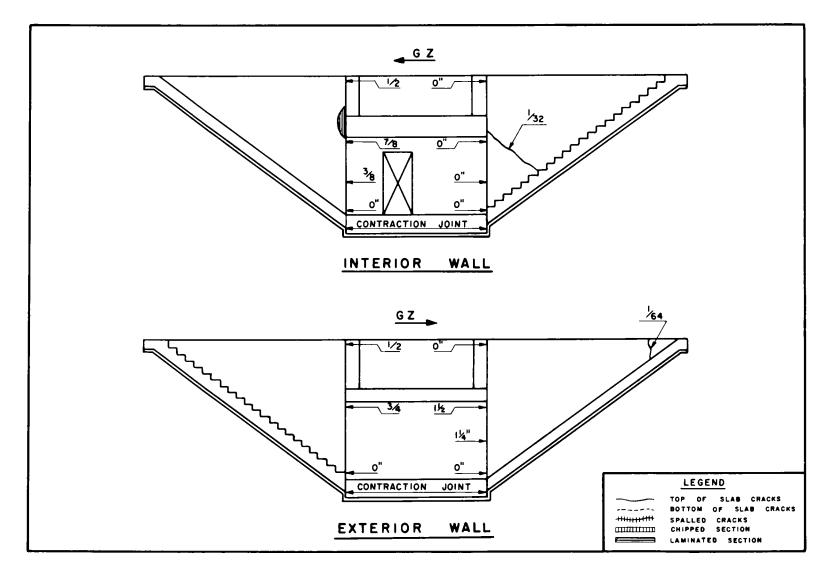
Fig. 3.56—Entrance crack pattern (structure RAd).
