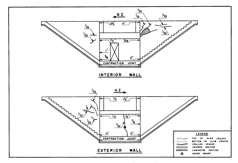
Fig. 3.35—Entrance crack pattern (structure RAc).
