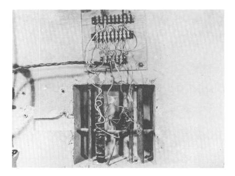
Fig. 3.31-Close-up of strain gauge in side wall of main chamber (structure RAb).
