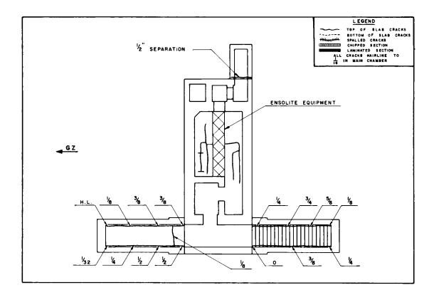
Fig. 3.34—Floor-slab crack pattern (structure RAc).
