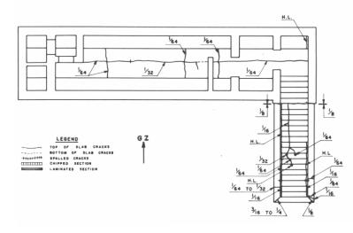
Fig. 3.74—Floor-slab crack pattern (structure CAb).
