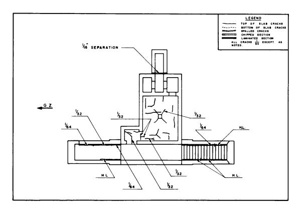
Fig. 3.83-Floor-slab crack pattern (structure RCa).
