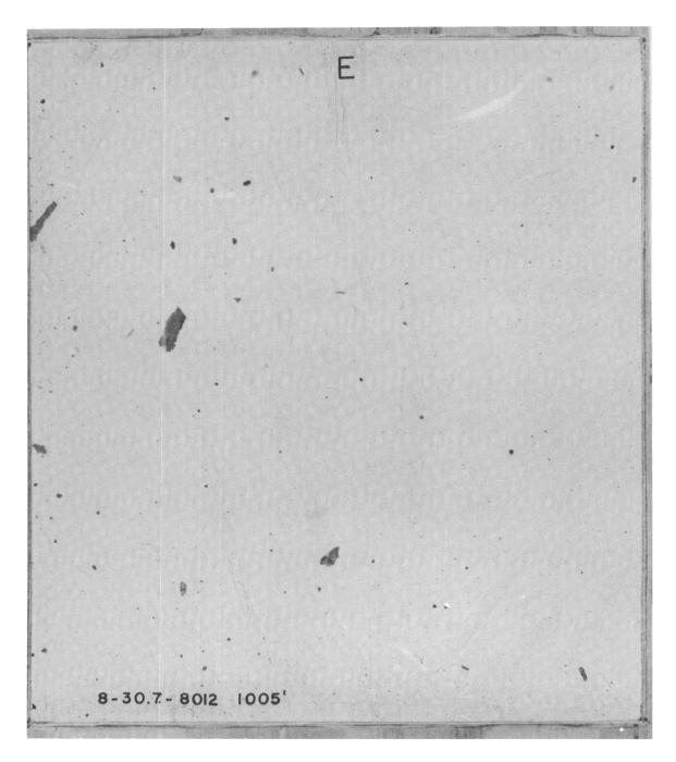
Fig. 3.135—Sticky-paper dust collector, type B (structure CAb).
