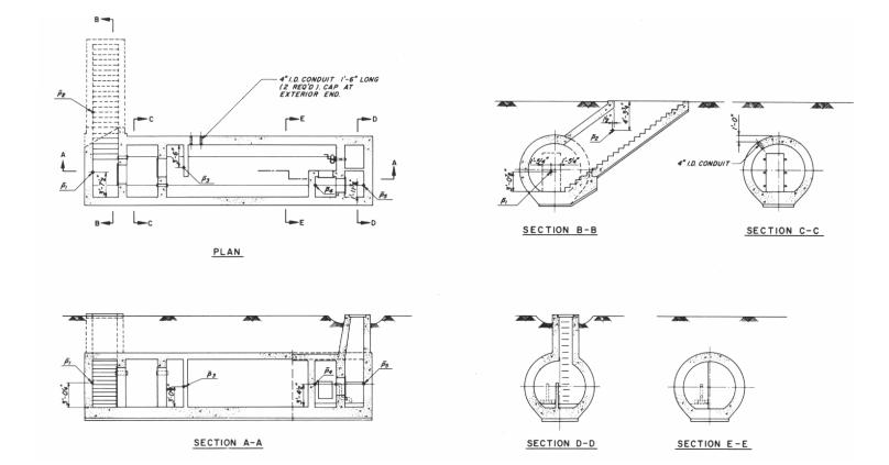
Fig. 2.9—Instrumentation layout for type A circular shelter (structure CAb).
