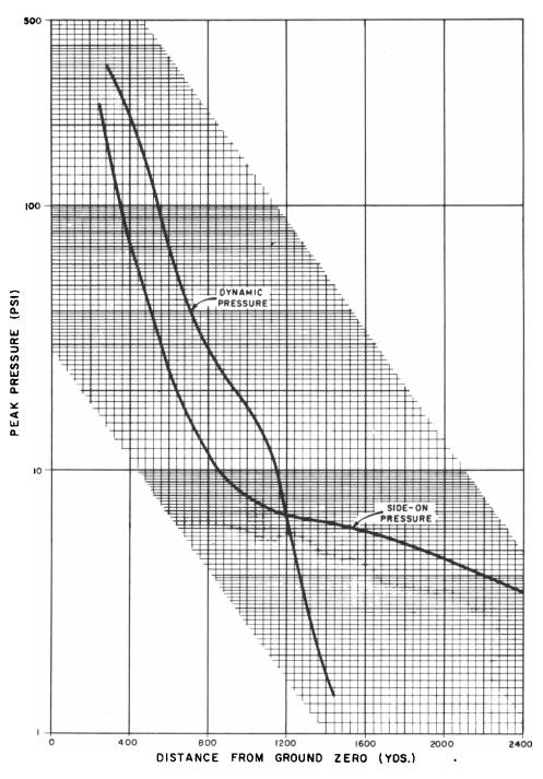
Fig. 3.106-Blast-line pressure-distance curve.
