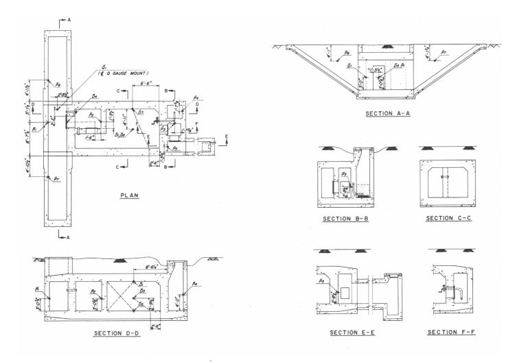
Fig. 2.4 — Instrumentation layout for type A rectangular shelter (structure RAa).
