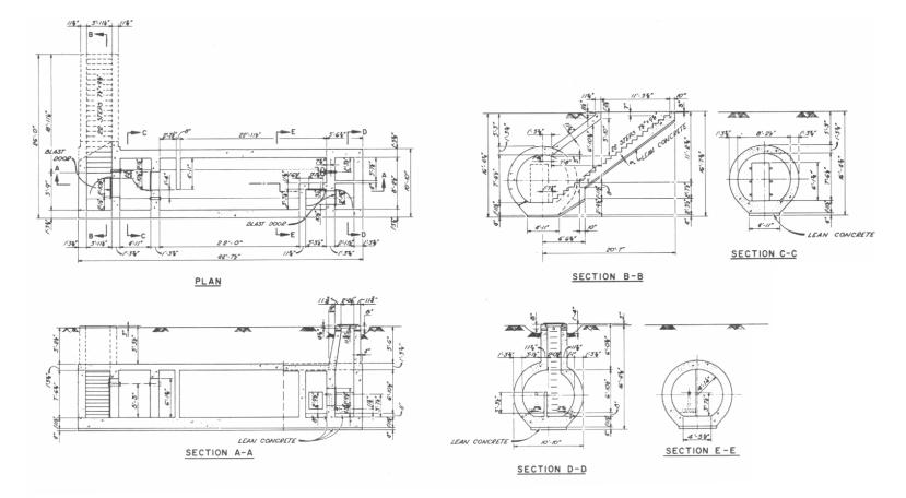
Fig. 1.2-Architectural layout for type A circular shelter.
