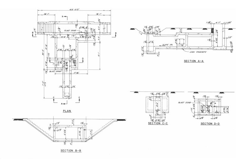
Fig. 1.3—Architectural layout for type C rectangular shelter.
