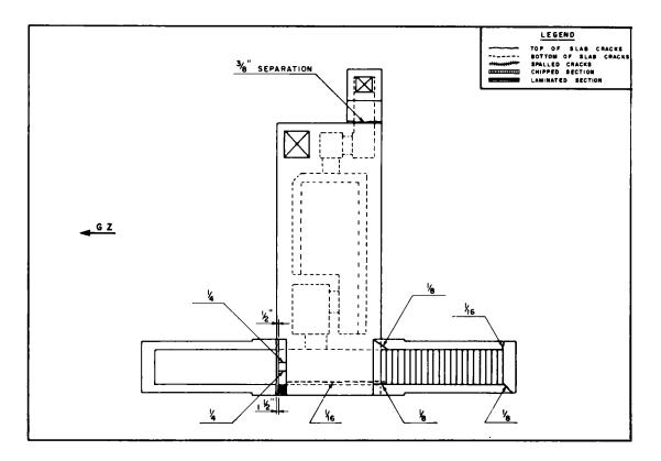
Fig. 3.54-Roof-slab crack pattern (structure RAd).
