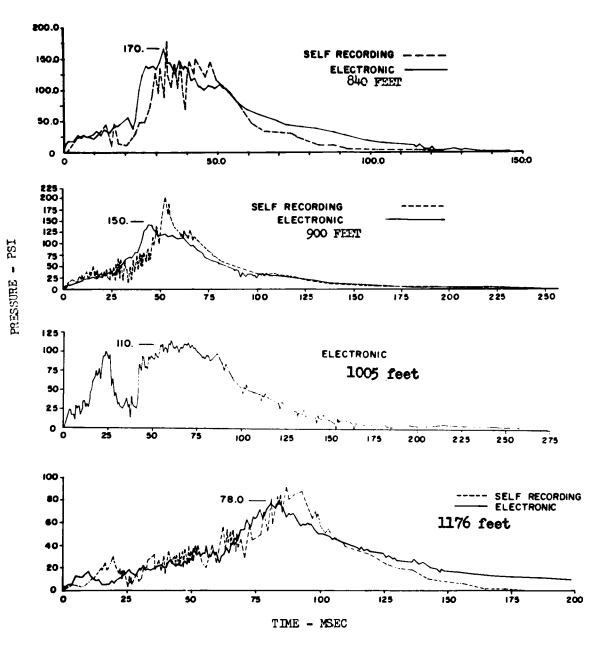
Fig. 3.108-Blast-line pressure-time; electronic and self-recording gauge records.
