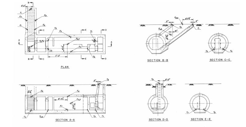
Fig. 2.2-Type A circular shelter, survey points.
