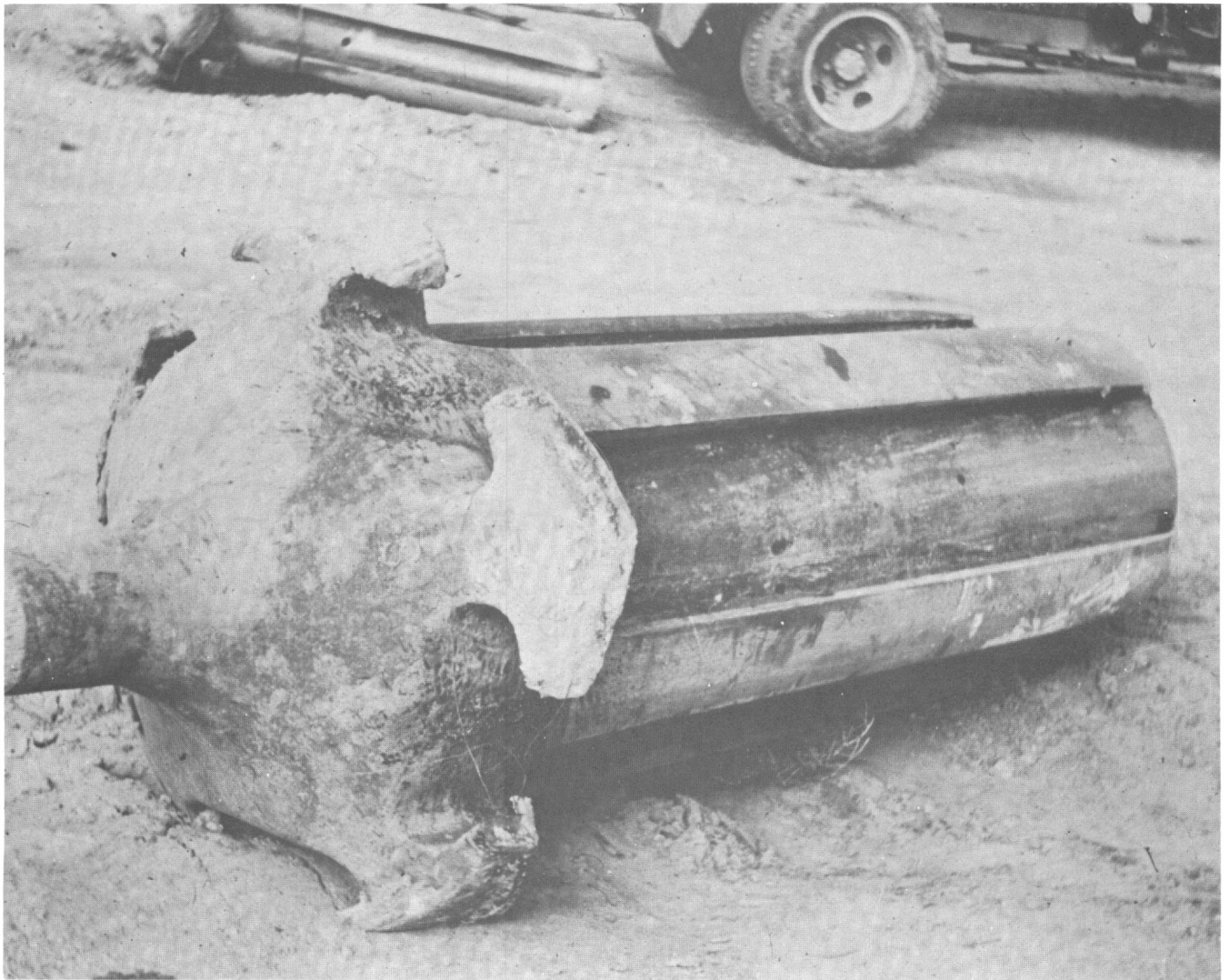
Fig. 2. View of a 32" to 42" churn drill hole opener bit. Photo-Layne Texas Co.
