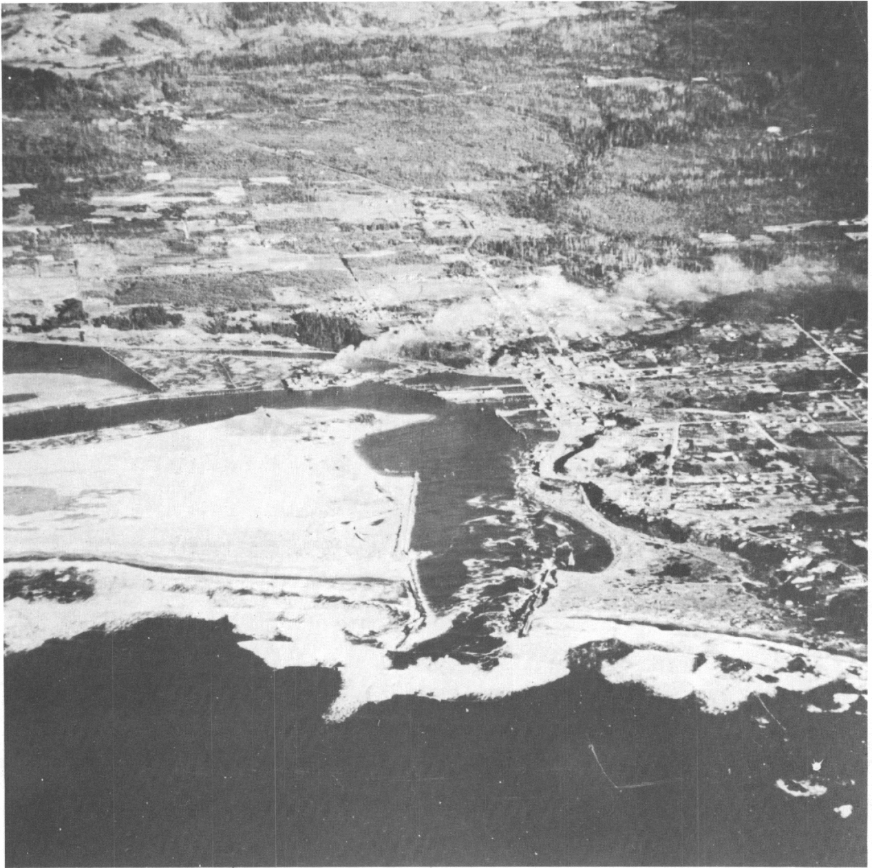
Fig. 5. Coquille River entrance. This entrance is improved by two jetties, the northern one being a monolithic concrete structure. Depths on the entrance are sufficient for coastal lumber schooners of light draft. The surf existing at the time this photograph was taken would preclude use of this entrance by any craft. In the summer and prior to winter freshets, bars are apt to shoal.
