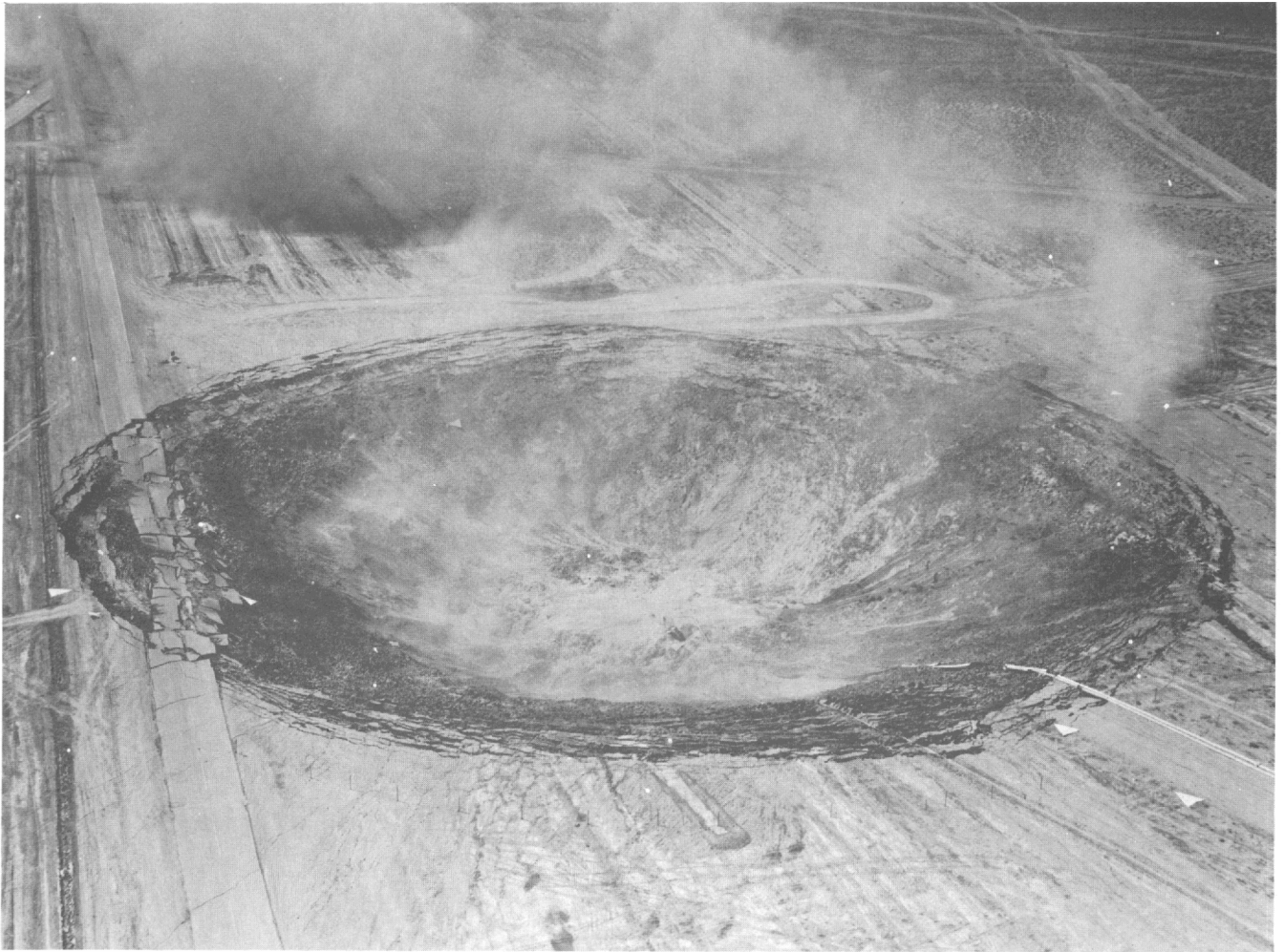
Fig. 10. Aerial view of a typical subsidence crater taken several seconds after collapse.
