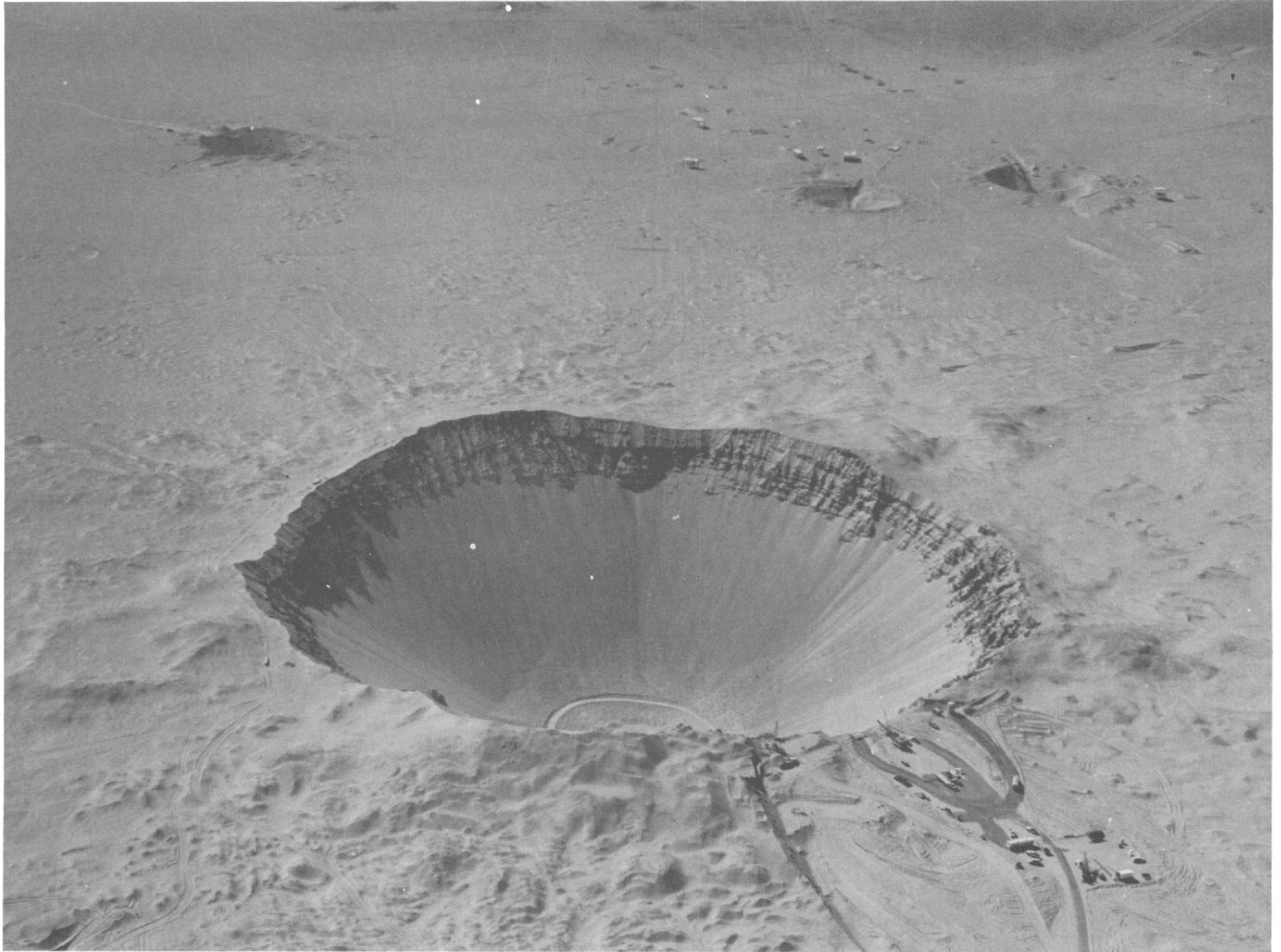
Fig. 6. Aerial view of Area 10, NTS showing the 100-kt Sedan crater in the foreground and three earlier kiloton-range craters.
