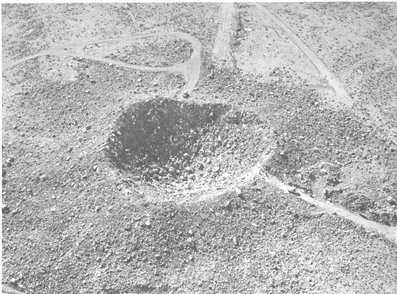
Fig. 14. Aerial view of Danny Boy crater showing particle size of fallback in relation to vehicles on lip.
