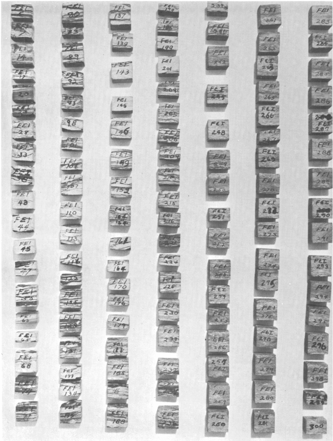
Fig. 7. Photograph of porosity-permeability plugs of a low deliverability gas reservoir showing laminations.
