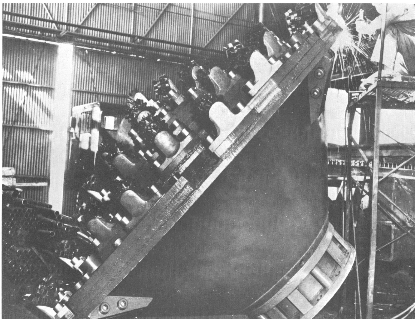
Fig. 8. View of a plate type large diameter drill bit. Photo-Hughes Tool Company.
