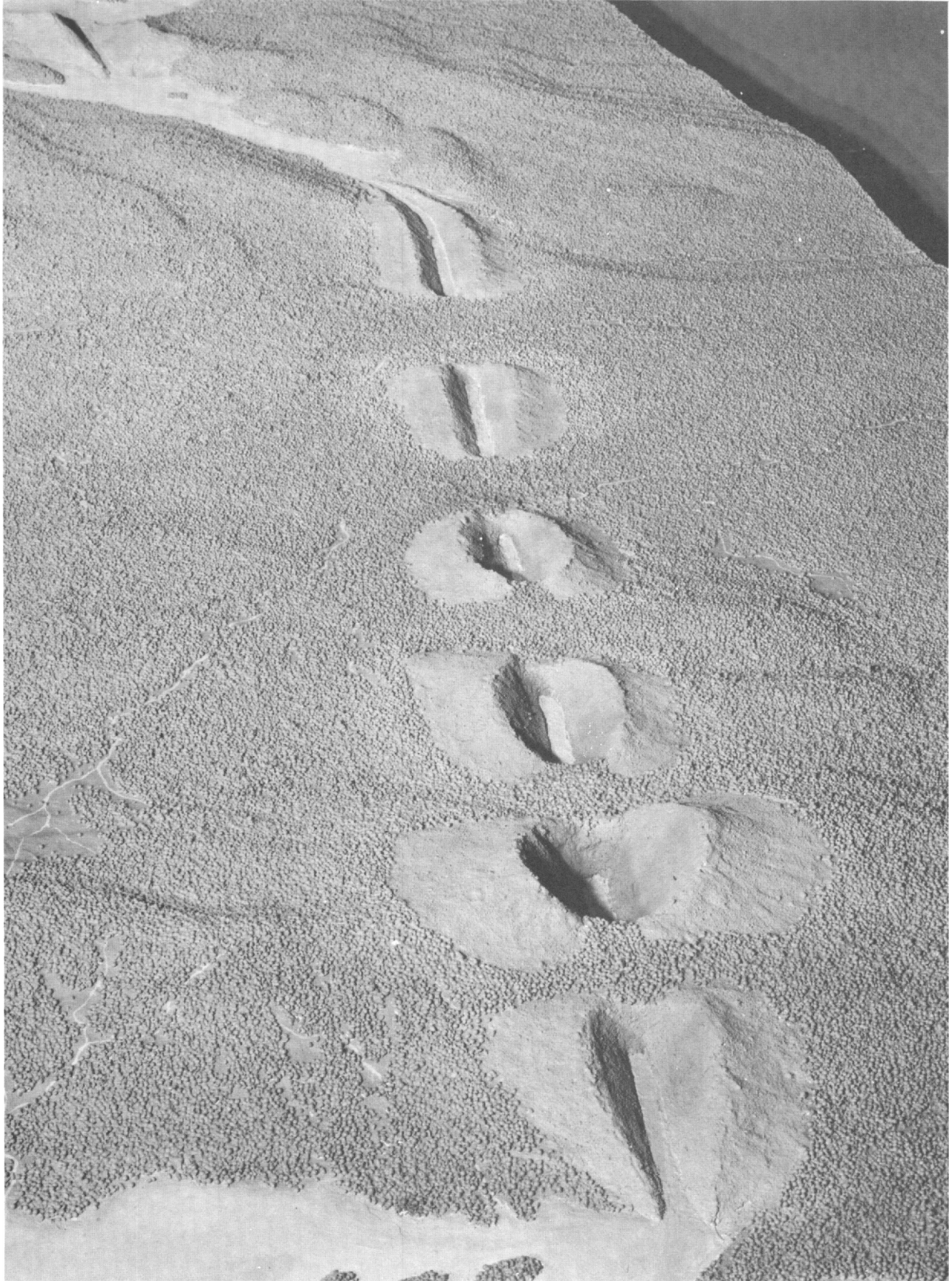
Fig. 5. Model of Route 17 showing nuclear excavations from Detonations 1-9.
