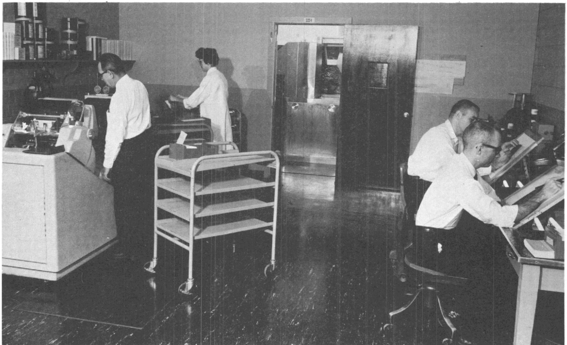
Fig. 2—Sequential card cameras photograph text typed on cards. Indexes for Nuclear Science Abstracts are run at 230 lines per minute, on paper for editing, and on film in a single roll negative. The film is stripped into a two-column page negative on vacuum-equipped light tables (right). Developing room at rear.
