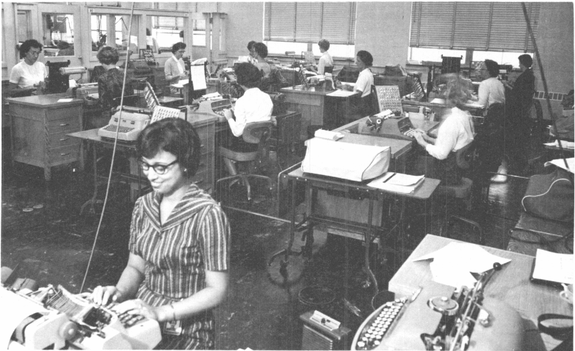
Fig. 1—Composing of reproducible copy. Racks hold demountable type bars carrying 180 Greek letters and mathematical characters for use in setting equations. Proofreading and correction rooms at left.
