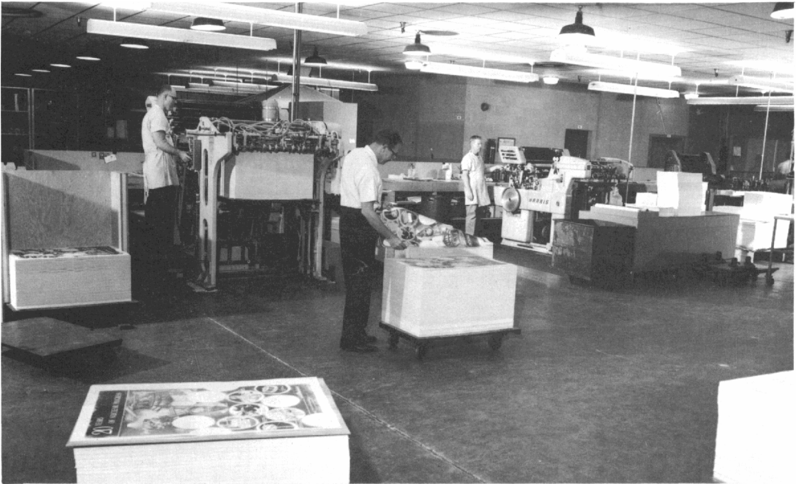
Fig. 3—Offset printing is done on eight-page press (left), two four-page presses (right), and a number of smaller presses.
