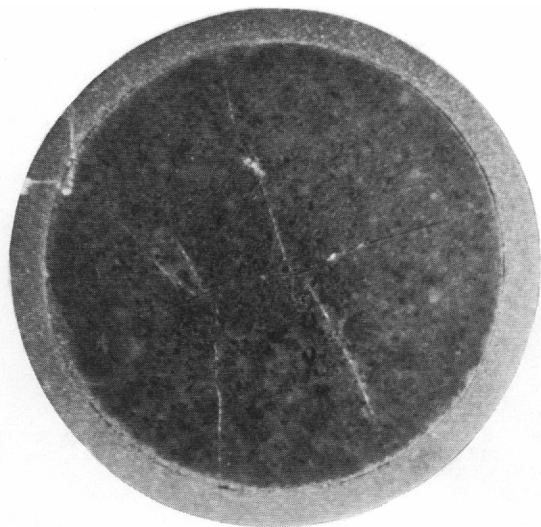
Figure 42. Transverse View of Ground and Etched Oxide Fuel Pellet after Two Seed Lives of Operation; X6.6.
