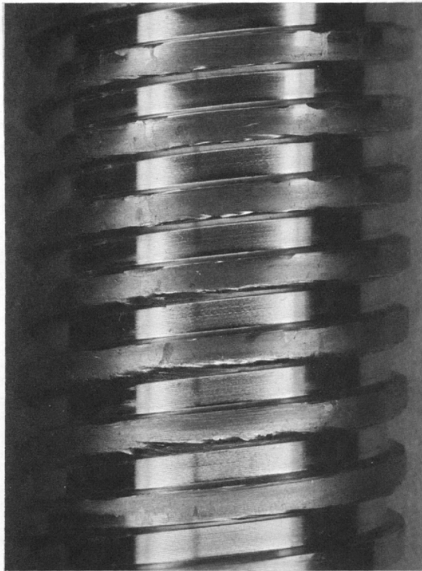
Figure 38. Latch Area of E-12 Lead Screw after Seed 2 Life; X8.
