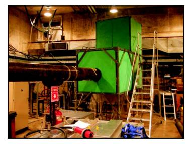
Figure 6. The assembled experimental system showing the polyethylene shielding structure surrounding the graphite heating system.
