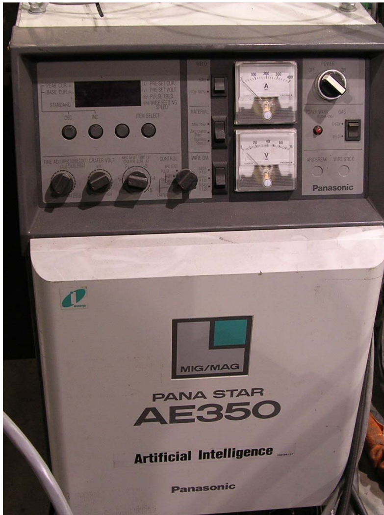
Figure 38 - Panasonic AE 350 Power Supply with Pulse Short-Circuit Metal Transfer Control
