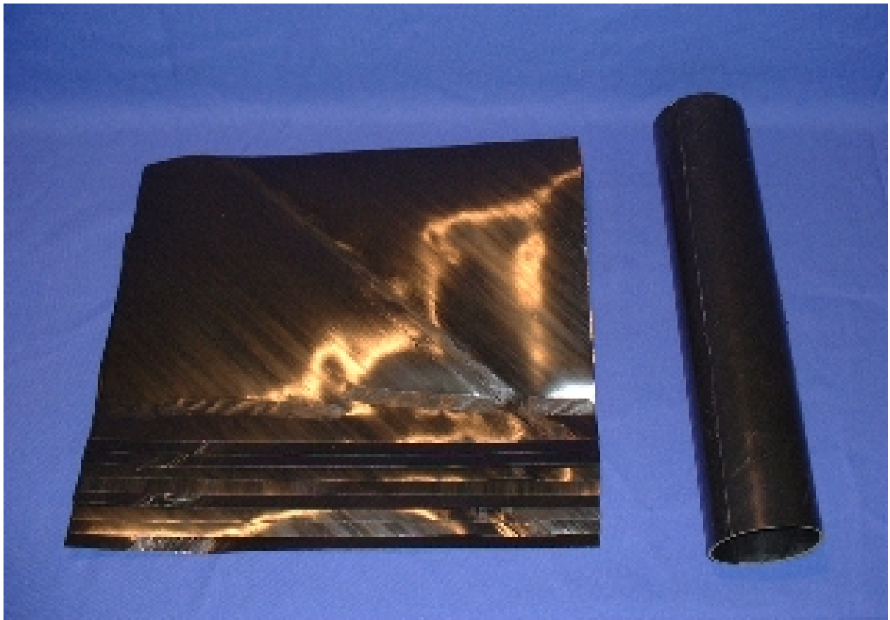
Figure 7 - Lay-Up and Forming of Fiber-Reinforced Composite Liner
