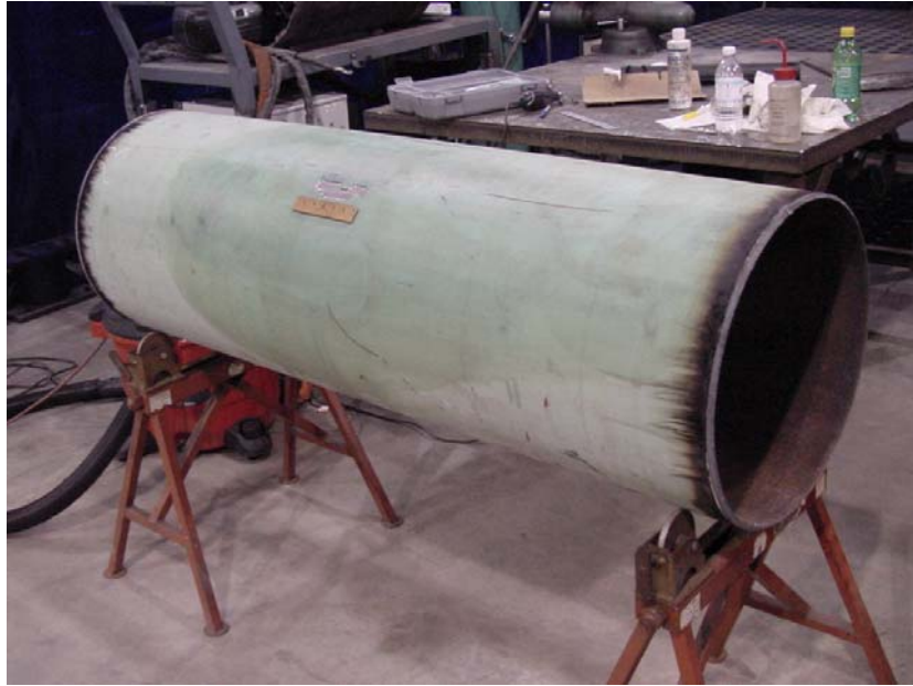
Figure 15 - 508 mm (20 in.) Diameter API 5L-X52 Pipe Section Used for Carbon Fiber Liner Repair Test
