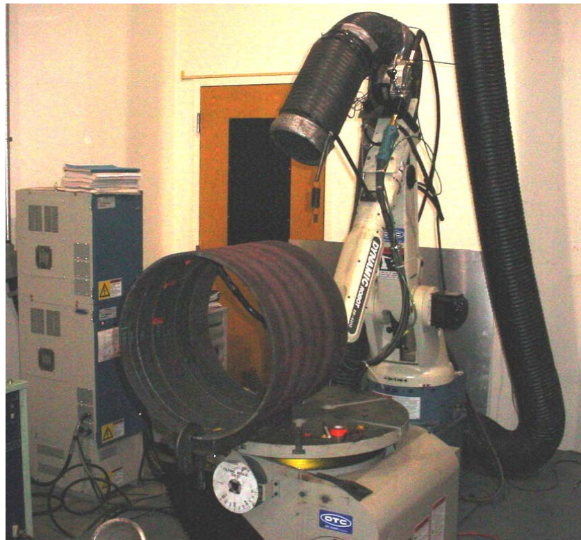
Figure 33 - OTC Robot Set-Up for Internal Welding
