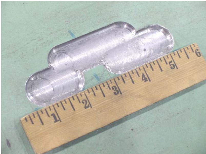
Figure 16 - Simulated Corrosion Defect for Carbon Fiber Liner Repair Test in 508 mm (20 in.) Diameter Pipe
