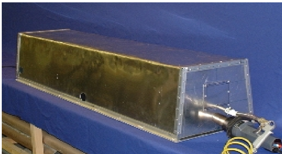
Figure 10 - Oven Used to Heat Pipe and Liner to 200°C (392°F)
