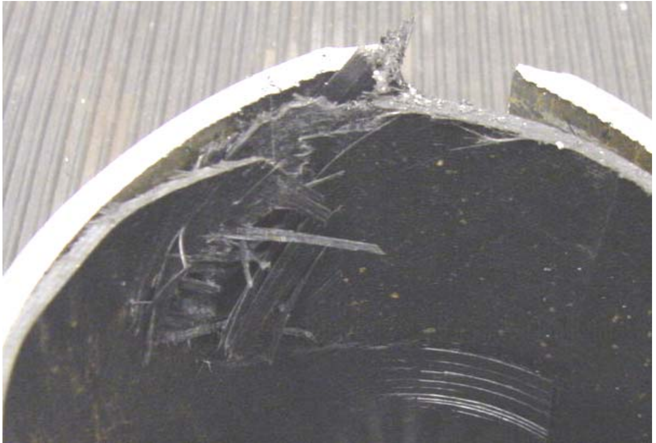
Figure 79 - Pipe Sample Containing Round-Bottom Longitudinal Slot Showing Rupture of Liner Material
