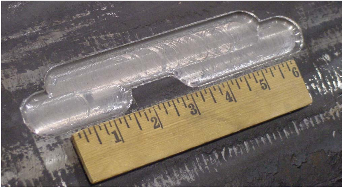
Figure 42 - Magnified View of Simulated Corrosion on 558.80 mm (22 in.) Pipe
