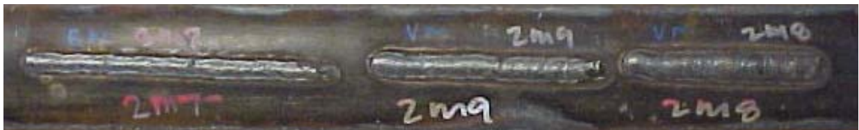
Figure 101 - External Appearance of Welds Made on 3.2 mm (0.125 in.) Thick Pipe with Methane Gas at 4.5 mPa (650 psi) and 6.1 m/sec (19.9 ft/sec) Flow Rate
