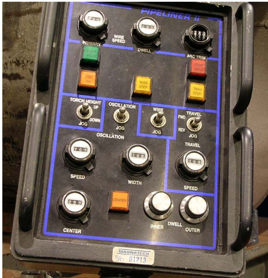
Figure 37 - Magnatech Control Pendant Showing Control Parameters
