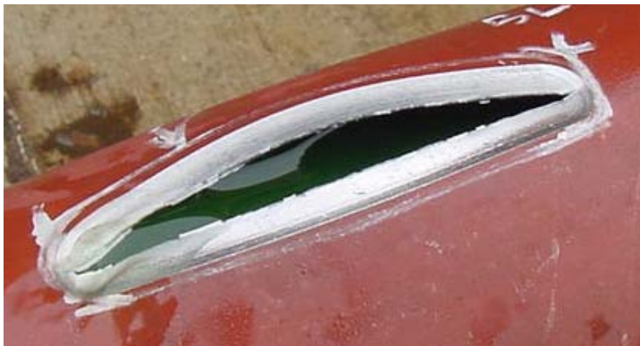
Figure 74 - Pipe Section with Long, Shallow Simulated Corrosion Damage – Without Liner - Following Hydrostatic Pressure Test
