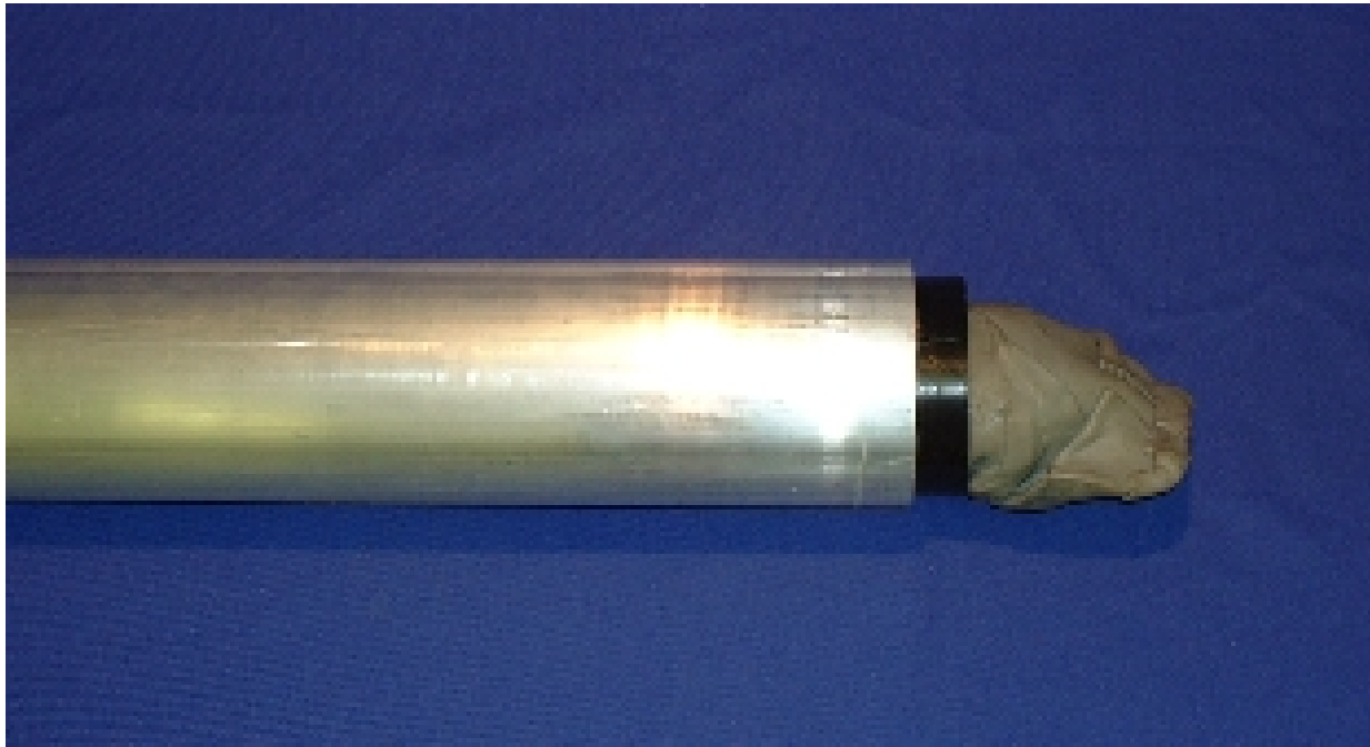
Figure 9 - Silicon Rubber Bag Inserted into Liner
