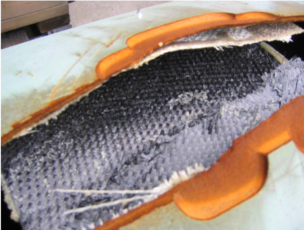
Figure 93 - Magnification of Carbon Fiber-Reinforced Patch After Burst Test
