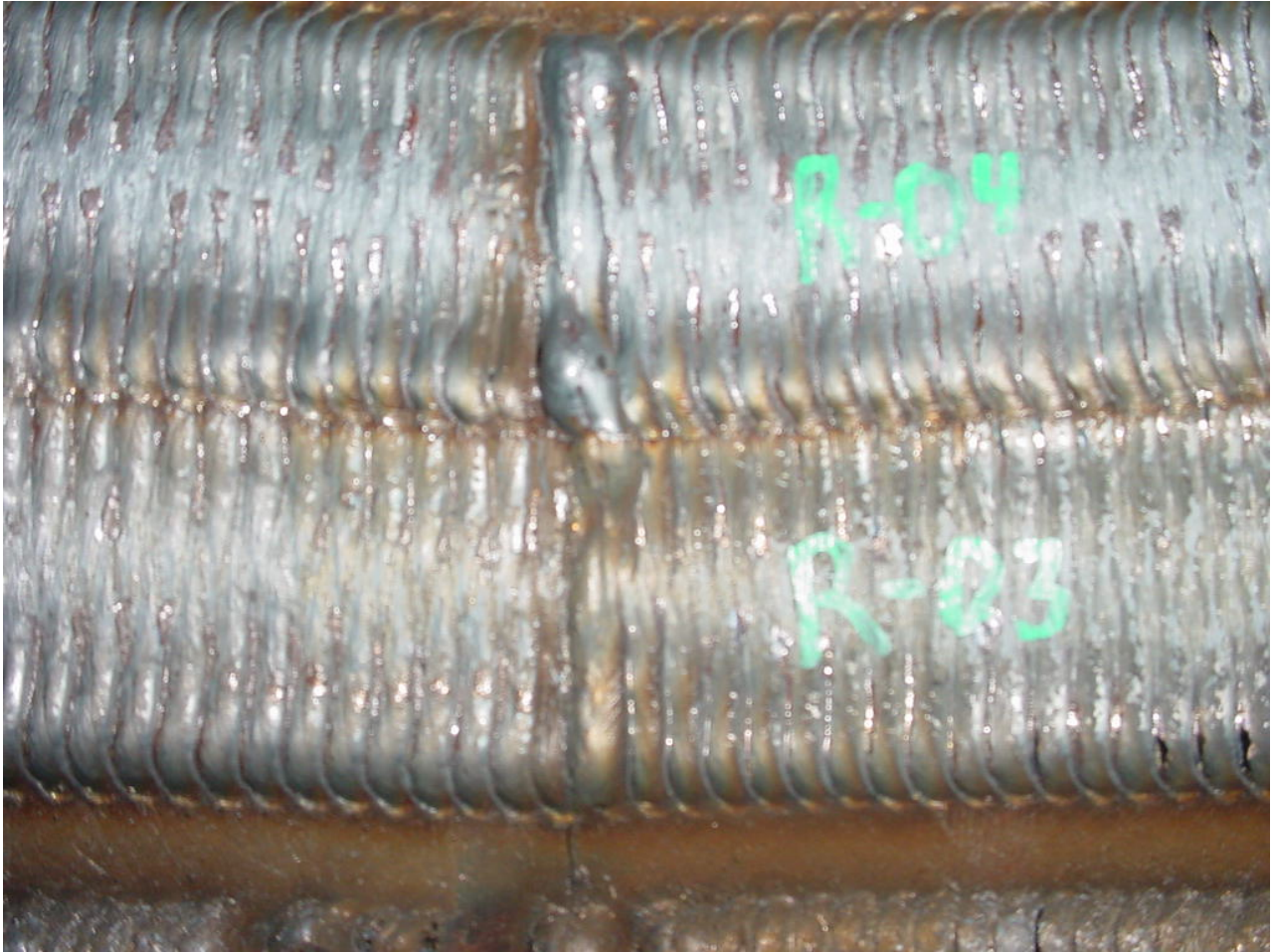
Figure 84 - Tests R-03 and R-04 at 12:00 Showing Better Stop-Start Overlap.
