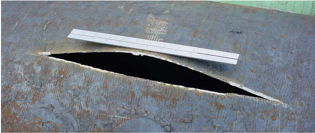
Figure 116 - Hydrostatic Burst Specimen of 558.8 mm (22 in.) Pipe in Virgin Pipe
