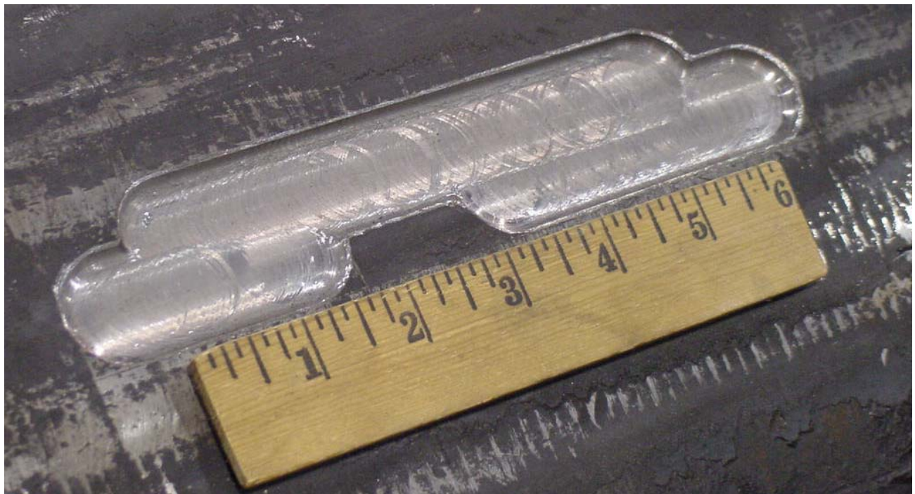
Figure 87 - Selected Configuration of Simulated Damage for 558.80 mm (22 in.) Diameter Pipe Sections
