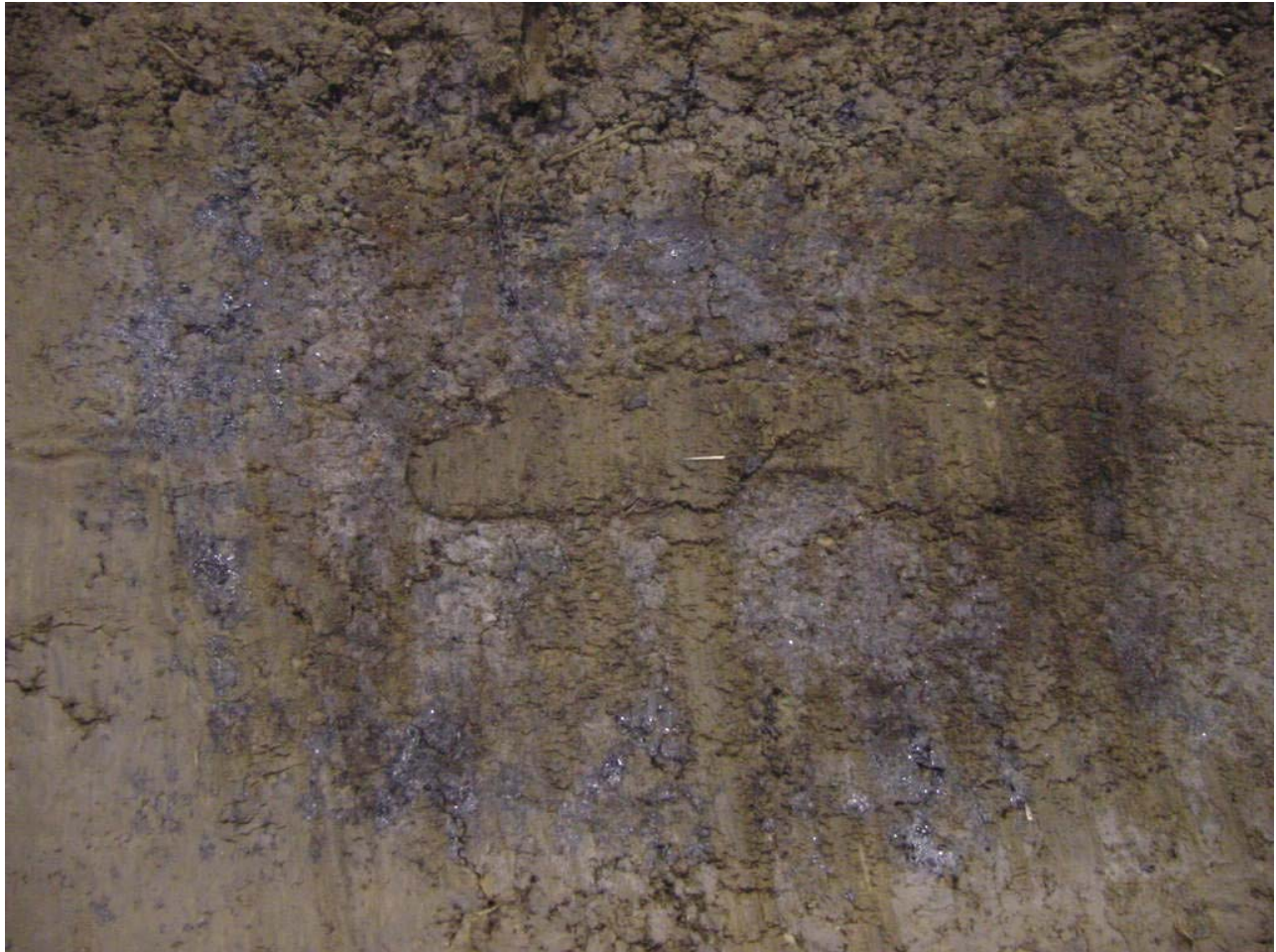
Figure 96 - Dirt That Was In Contact With Pipe During Internal Weld Deposition Repair
