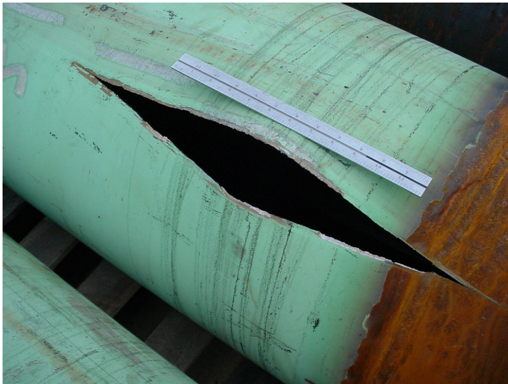
Figure 114 - Hydrostatic Burst Specimen of 508.0 mm (20 in.) in Virgin Pipe
