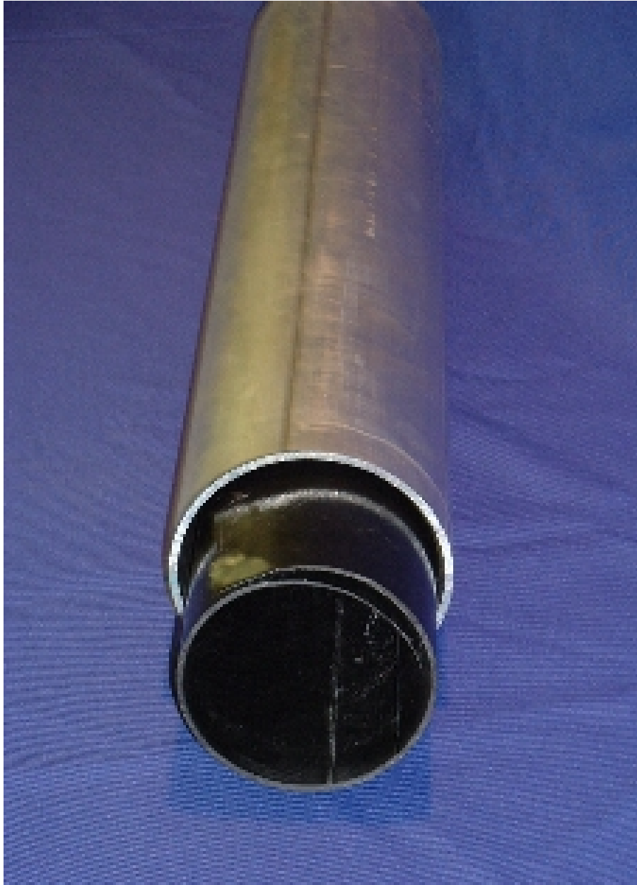
Figure 8 - Insertion of Liner into 114.3 mm (4.5 in.) Diameter Pipe
