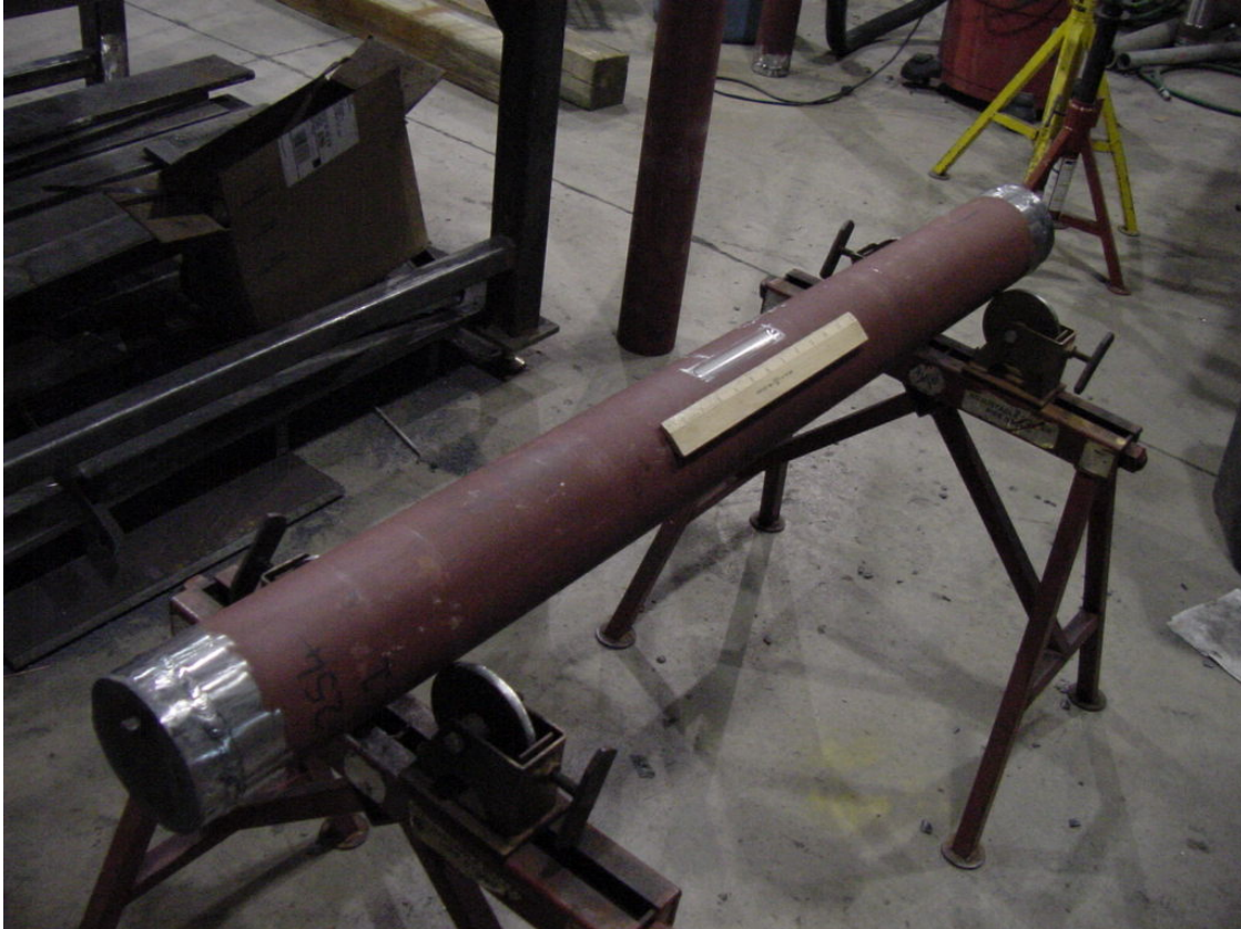
Figure 14 - 114.3 mm (4.5 in.) Diameter Pipe Section with End Caps Welded and Simulated Corrosion Damage
