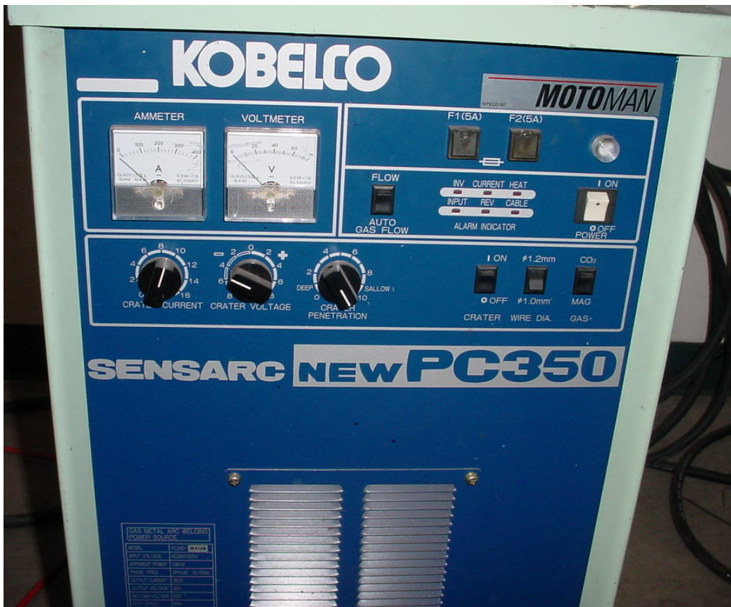
Figure 35 - Kobelco PC-350 Variable Polarity Fuzzy Logic Power Supply
