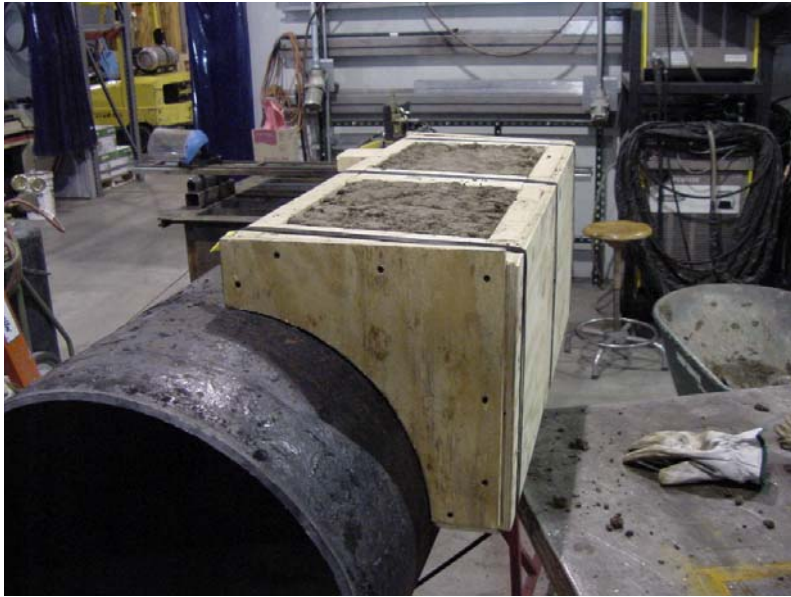
Figure 43 - Dirt Box for Weld Deposition Repair
