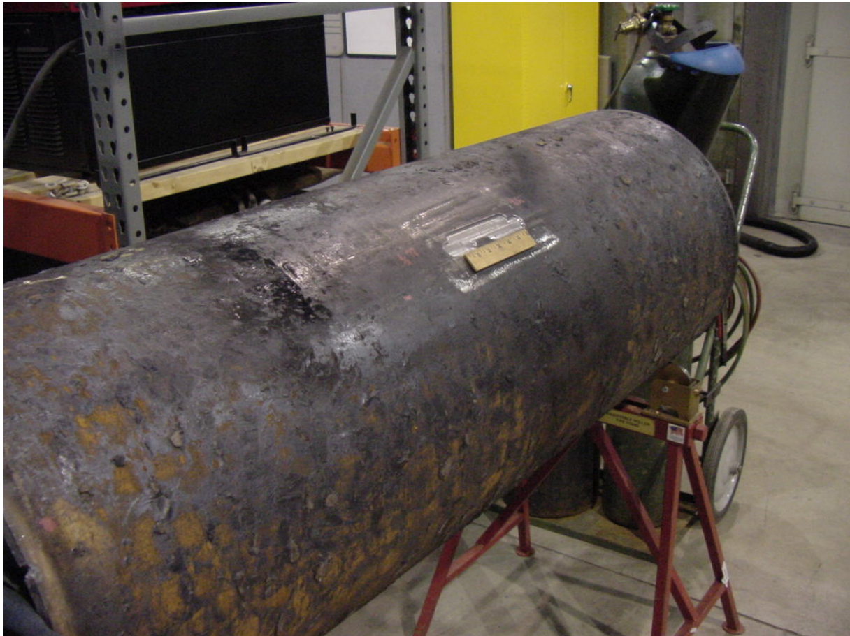
Figure 41 - Simulated Corrosion on 558.80 mm (22 in.) Pipe
