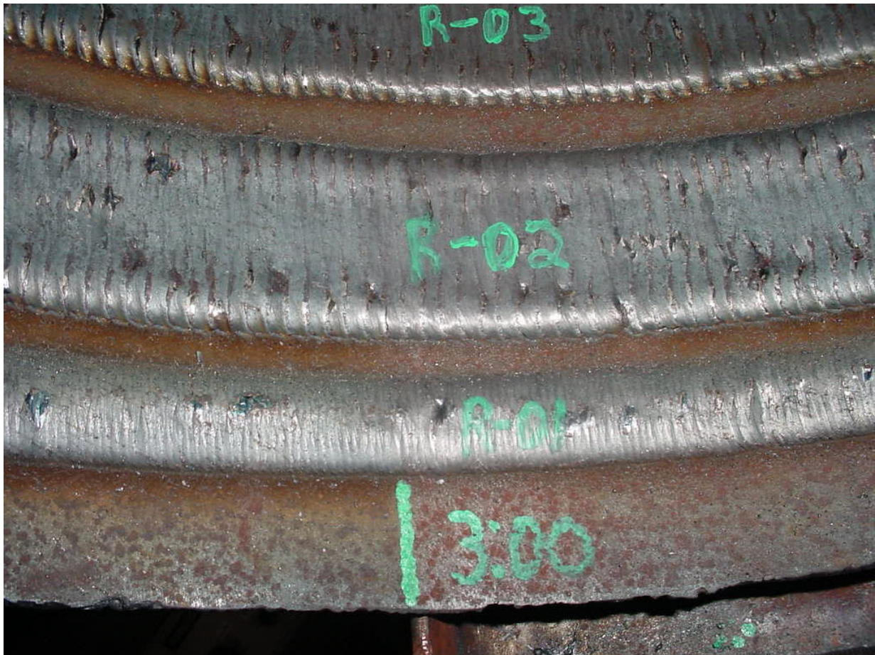
Figure 85 - Tests R-01 and R-02 at 3:00 Showing Steady-State Bead Shape
