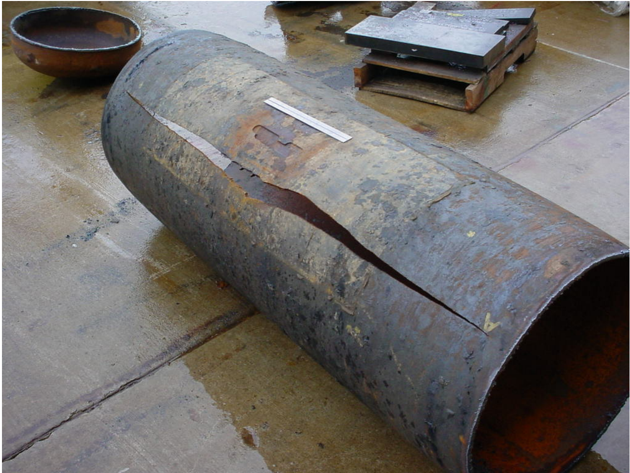
Figure 99 - Pipe Section with Internal Weld Deposition Repair After Hydrostatic Burst Test
