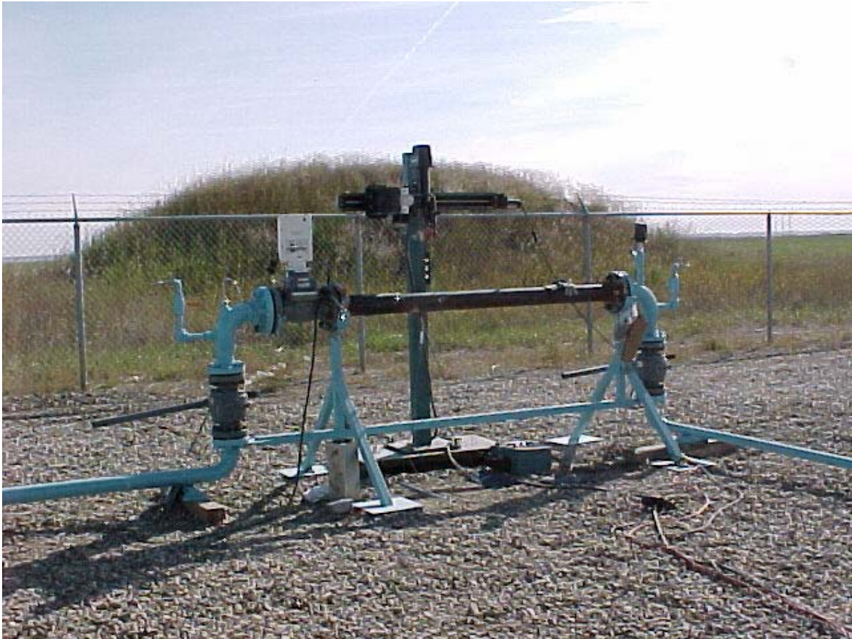
Figure 100 - Experimental Set-Up for Welding onto Thin-Wall Pipe containing Pressurized Methane Gas
