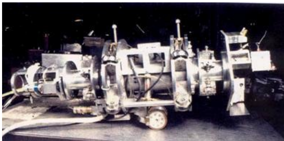
Figure 3 - Osaka Gas System for Remote Robotic Internal Repair of Root Weld Defects in Gas Transmission Pipelines
