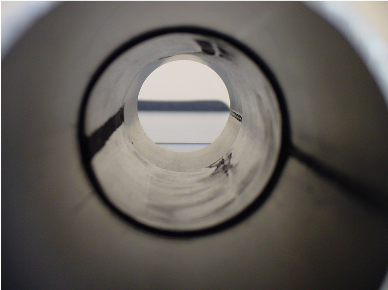
Figure 11 - Liner Inserted into Center of 114.3 mm (4.5 in.) Diameter Pipe
