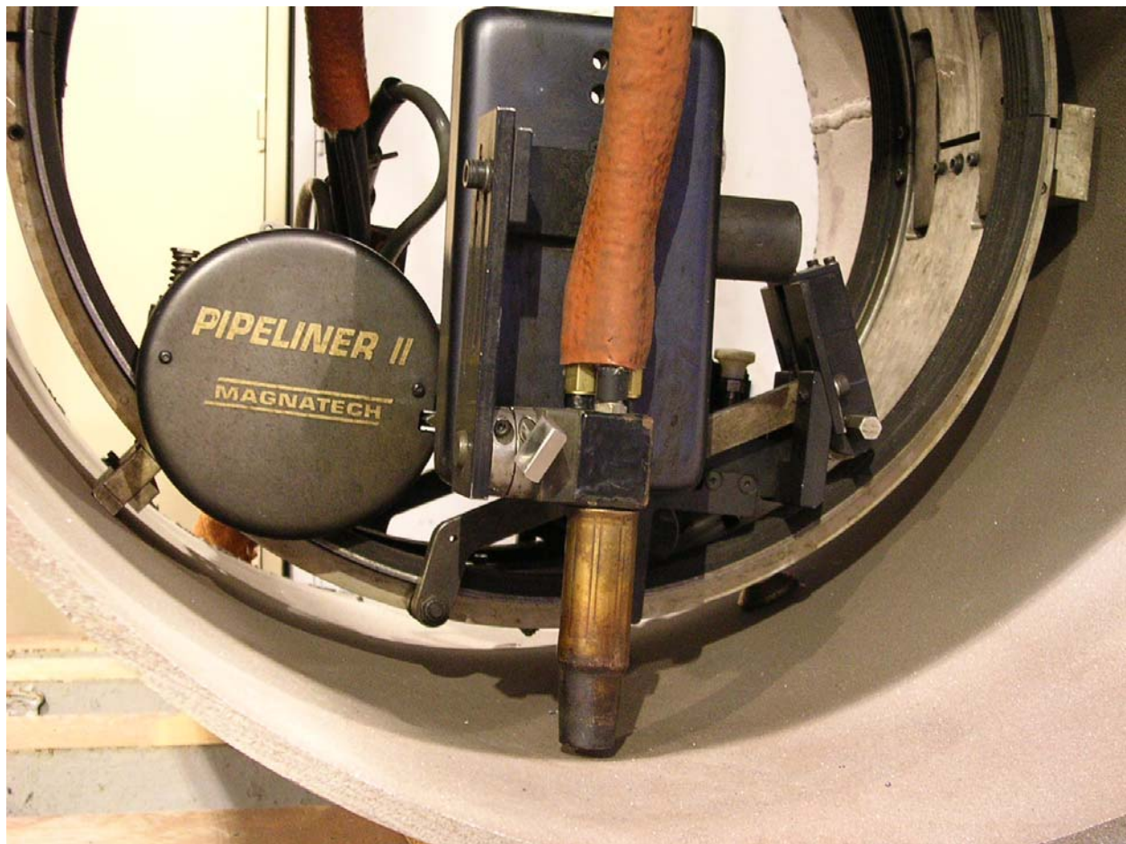
Figure 36 - Magnatech ID Welding Tractor Capable of Spiral & Ring Motion with Oscillation
