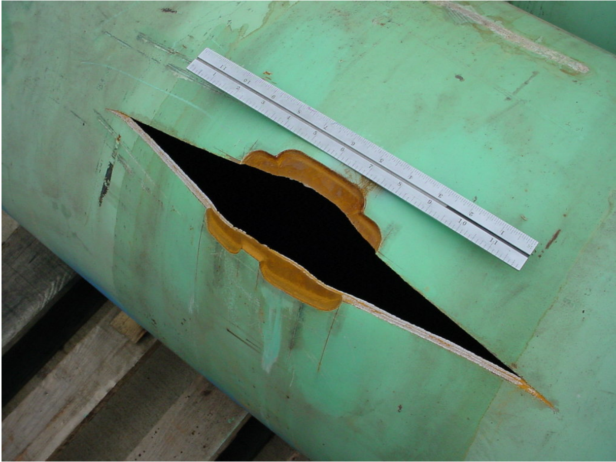
Figure 115 - Hydrostatic Burst Specimen of 508.0 mm (20 in.) with Un-Repaired Damage
