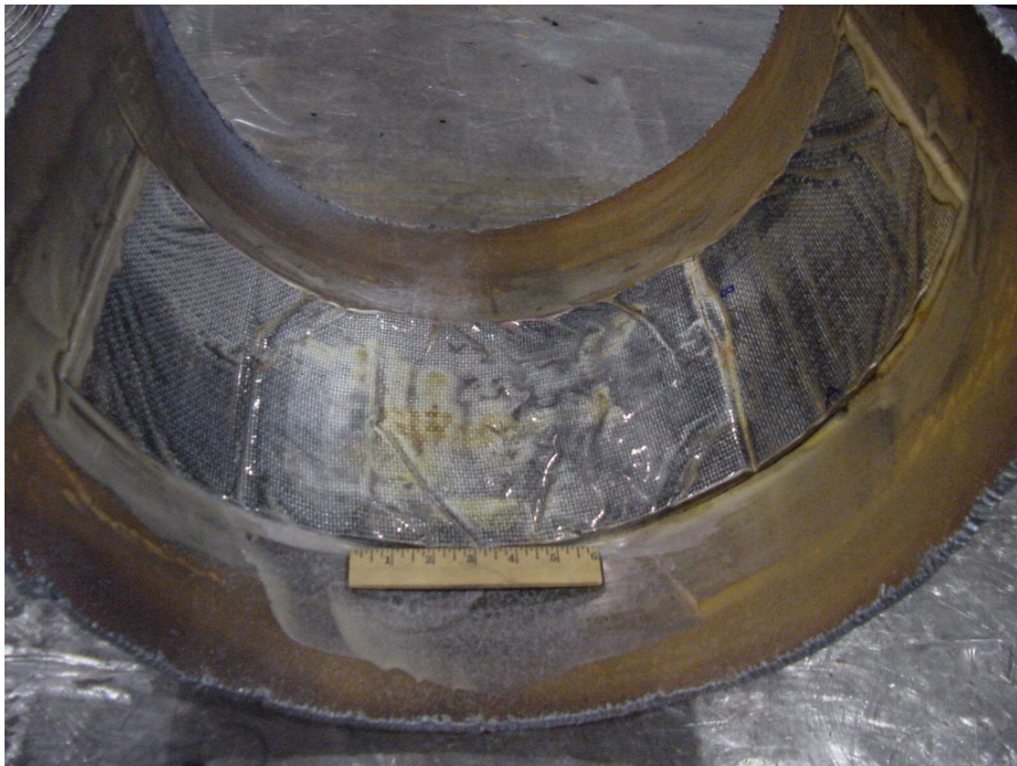
Figure 28 - Pressure Bandage Carbon Fiber-Reinforced Patch Configuration
