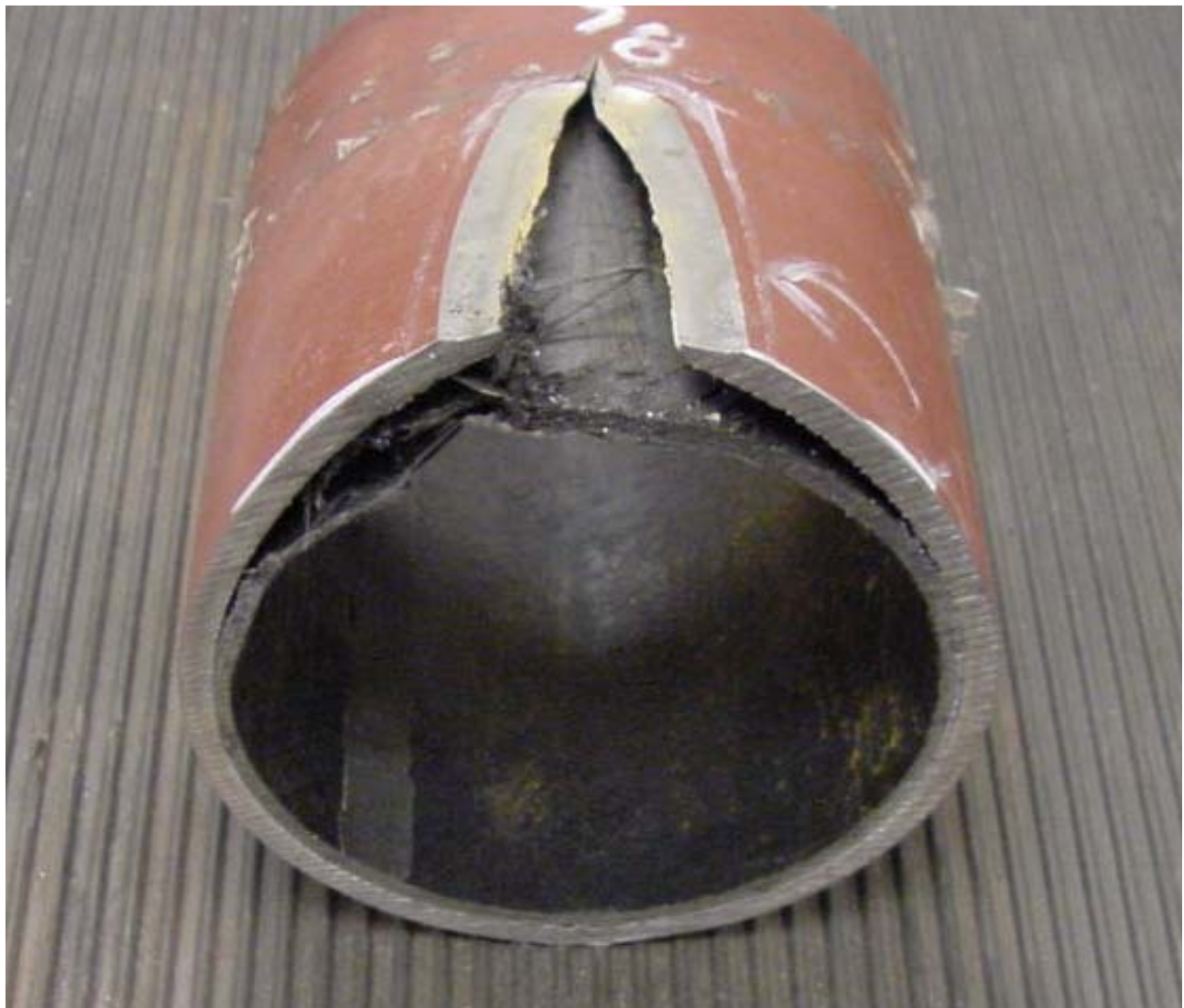
Figure 78 - Water-Jet Cut Section through Pipe Sample Containing Round-Bottom Longitudinal Slot with Liner Installed
