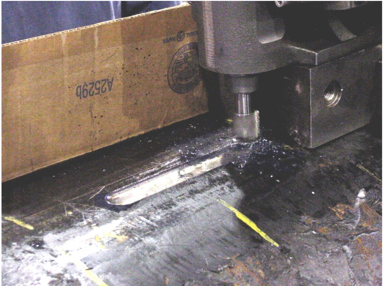
Figure 39 - Milling Machine Set-Up Used to Simulate Corrosion on Pipe Sections
