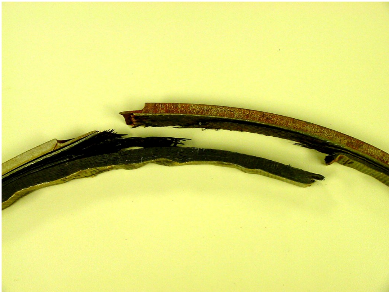
Figure 119 - Failure of Pipe and Composite Repair
