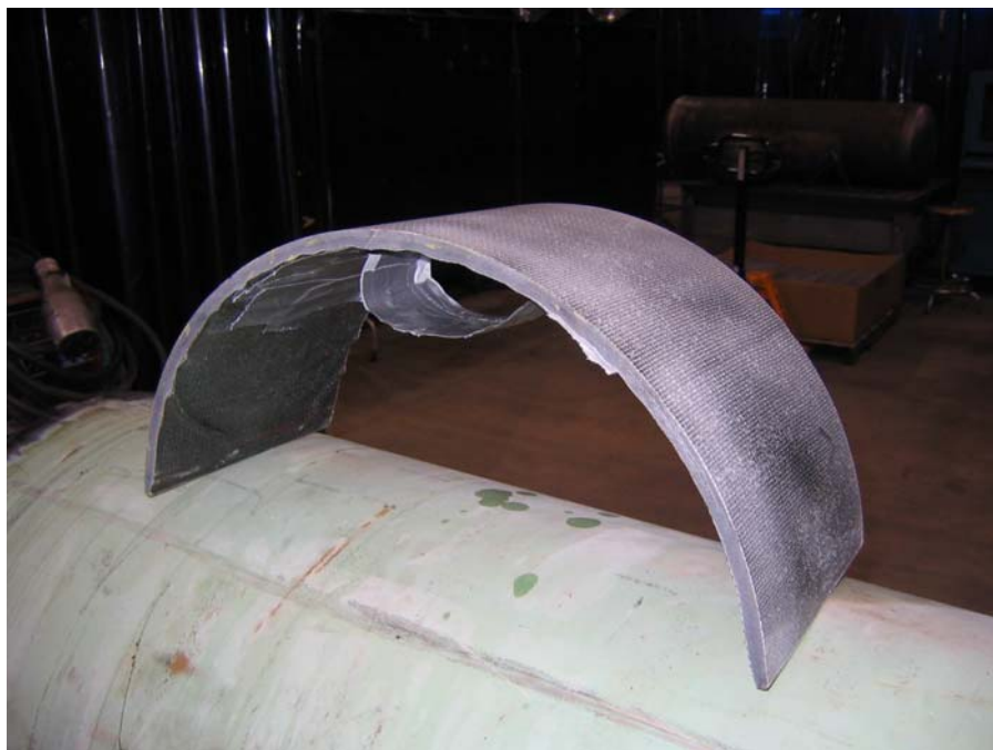
Figure 22 - Completed Repair Patch with Grit-Blasted Outer Diameter
