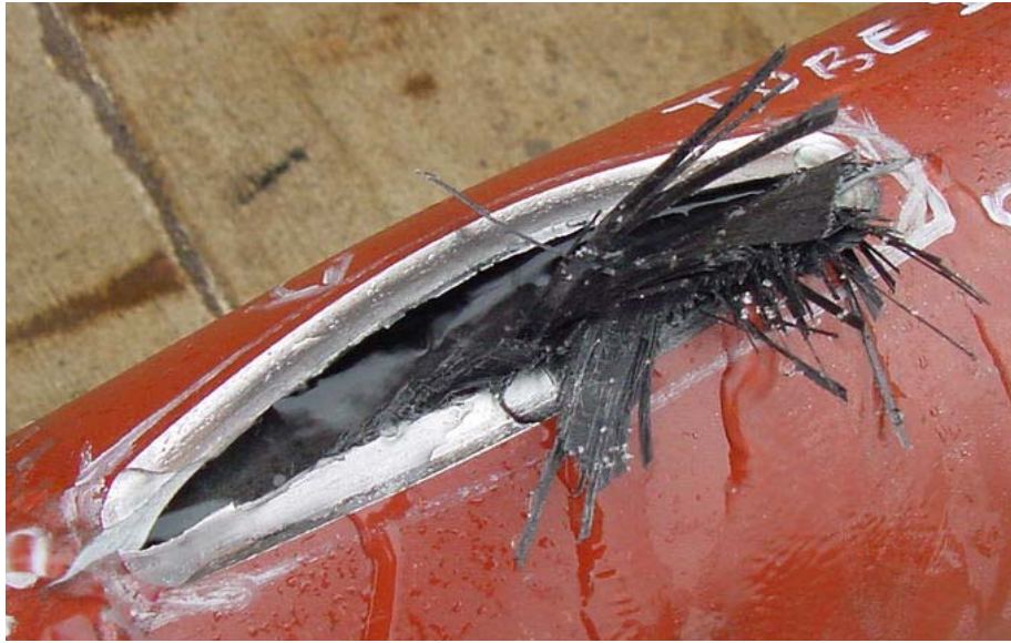
Figure 75 - Pipe Section with Long, Shallow Simulated Corrosion Damage – With Liner – Following Hydrostatic Pressure Test
