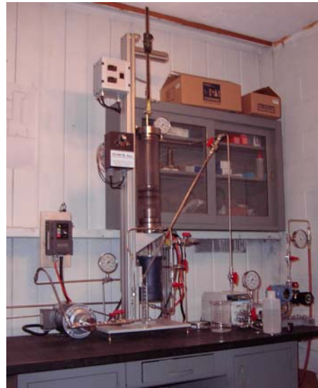
Fig. 3.2 Foam Generator Assembly
