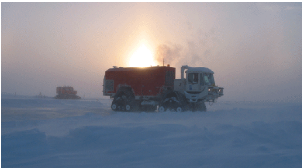
Figure 10. PGS Vibrator during VSP Production Recording
