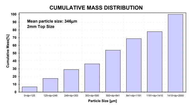
Figure 7: Particle Size Distribution of the Minus 2mm Lignite
