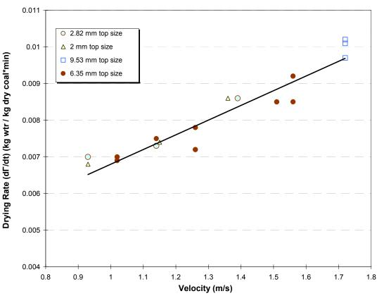
DRYING RATE VERSUS VELOCITY
