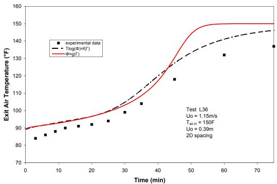
Figure 20: Exit Air Temperature for Test 36 – Comparison of Predictions From Two Equilibrium Models
