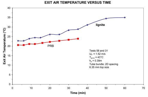
Figure 13: Comparison of Exit Air Temperatures for Lignite and PRB Coals for a 43°C Drying Temperature
