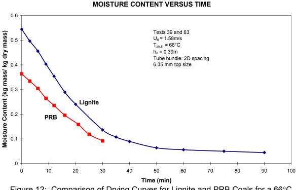
Figure 12: Comparison of Drying Curves for Lignite and PRB Coals for a 66°C Drying Temperature
