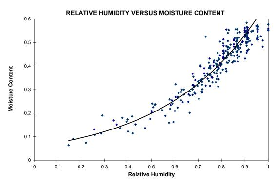
Figure 16: Equilibrium Relative Humidity of Air Versus Moisture Content of Lignite
