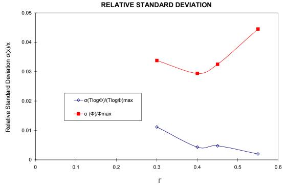
Figure 18: Relative Standard Deviation for the Two Equilibrium Moisture Models
