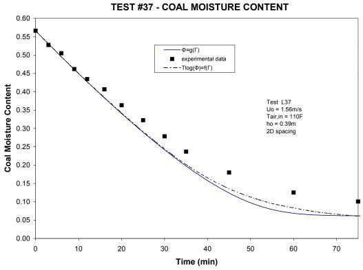
Figure 23: Drying Curve for Test 37 – Comparison of Predictions From Two Equilibrium Models
