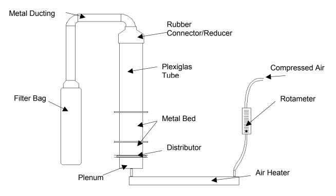
Figure 6: Sketch of Experimental Bed Setup
