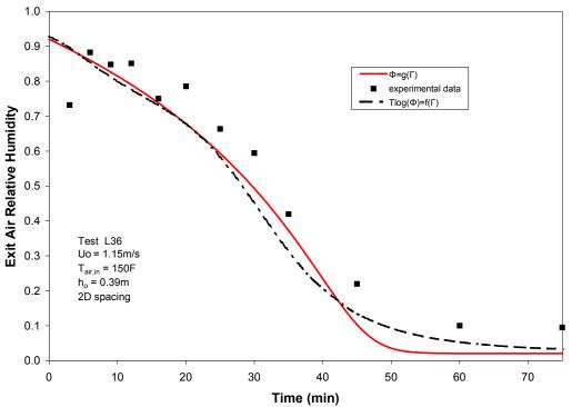
Figure 22: Exit Air Relative Humidity for Test 36 – Comparison of Predictions From Two Equilibrium Models
