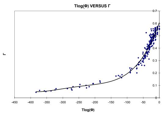
Figure 17: Improved Model for Equilibrium Relative Humidity of Air Versus Moisture Content of Lignite
