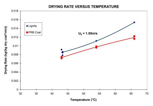
Figure 15: Comparison of Drying Rates for Lignite and PRB
