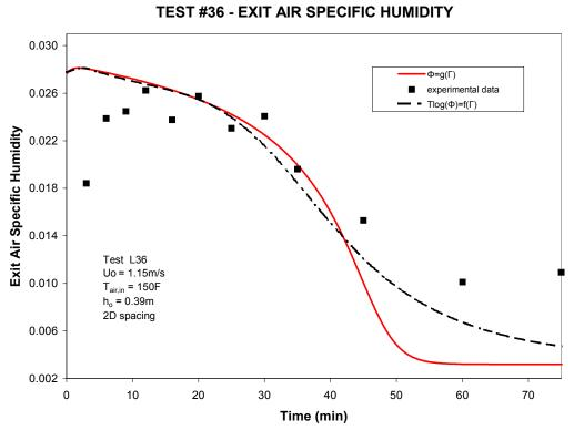
Figure 21: Exit Air Specific Humidity for Test 36 – Comparison of Predictions From Two Equilibrium Models
