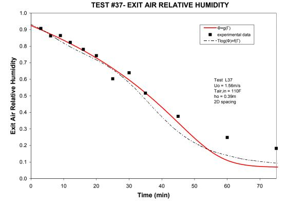
Figure 26: Exit Air Relative Humidity for Test 37 – Comparison of Predictions From Two Equilibrium Models
