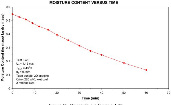
Figure 9: Drying Curve for Test L45
