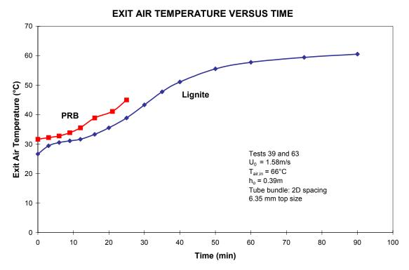
Figure 14: Comparison of Exit Air Temperatures for Lignite and PRB Coals for a 66°C Drying Temperature
