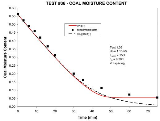
Figure 19: Lignite Drying Curve for Test 36 – Comparison of Predictions From Two Equilibrium Models
