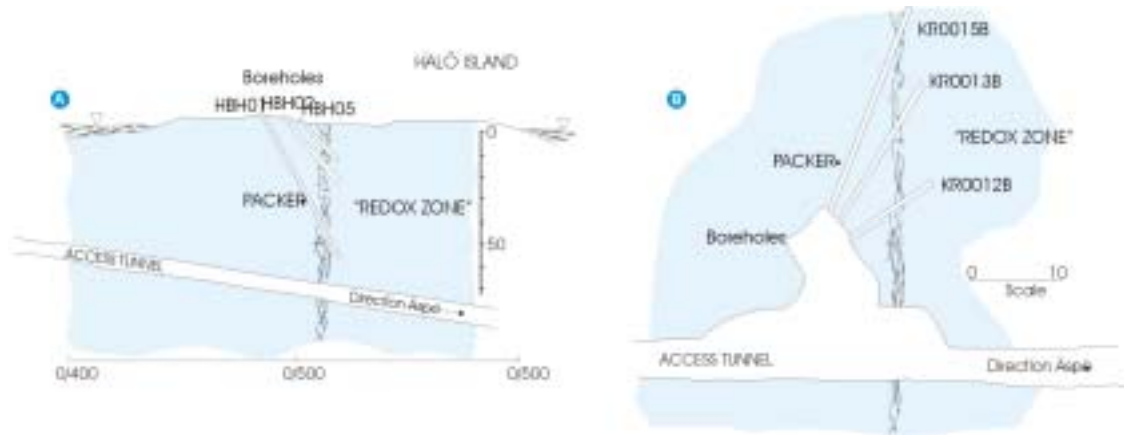
Figure 2-2. Cross-section and plan view of the Redox Zone Experiment: A) Cross-section view with the location of boreholes drilled from the surface (HBH01, HBH02 and HBH05); and B) Plan view with the location of boreholes drilled from the tunnel at a depth of 70 m (KR0012B, KR0013B and KR0015B). Modified from /Gustafsson et al, 1994/.
