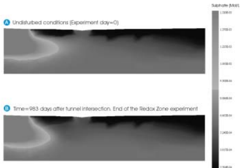
Figure 3-26. Numerically computed sulphate concentrations distribution (Mol/L). A) Undisturbed conditions, prior to tunnel intersection. B) End of the experiment (983 days after tunnel intersection).
