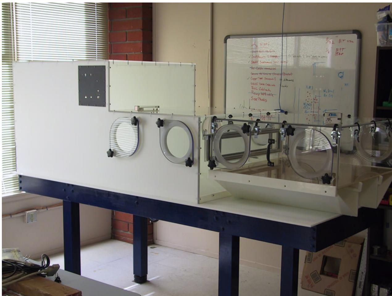
**Figure 20:** N<sub>2</sub> housing for the old alpha detector, including a sample glove box.
