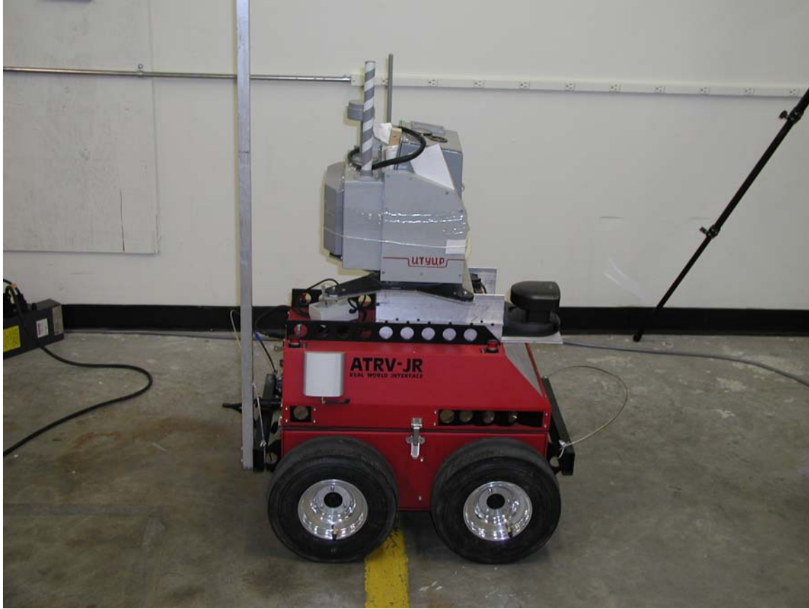
Figure 4. The GLD/IID on an INEEL robot was used to survey a hot area to limit personnel exposure.
