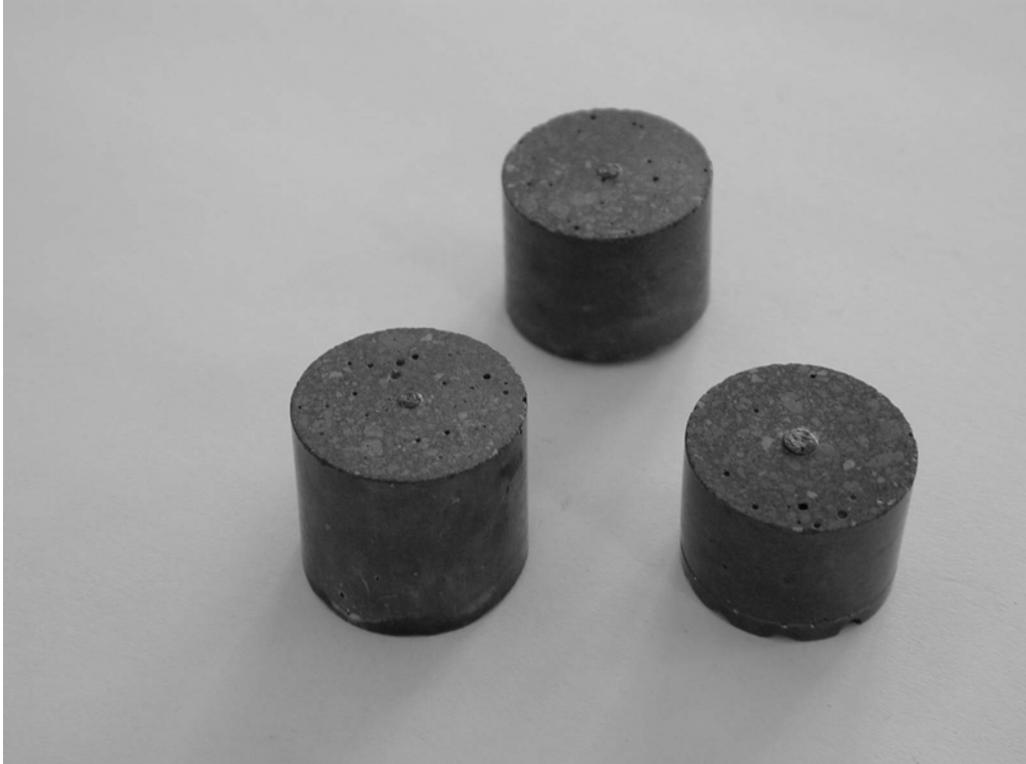
Fig.4 Graphite concrete samples, diameter 21 mm
