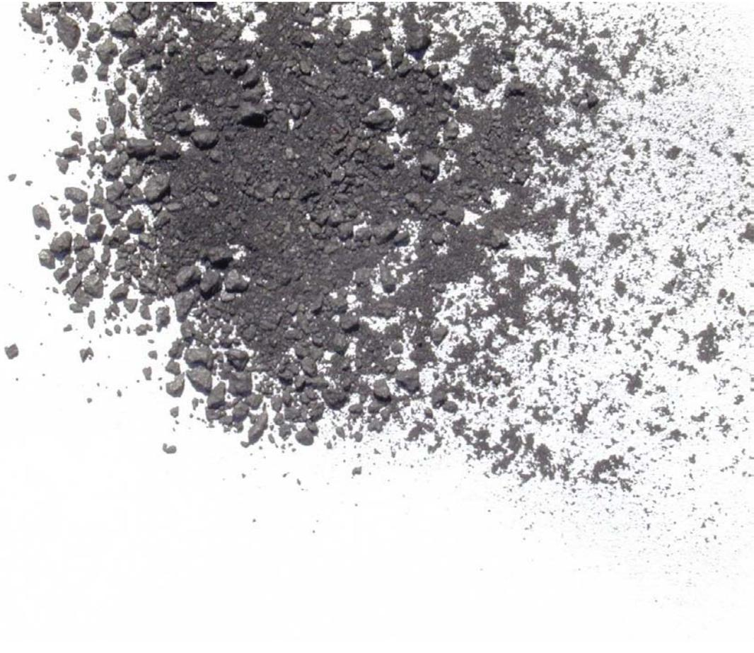
Fig. 3 Crushed graphite, maximum particle size 6 mm
