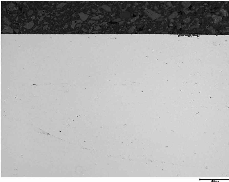
Figure 8: Optical Micrograph of the Super 304H Sample (750°C)
