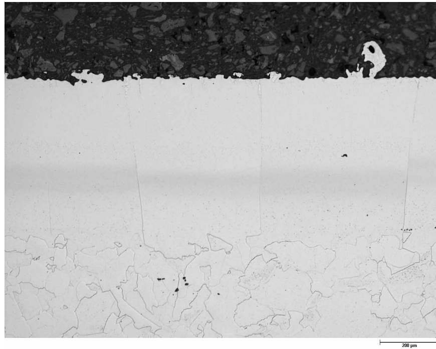
Figure 1: Optical Micrograph of the Grade 92 Si-Cr Sample (750°C)
