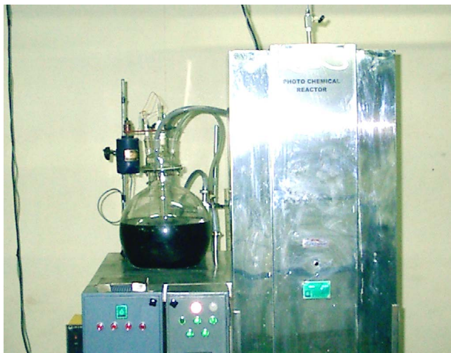
Fig. 1. Tubular Flow Photochemical Reactor system
