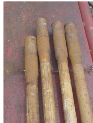
After 160,000 cycles, the pipe exhibits little to no signs of wear.
