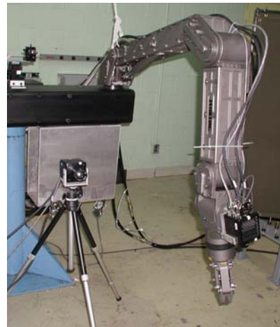
Figure 1: Experimental test bed including a Schilling Titan II hydraulic manipulator with a fixed camera and an in-hand camera.
