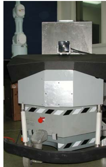
Figure 2: Experimental test bed including a K2A mobile robot and on-board camera.
