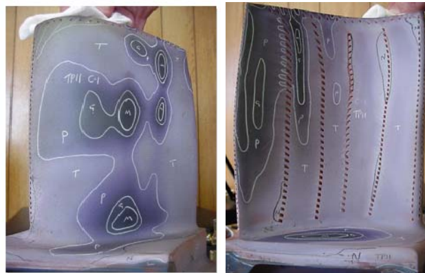
Figure 105 Thermal Paint Test Results on First Stage Blade
