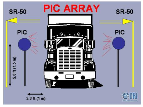
Figure 5. Front view schematic of PIC array.
