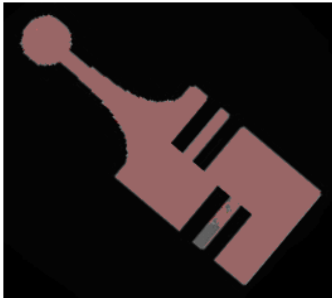
Section I-Figure 5.14: CastView result for finger part using new algorithm. The second finger is the last region to be filled.
