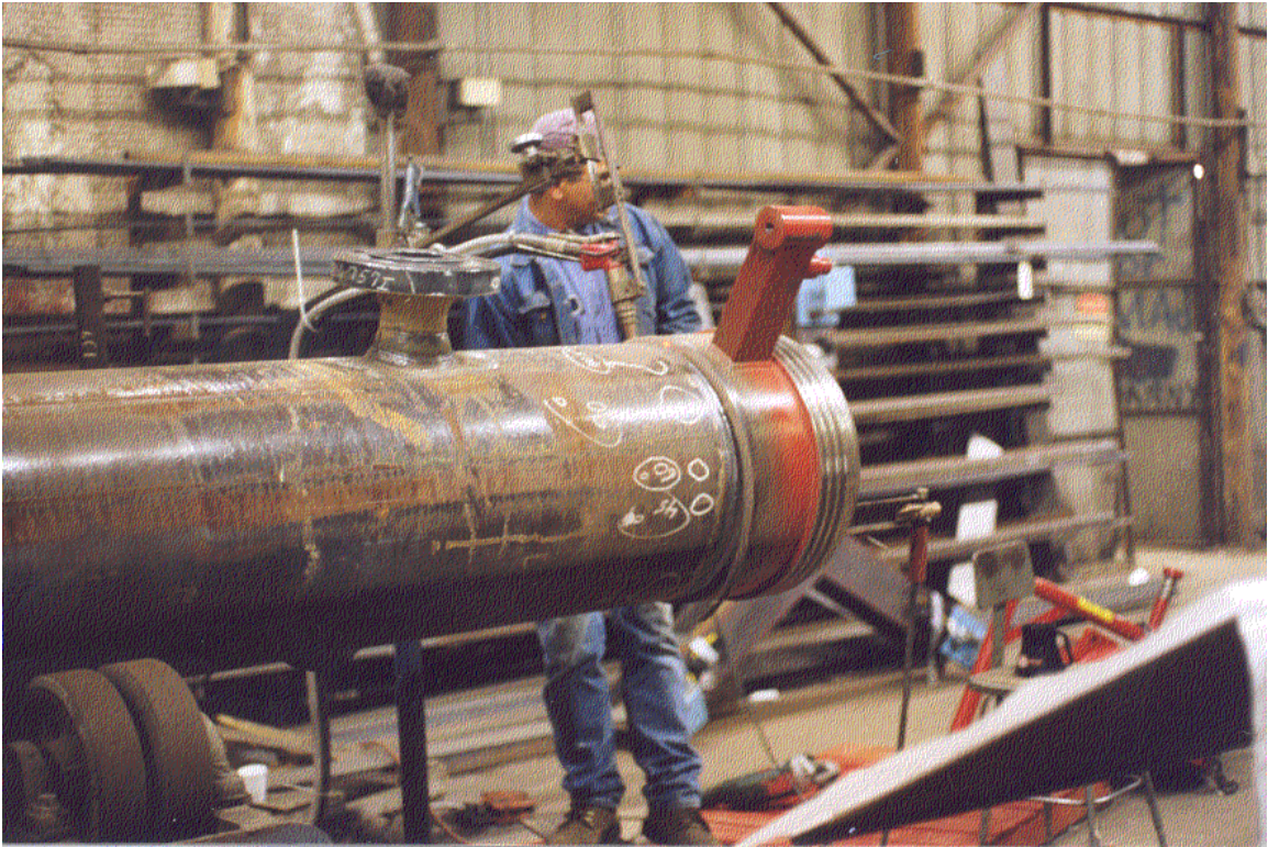
Figure 3.3 - Fabrication of Cuttings Injection Hopper
