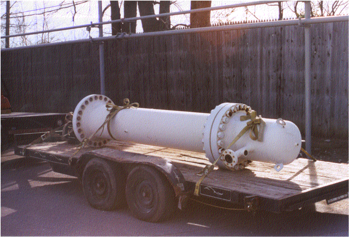
Figure 3.1 - Existing Foam Breaker Tower
