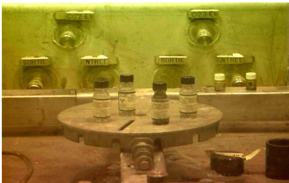
Figure 7: ^{243}\text{Am} , ^{240}\text{Pu} , ^{241}\text{Pu} and ^{242}\text{Pu} from DOE stocked in a hot cell in Marcoule
