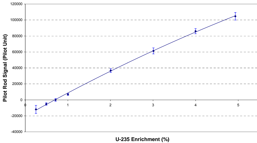
Figure 21: Calibration curve of the ^{235}\text{U} calibration samples for the R1-MOX configuration
