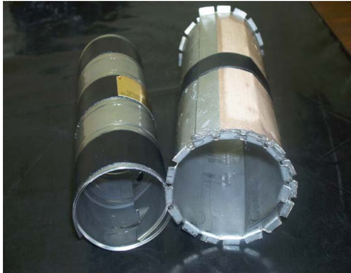
Figure 5. Coiled Diameter Comparison for 28 and 24 Gage
