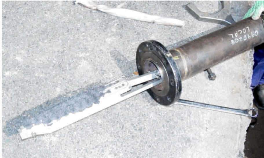
Figure 41. Magnet Assembly for Removing Filings
