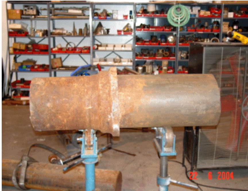
Figure 9. 12-Inch Cast Iron Pipe Sample
