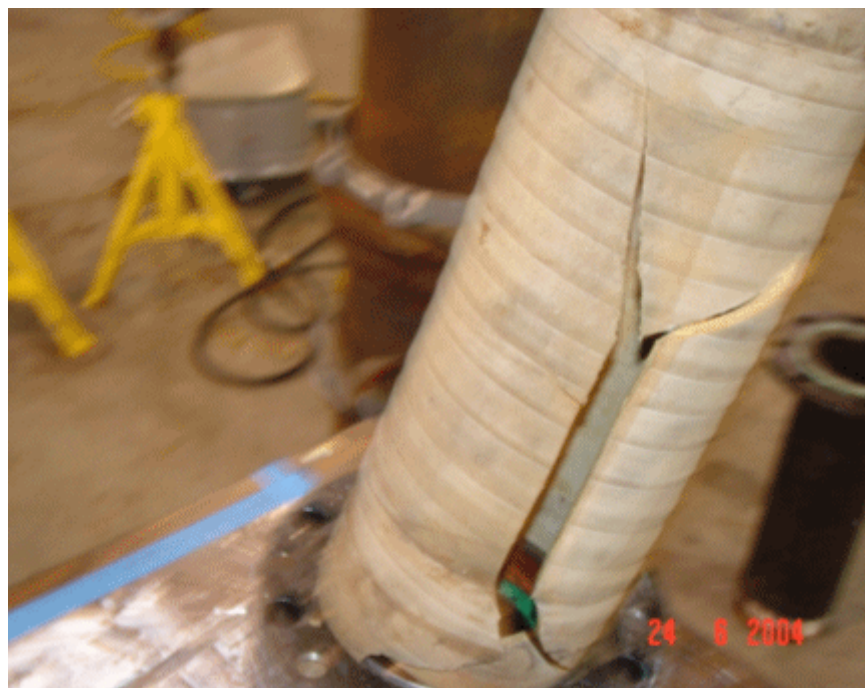
Figure 13. Ruptured Inflation Bladder
