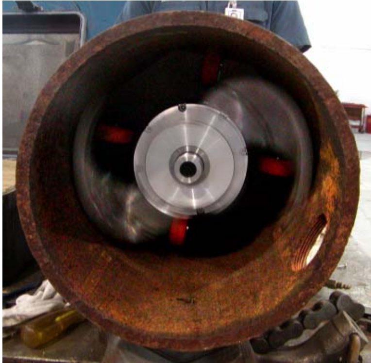
Figure 26. Pipe Wall Cleaning Test
