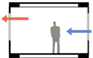
Cross ventilation: D \leq 5H When the room has windows on opposite sides, cross ventilation is effective up to 40 ft of the room depth or five times the room height.
