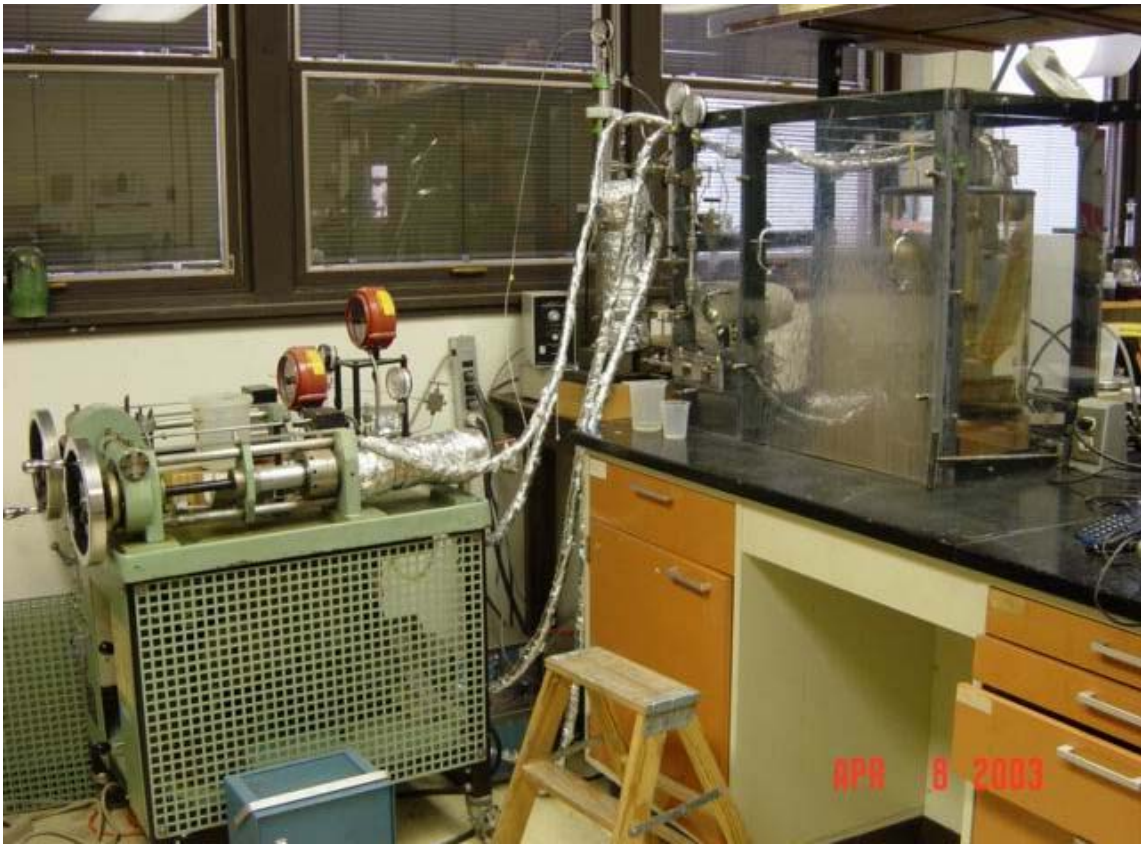
Fig. 1-2. Foam stability apparatus set-up.
