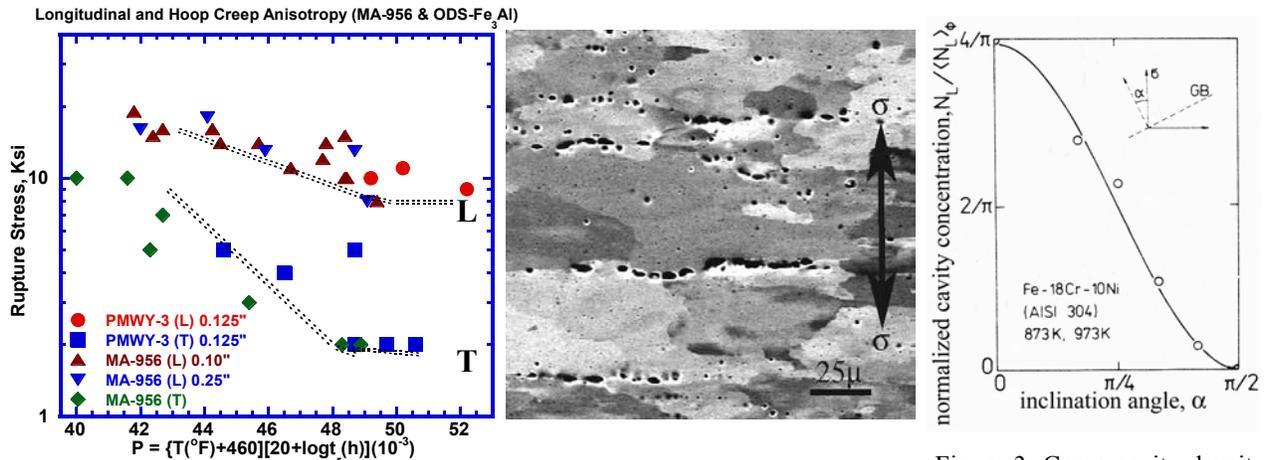
Figure 2. Longitudinal (L) vs. transverse (T) creep anisotropy in Fe<sub>3</sub>Al (PMWY3) and MA-956 tubes. **b)** Creep cavitation observations in hoop creep loading tests.
