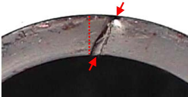
Figure 5. Cross rolling of MA956 tube via repeated passes at 900°C. The red line indicates the notch as inscribed on the tube wall prior to testing. The angle between the red line and the sheared image (denoted by red arrows) gives the shear strain incurred via rotary cross-rolling process.
