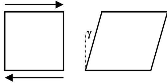
Figure 6. Schematic illustration of deformation shear strain as introduced via rotary deformation.
