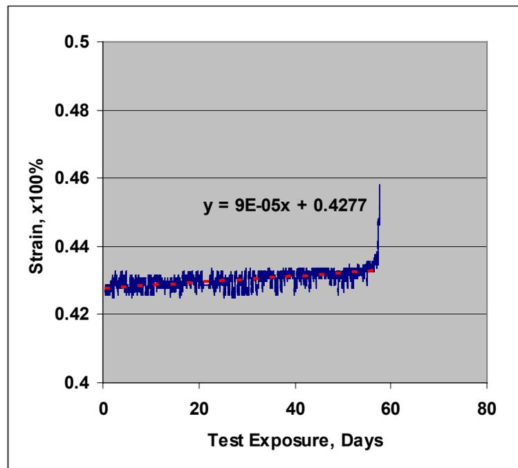
Figure 8. Creep test of a MA956 sample extracted from a 2 1/2" OD, 1/4" wall thickness tube and cross-rolled at 900°C to 20% reduction. Creep test conducted at 900°C at 2Ksi stress in air.
