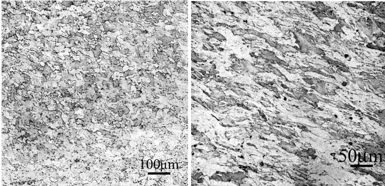
Figure 7. Cross-sectional view of the a) as-received, recrystallized and b) cross-rolled and recrystallized MA956 tube. The grain shape is significantly modified, with the grain long axis now stretched along the hoop direction.
