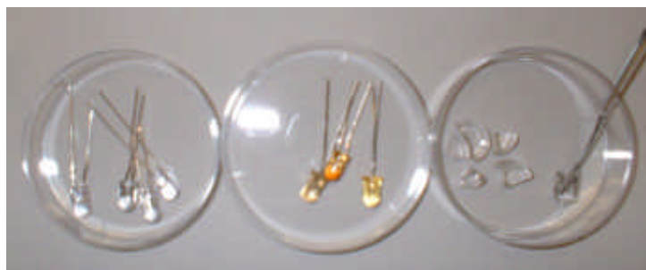
Fig. 76. Comparison of VPC 2000 with conventional 5 mm LED epoxy. Left: unheated conventional epoxy; center: conventional epoxy heated at 140°C for 14 days; right: VPC 2000 heated at 140°C for 3 months.
