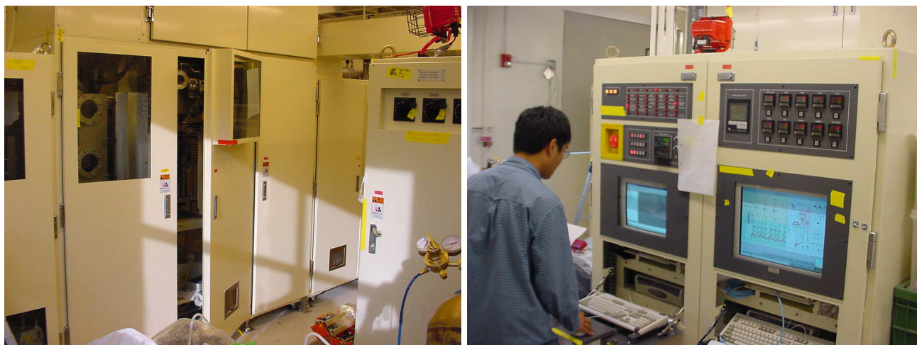
Fig. 2. Front view of Nippon Sanso MOCVD system (left) and Control Panel (right).
