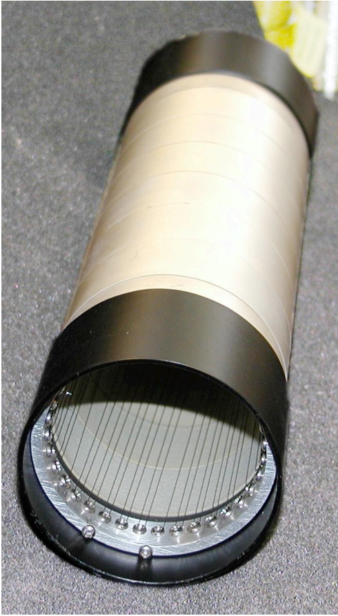
Fig. 2: Photograph of the 20 cm ferroelectric plasma source showing the aluminium mounting rings and the stainless steel electrode wires.
