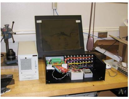
Figure 3-2. Rear View of Field Data Acquisition System (DAS)
