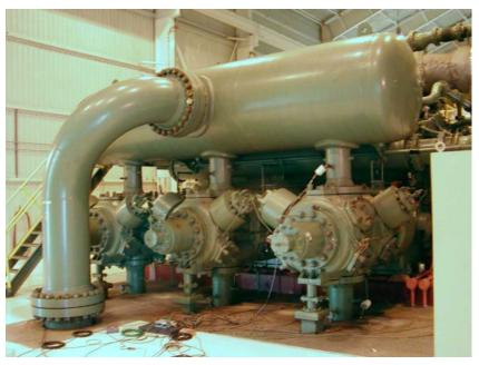
Figure 4-2. Heated Pressure Sensors Temporarily Installed on Cylinder 1; Dresser-Rand TCVC10; Dominion Groveport Station Unit 1; April 20, 2005
