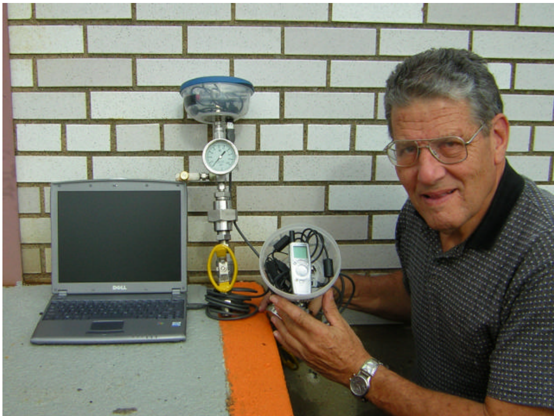
Figure 15: On the left is a complete Pipeline Acoustic Monitoring Package (PAMP) shown with a laptop for data analysis. The PAMP (on right) shows that unit can also be operated without a laptop, using its internal data recorder. The internal microphone is pressure equalized up to 1000 psi.
