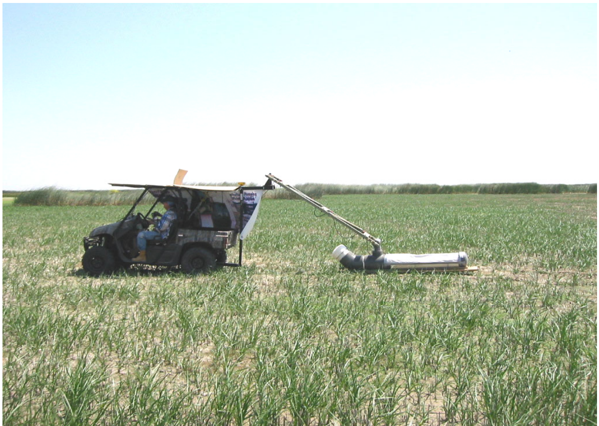
Figure 5.3 EM-38 dual mode meter (Geonics Ltd) placed in a carrier-sled that was attached at the rear of an ATV. Horizontal and vertical aligned coupled meters provide sensing of near-surface bulk salinity (top 6 inches) and deeper bulk salinity (up to 6 feet).
