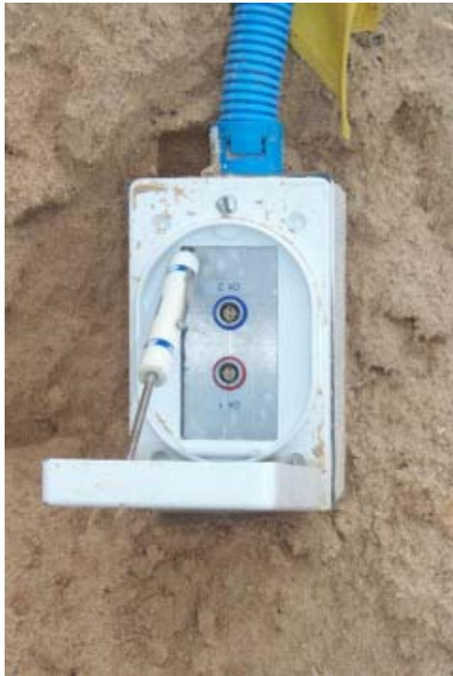
**Figure 4. Photograph of the junction box showing the connectors that are connected to the MsS instrument for collecting MsS data**
