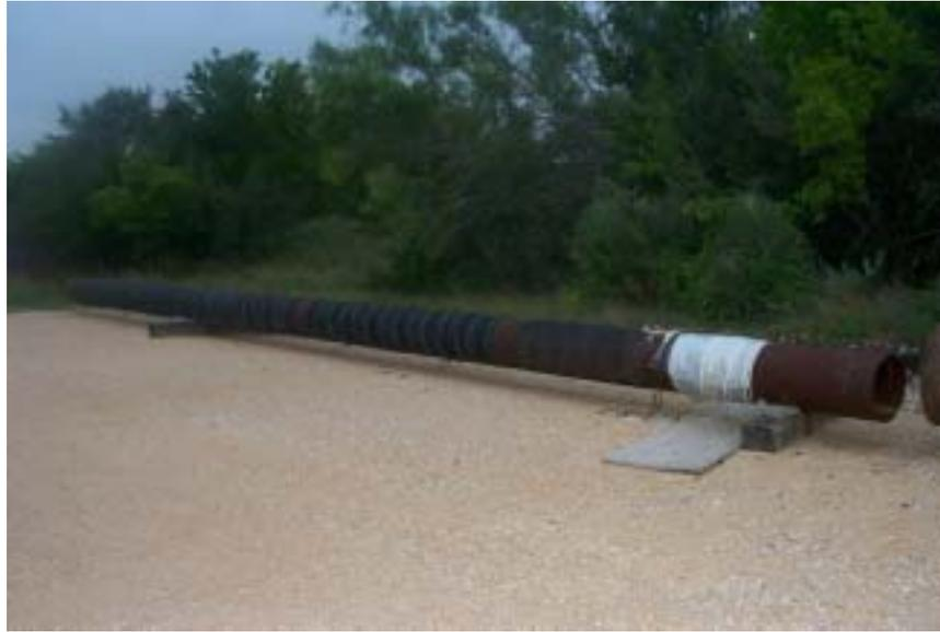
**Figure 14. Photograph of the bitumen coated, 16-inch-diameter pipe**
