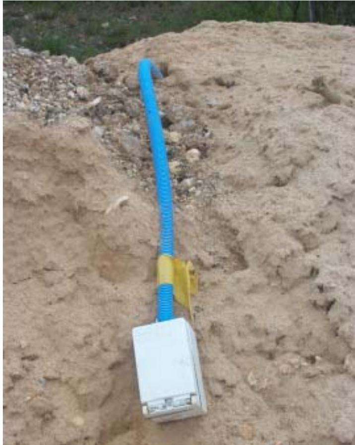
Figure 18. Photograph of one of the locations of an MsS bonded to the buried 610-mm (24-inch)-diameter pipe
