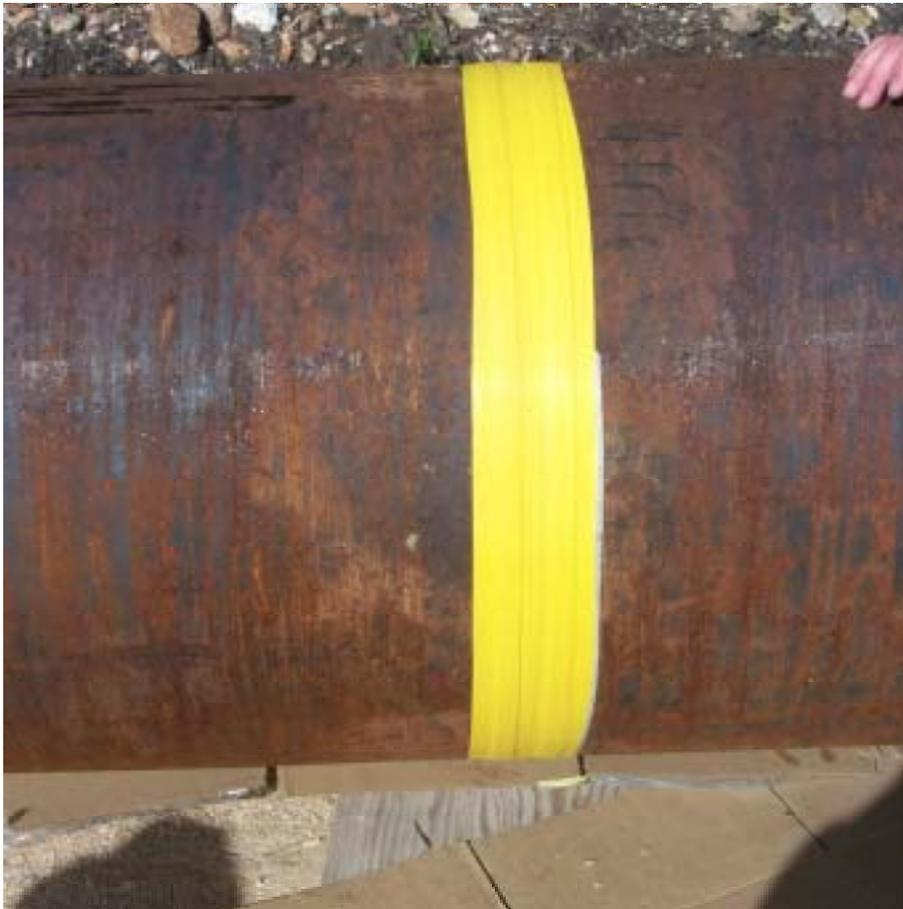
**Figure 3. Protective tape coating over nickel strip and electrical coil**
