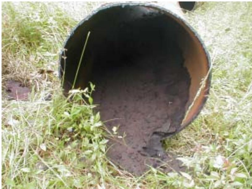
**Figure 31. Inside surface of pipeline showing major internal corrosion**
