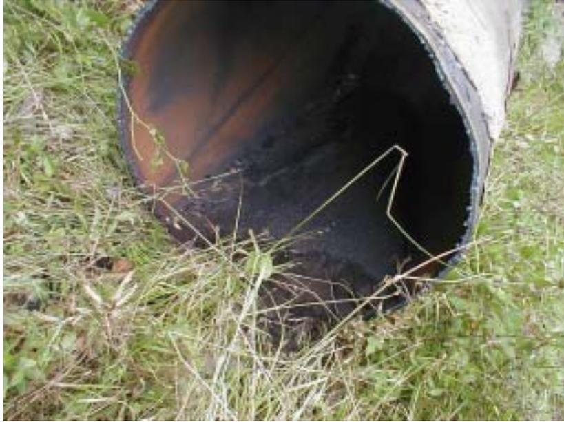
**Figure 32. Another view of the inside surface of the pipeline showing major internal corrosion**
