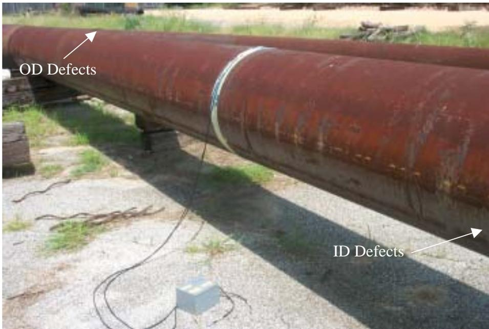
**Figure 5. Photograph of the 610-mm (24-inch)-diameter pipe showing the location of the MsS and the OD and ID defects along the pipe axis**
