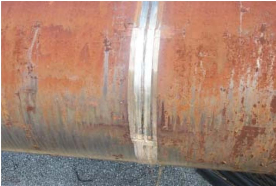
**Figure 3. Photograph showing nickel strip bonded to the 610-mm (24-inch)-diameter pipe. The two strips are used to provide directionality in the transmitted signal.**
