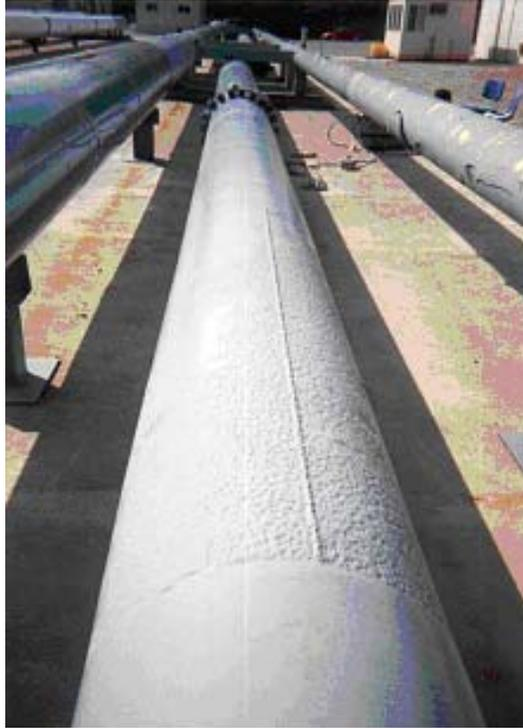
**Figure 29. Photograph showing MsS probe installed on pipe having a heavily corroded section**
