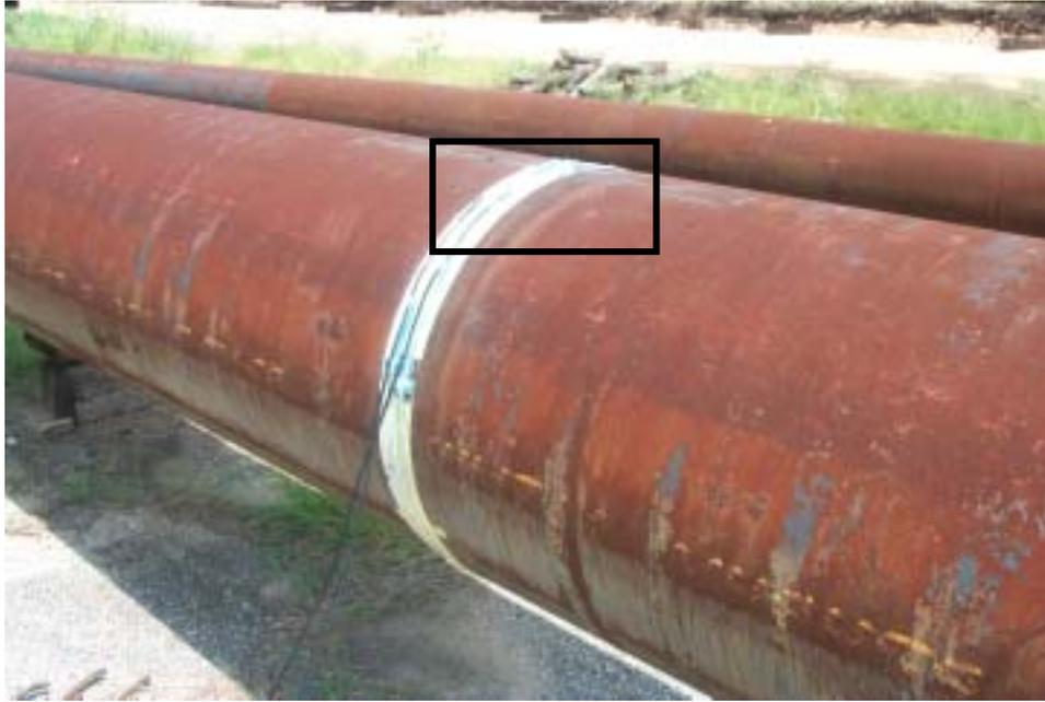
**Figure 4. Photograph of the nickel strip and coil bonded to the test pipe showing the low height profile of the MsS**
