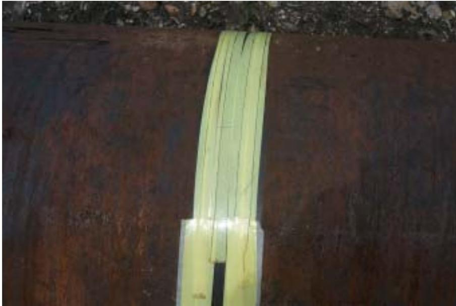
**Figure 1. Photograph showing tape wrapped around the two-nickel strips with their outline marked with a pen**
