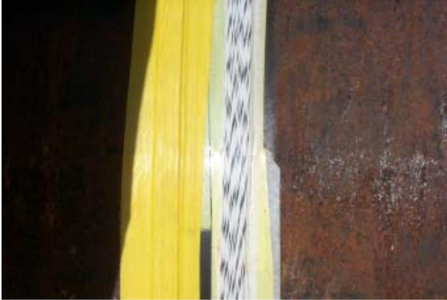
**Figure 2. Photograph of the coils wound on the pipe showing yellow vinyl duct tape used to cover the windings of one coil while the second coil is held down with double-sided tape**
