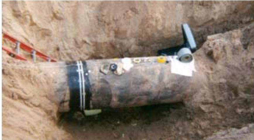
**Figure 35. MsS installed on the 762-mm (30-inch)-OD gas transmission pipeline**
