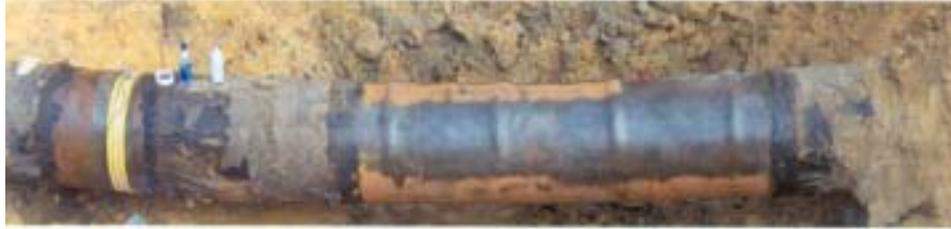
**Figure 26. Photograph of the pipe excavated at the Cleveland site showing the location of the MsS coil and bend rings**
