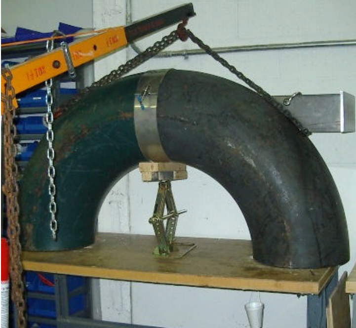
Figure 3. Friction coefficient test setup
