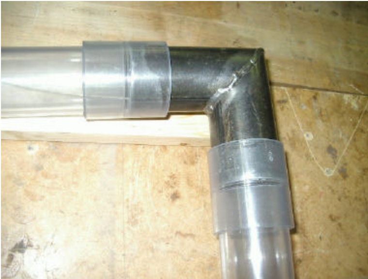
Figure 4. Tether abrasion test in mitered corner
