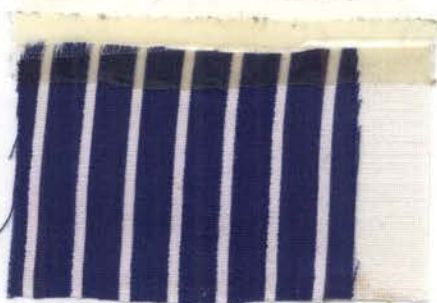
Fig. 73.--Sample 9 (labeled "Fast to Washing") before washing.
