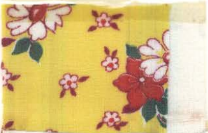
Fig. 90.--Sample 11 after first washing with detergent B.
