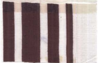
Fig. 124.--Sample 15 after twentieth washing with detergent B.
