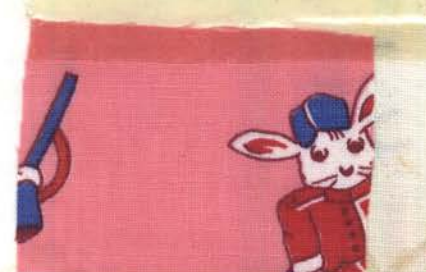
Fig. 54.--Sample 8 after first washing with detergent A.
