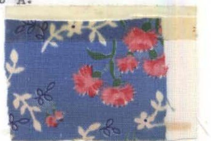
Fig. 103.--Sample 14 after tenth washing with detergent A.
