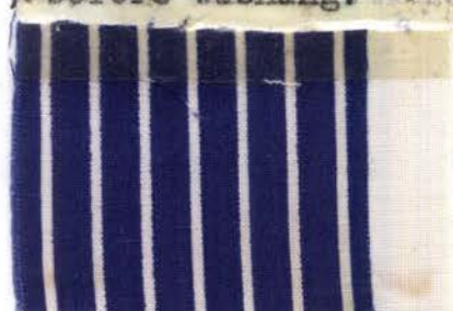
Fig. 78.--Sample 10 after first washing with detergent B.
