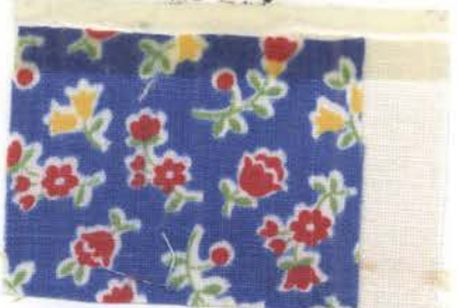
Fig. 98.--Sample 13 after first washing with detergent A.
