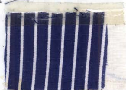
Fig. 67.--Sample 9 after tenth washing with detergent A.
