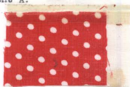
Fig. 24.--Sample 4 after twentieth washing with detergent A.
