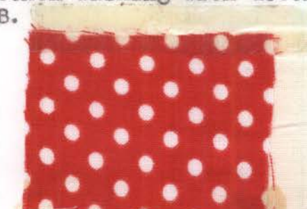
Fig. 28.--Sample 3 after twentieth washing with detergent B.
