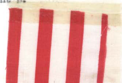
Fig. 47.--Sample 6 after tenth washing with detergent B.
