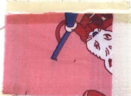
Fig. 61.--Sample 8 (labeled "Guaranteed Fast Color") before washing.
