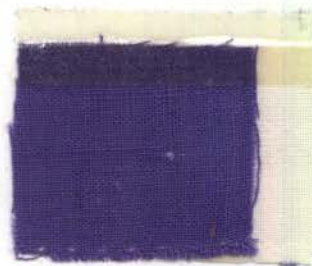
Standard samples after tenth washing with detergent A.
