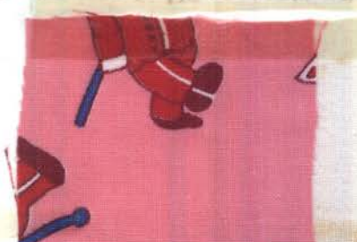
Fig. 63.--Sample 8 after tenth washing with detergent B.
