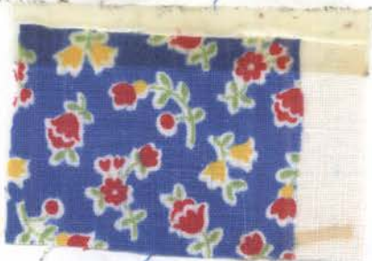
Fig. 99.--Sample 13 after tenth washing with detergent A.
