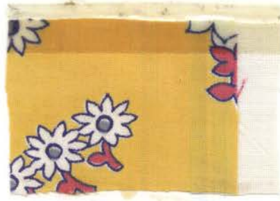
Fig. 85.--Sample 12 (labeled "Guaranteed Fast Color") before washing.
