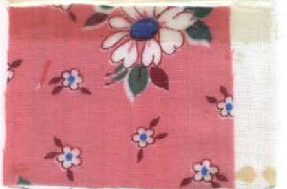
Fig. 51.--Sample 7 after tenth washing with detergent A.
