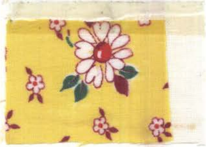
Fig. 84.--Sample 11 after twentieth washing with detergent A.
