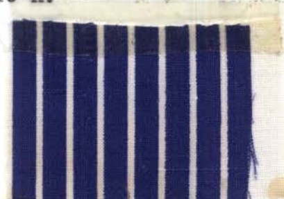
Fig. 72.--Sample 10 after twentieth washing with detergent A.
