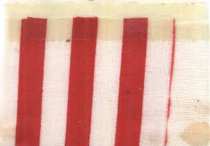
Fig. 34.--Sample 5 after first washing with detergent A.
