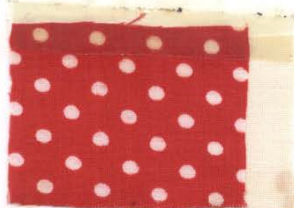
Fig. 29.--Sample 4 (labeled "Guaranteed Fast Color") before washing.
