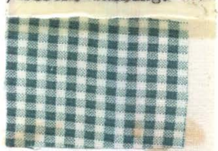
Fig. 14.--Sample 2 after first washing with detergent B.
