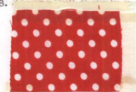
Fig. 27.--Sample 3 after tenth washing with detergent B.
