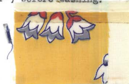
Fig. 86.--Sample 12 after first washing with detergent A.
