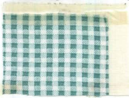
Fig. 12.--Sample 1 after twentieth washing with detergent B.
