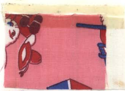
Fig. 53.--Sample 8 (labeled "Guaranteed Fast Color") before washing.
