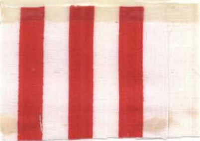
Fig. 44.--Sample 5 after twentieth washing with detergent B.
