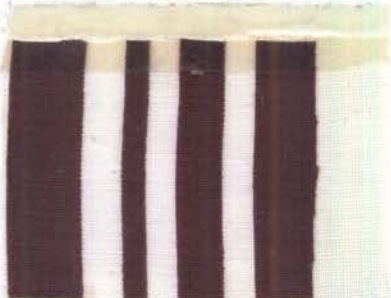
Fig. 116.--Sample 15 after twentieth washing with detergent A.
