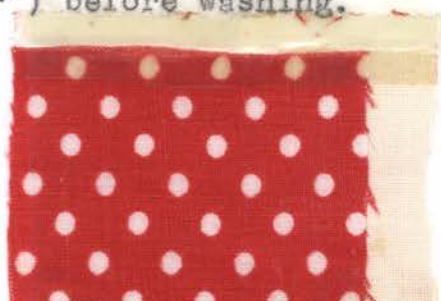
Fig. 30.--Sample 4 after first washing with detergent B.
