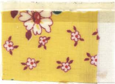
Fig. 81.--Sample 11 (labeled "Fast to Washing") before washing.
