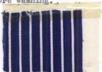
Fig. 74.--Sample 9 after first washing with detergent B.
