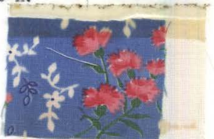
Fig. 104.--Sample 14 after twentieth washing with detergent A.
