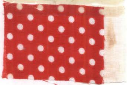
Fig. 19.--Sample 3 after tenth washing with detergent A.
