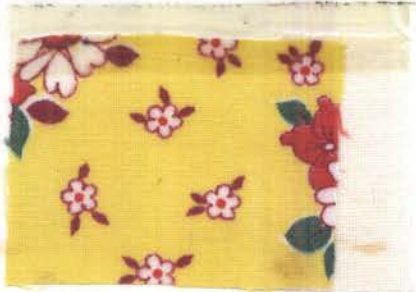
Fig. 83.--Sample 11 after tenth washing with detergent A.
