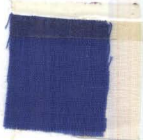
Standard samples after tenth washing with detergent B.
