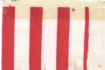
Fig. 39.--Sample 6 after tenth washing with detergent A.
