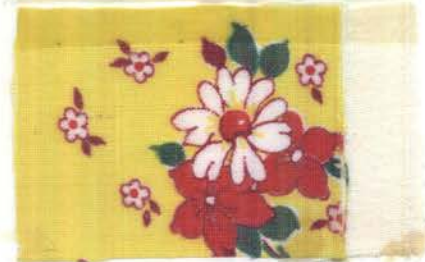
Fig. 92.--Sample 11 after twentieth washing with detergent B.
