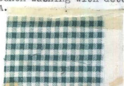
Fig. 8.--Sample 2 after twentieth washing with detergent A.
