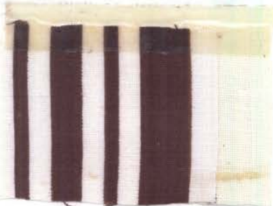
Fig. 115.--Sample 15 after tenth washing with detergent A.
