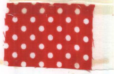
Fig. 20.--Sample 3 after twentieth washing with detergent A.
