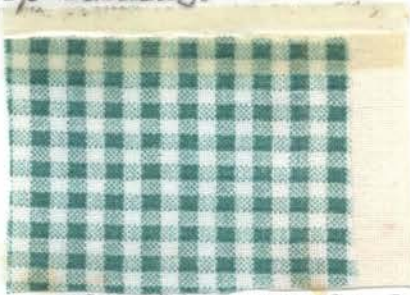
Fig. 10.--Sample 1 after first washing with detergent B.
