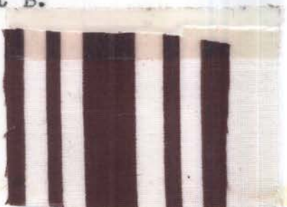
Fig. 123.--Sample 15 after tenth washing with detergent B.
