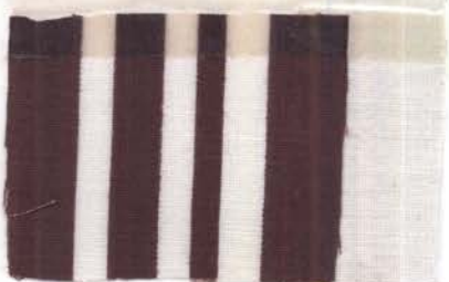
Fig. 122.--Sample 15 after first washing with detergent B.
