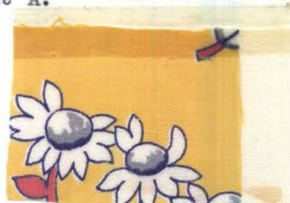
Fig. 87.--Sample 12 after tenth washing with detergent A.
