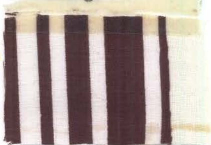
Fig. 114.--Sample 15 after first washing with detergent A.
