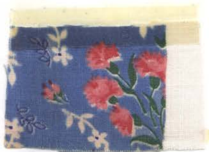
Fig. 109.--Sample 14 (labeled "Guaranteed Fast Color") before washing.
