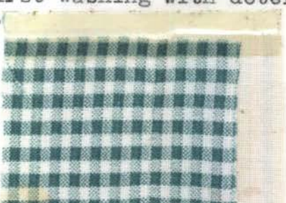
Fig. 7.--Sample 2 after tenth washing with detergent A.
