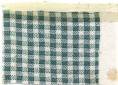
Fig. 5.--Sample 2 (labeled "Guaranteed Fast Color") before washing.
