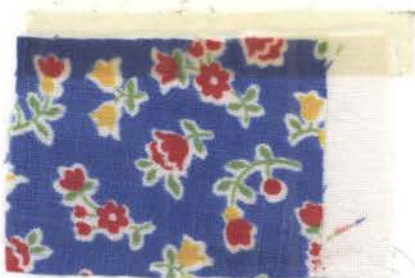
Fig. 105.--Sample 13 (labeled "Fast to Washing") before washing.
