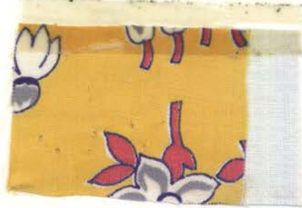
Fig. 93.--Sample 12 (labeled "Guaranteed Fast Color") before washing.
