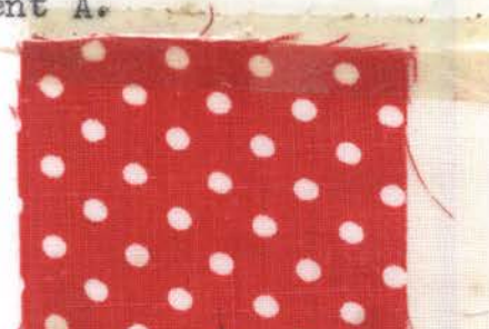
Fig. 23.--Sample 4 after tenth washing with detergent A.
