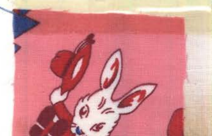
Fig. 55.--Sample 8 after tenth washing with detergent A.
