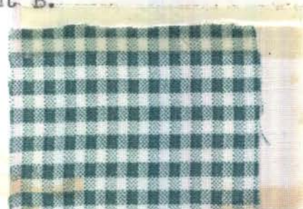
Fig. 15.--Sample 2 after tenth washing with detergent B.
