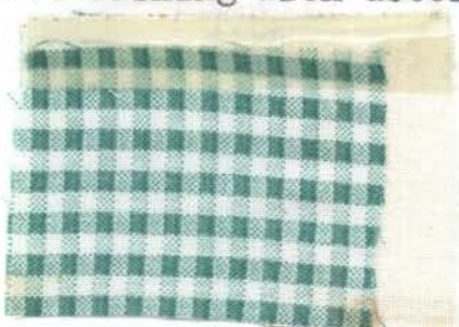
Fig. 3.--Sample 1 after tenth washing with detergent A.
