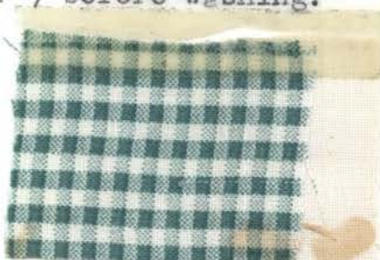
Fig. 6.--Sample 2 after first washing with detergent A.
