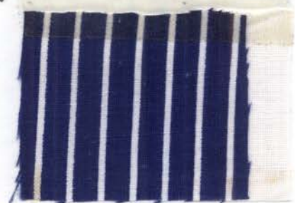
Fig. 68.--Sample 9 after twentieth washing with detergent A.
