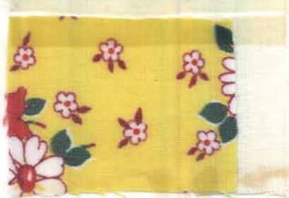
Fig. 91.--Sample 11 after tenth washing with detergent B.
