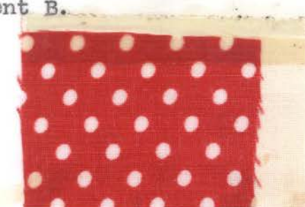
Fig. 31.--Sample 4 after tenth washing with detergent B.
