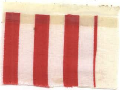
Fig. 41.--Sample 5 (labeled "Fast to Washing") before washing.
