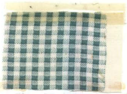
Fig. 13.--Sample 2 (labeled "Guaranteed Fast Color") before washing.
