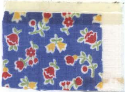
Fig. 107.--Sample 13 after tenth washing with detergent B.
