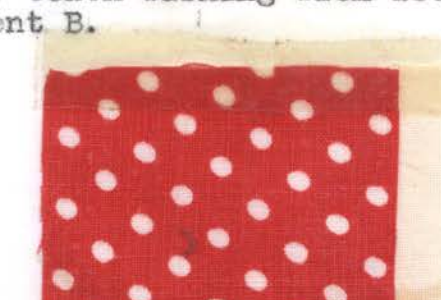
Fig. 32.--Sample 4 after twentieth washing with detergent B.
