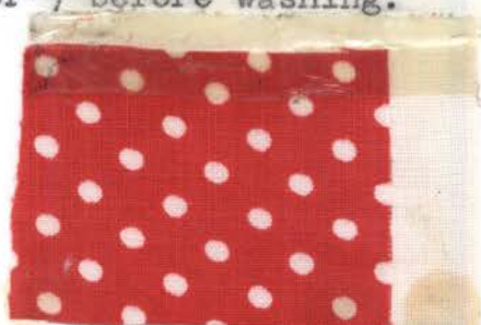
Fig. 22.--Sample 4 after first washing with detergent A.
