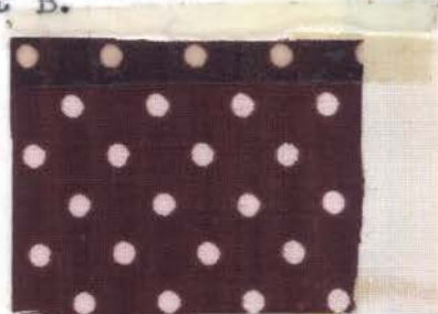
Fig. 127.--Sample 16 after tenth washing with detergent B.
