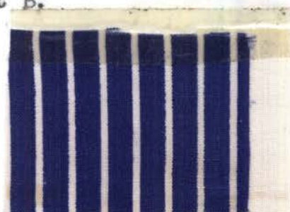
Fig. 79.--Sample 10 after tenth washing with detergent B.
