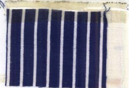
Fig. 75.--Sample 9 after tenth washing with detergent B.
