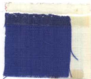
Standard samples after tenth washing with detergent A.
