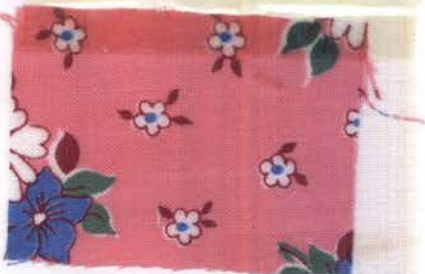
Fig. 59.--Sample 7 after tenth washing with detergent B.
