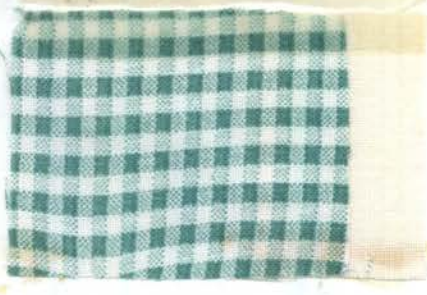
Fig. 11.--Sample 1 after tenth washing with detergent B.
