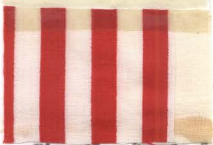
Fig. 42.--Sample 5 after first washing with detergent B.
