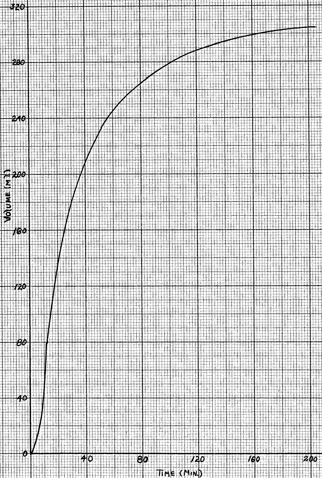
Fig. 12.--Rates of Reaction with a 5:1 Mixture of 2, 2, 4-Trimethylpentane and Normal Octane.
