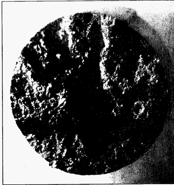
Figure 26. Stereo Picture of Fracture Surface after Uniaxial Tensile Testing of Aluminum 319 Alloy
