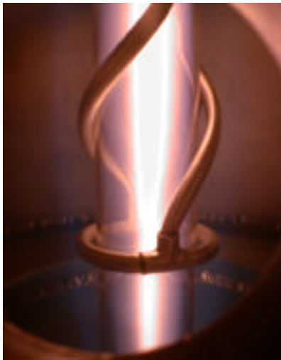
Figure 4. Steady-state helicon discharge in helium on the ASPL experiment.
