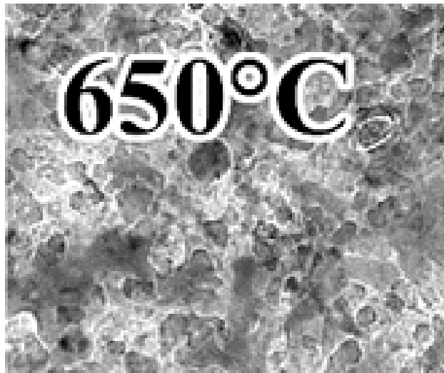
Figure 38 (continued). Microstructure as a Function of Annealing Temperature in the 316 SS Hex Duct irradiated to 30 dpa. Diffraction pattern illustrates oxide formation at 650°C.
