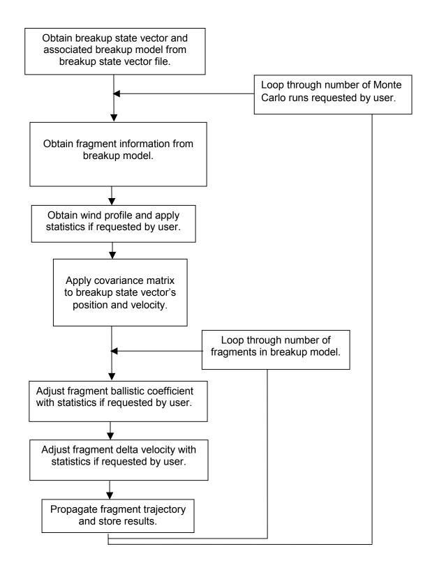
Figure 2-1. Internal Procedure to Initialize and Propagate Breakup Fragments
