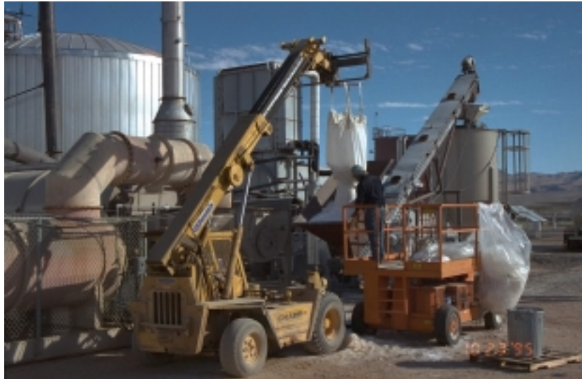
Figure L-3. The salt handling system crushed the salt and transported it to the melter.
