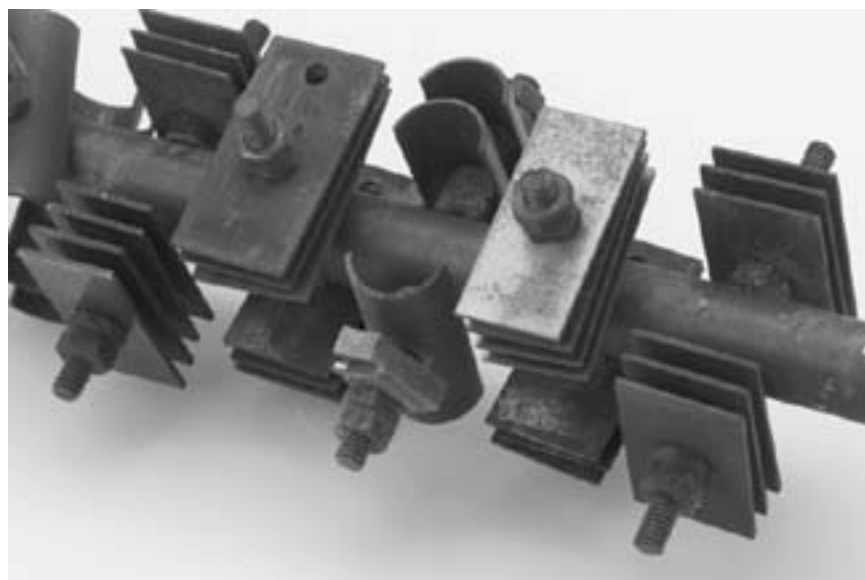
Figure H-4. Typical specimen mounting arrangement from the chamber Y-251 specimen tree. Flat coupons include 304SS and 316SS. Curved coupons are pieces of 316SS Solar Two receiver tubing.
