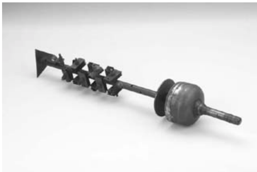
Figure H-3. Specimen mounting tree after removal from Chamber Y-251, with branches and specimens for first sampling interval already removed from the end of the tree nearest end cap.
