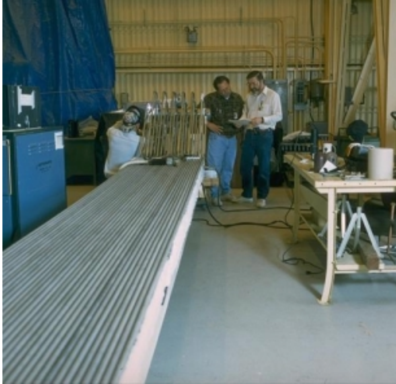
Figure H-11. Single panel from Solar Two receiver. Individual tubes can be seen in the foreground and the headers are in the background. This is before installation vertically into the receiver.
