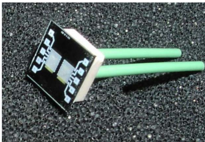
Figure 33. Dual membrane chemical sensor chip mounted to a plastic (PEEK) header.
