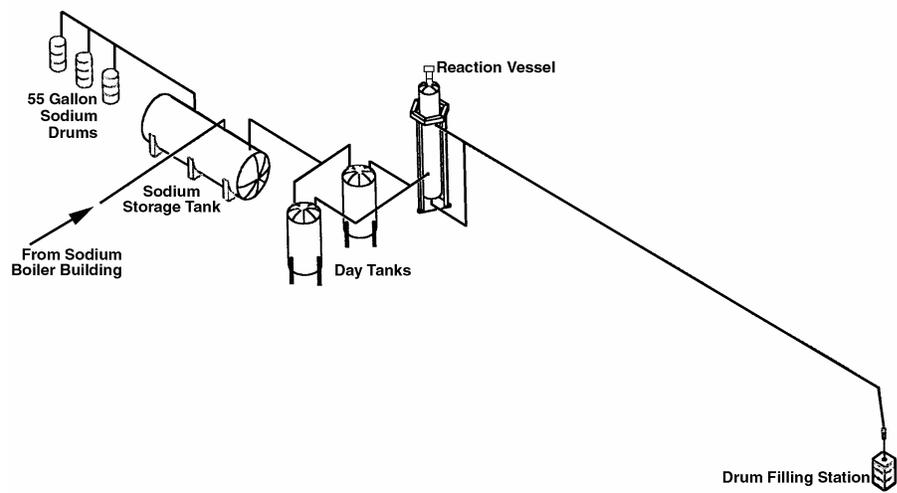
Fig. 3. Sodium Process Facility Flow Diagram
